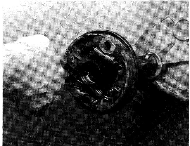
4. Remove inner snap ring. Use caution as not to damage bearing surfaces.
