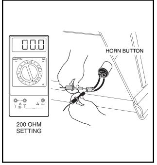
Figure 11-56 Horn Circuit Test
