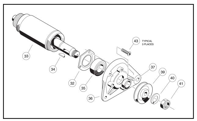
Figure 12-7 Armature and Output End Cover Assembly
