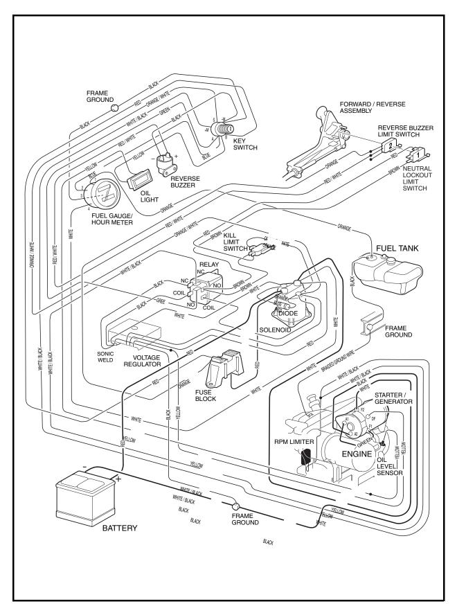
Figure 11-7 Wiring Diagram for Carryall 2 Plus Vehicle
