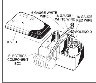
Figure 11-15 Key Switch Test – Accessory Terminal
