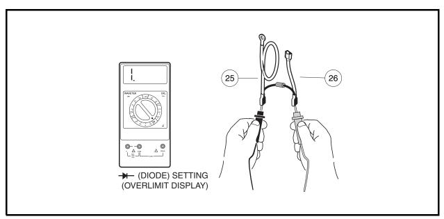
Figure 11-49 Voltage Suppressor Test
