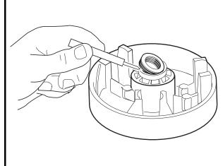
Figure 17-12 Remove Idler Bearing
