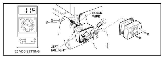
Figure 11-52 Taillight Socket Voltage Test
