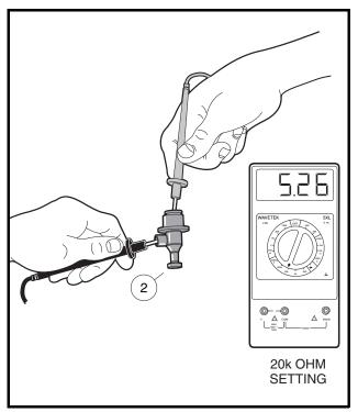
Figure 11-30 Spark Plug Cap Test
