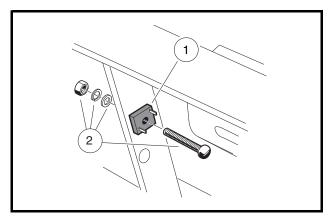
Figure 12-35 Voltage Limiter
