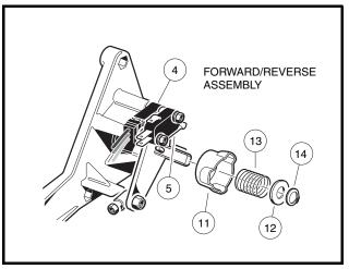
Figure 12-20 Neutral Lockout Cam
