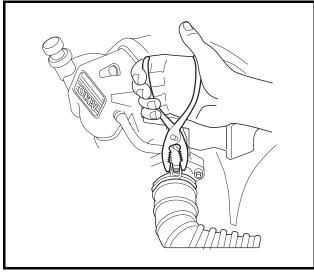
Figure 16-9 Fuel Vent Tube
