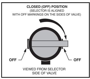
Figure 14-16 Closed Fuel Shut-off Valve
