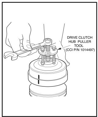
Figure 17-6 Mark Drive Clutch Hub
