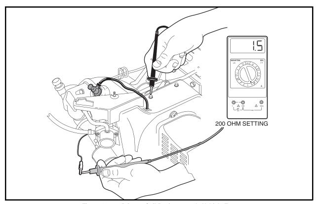
Figure 11-26 Primary Coil Resistance – In Vehicle Test
