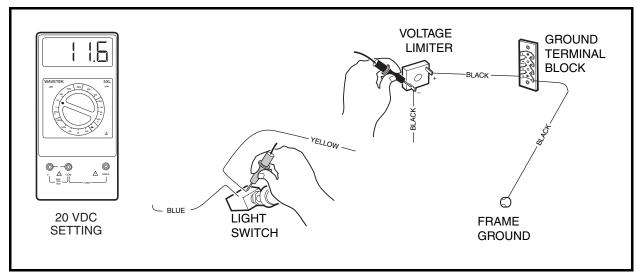
Figure 11-51 Voltage Limiter Circuit Test
