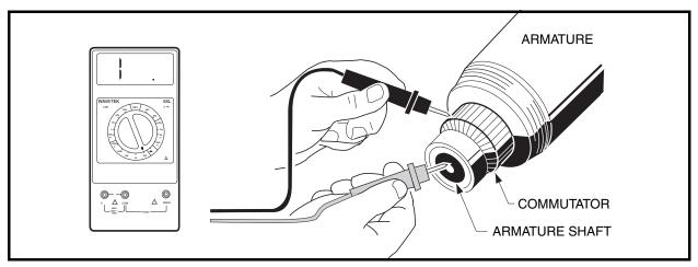
Figure 12-12 Armature Ground Test
