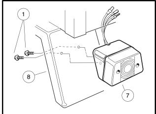
Figure 12-34 Mount Taillight To Rear Fender
