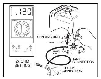
Figure 11-39 Fuel Level Sending Unit Test
