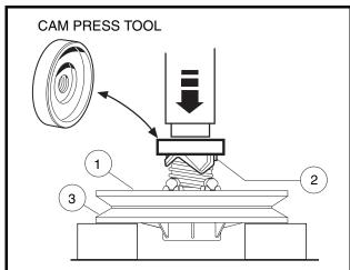
Figure 17-19 Cam Press Tool
