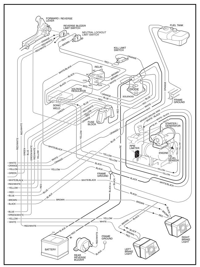
Figure 11-4 Wiring Diagram for Carryall 6, Villager, and TransPorter Vehicles (Rear)
