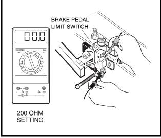
Figure 11-54 Check Park Brake Limit Switch Circuit
