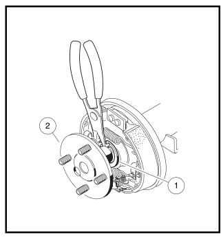
Figure 16-3 Retaining Ring
