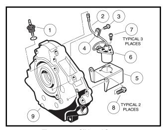
Figure 13-5 Oil Level Sensor
