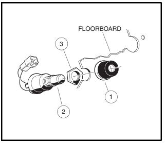
Figure 12-42 Horn Assembly
