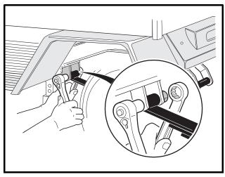
Figure 16-23 Spring Retainer Bolts
