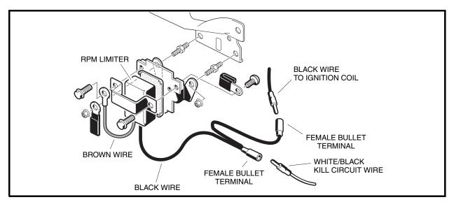
Figure 11-25 RPM Limiter
