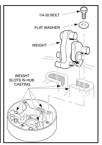
Figure 17-8 Drive Button Mounting
