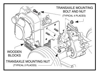
Figure 16-34 Transaxle Mounting
