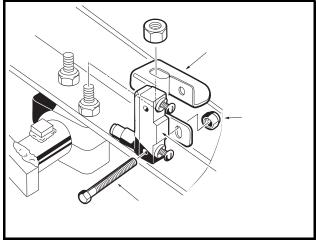
Figure 12-41 Mount Brake Pedal Limit Switch to Brake Pedal Mounting Bracket
