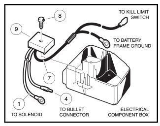
Figure 12-15 Voltage Regulator for Pedal-Start Vehicles
