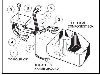
Figure 12-16 Voltage Regulator for Key-Start Vehicles
