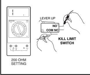
Figure 11-35 Kill Limit Switch for Pedal-Start Vehicle
