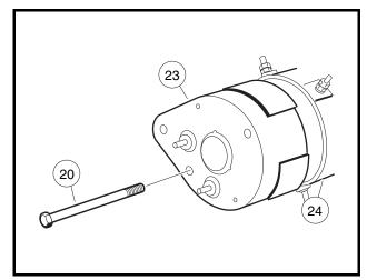
Figure 12-2 Commutator End Cover
