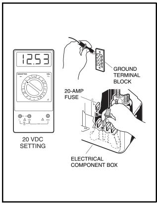
Figure 11-44 Starter/Generator and Neutral Lockout Circuits Relay Test
