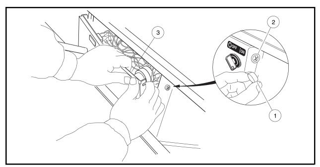
Figure 12-17 Center Dash Panel Removal
