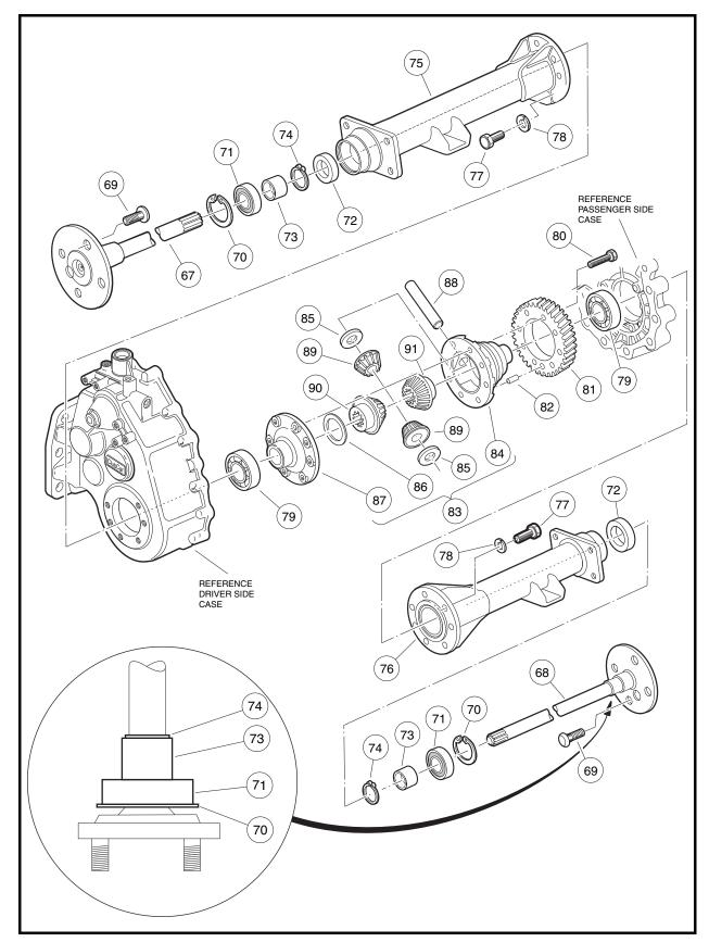
Figure 16-6 Differential Gear Case/Axle Tubes
