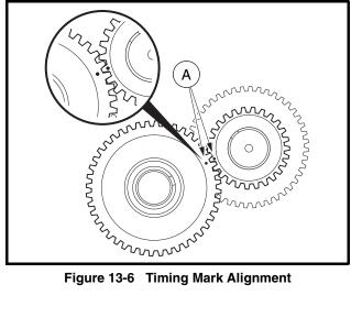
Figure 13-6 Timing Mark Alignment
