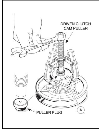
Figure 17-16 Remove Retaining Ring
