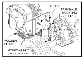
Figure 16-36 Transaxle Mounting
