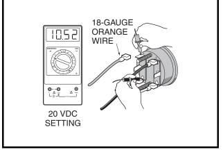
Figure 11-41 Fuel Gauge Voltage Test
