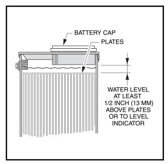
Figure 12-44 Battery Water Level
