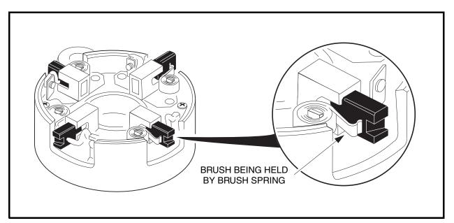
Figure 12-6 Pull Brushes Away from Center of the Commutator End Cover
