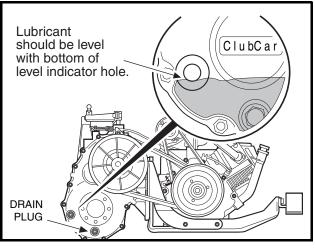
Figure 16-2 Lubricant Level
