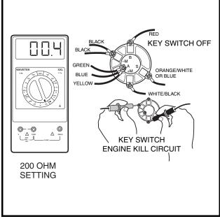
Figure 11-37 Key Switch Test – Engine Kill Circuit for Pedal-Start Vehicles
