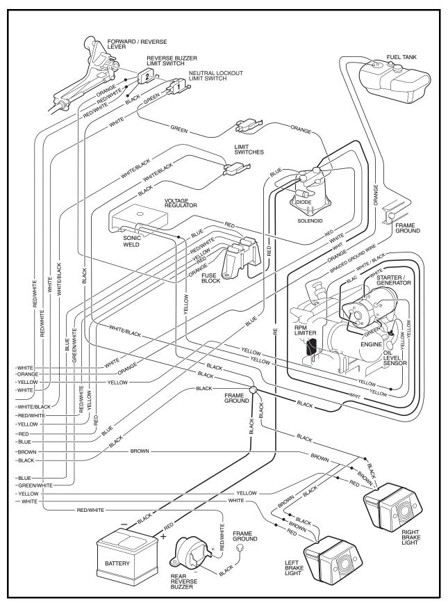
Figure 11-6 Wiring Diagram for Turf 6 Vehicle (Rear)
