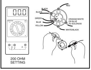
Figure 11-13 Key Switch Starter Circuit Test for Pedal-Start Vehicles
