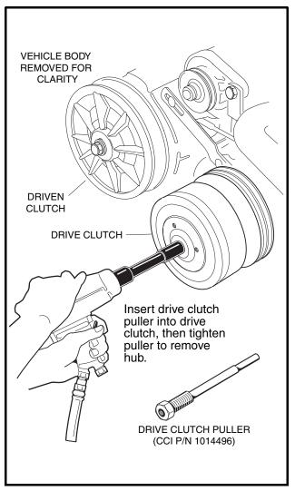
Figure 17-4 Drive Clutch Removal
