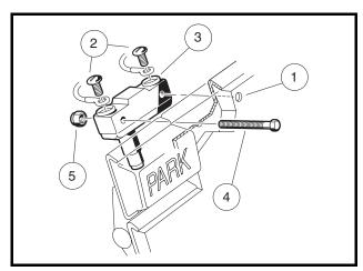
Figure 12-39 Park Brake Limit Switch
