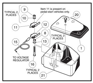
Figure 12-18 Accelerator Pedal and Kill Limit Switches
