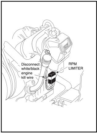
Figure 11-23 Ignition Spark Test
