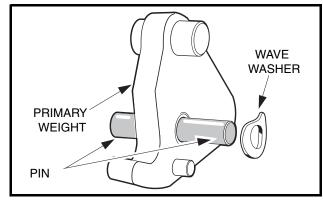
Figure 17-10 Install Pin and Washer
