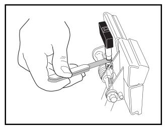
Figure 12-40 Mount Park Brake Limit Switch to Brake Pedal Using Feeler Gauge
