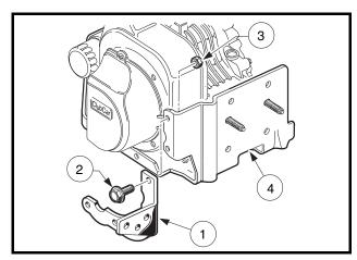
Figure 12-26 Stiffener Removal
