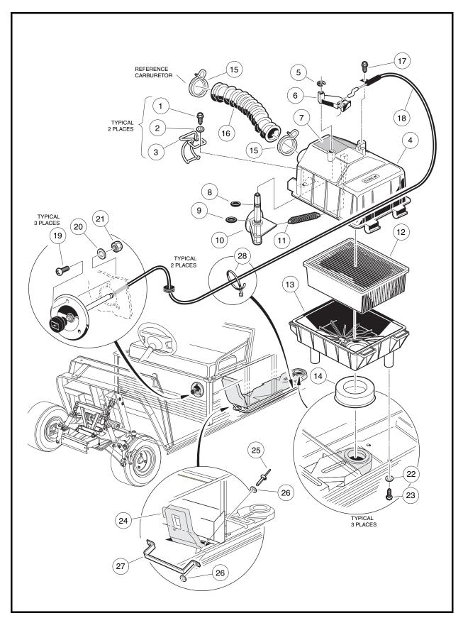
Figure 14-9 Turf 6, Carryall 6, TransPorter, and Villager Air Intake and Choke Assemblies
