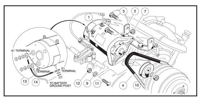
Figure 12-1 Starter/Generator Removal
