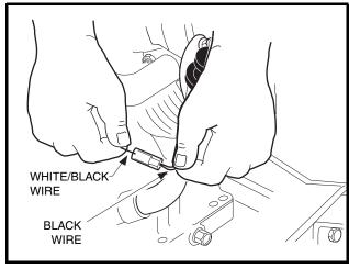
Figure 16-17 Oil Level Sensor Jumper Wire
