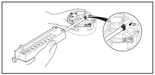
Figure 12-5 Brush Spring Tension Test
