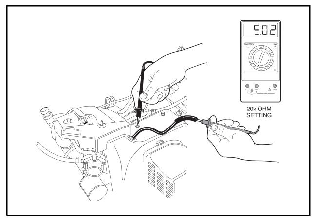
Figure 11-31 Secondary Coil Test Without Cap
