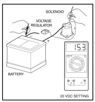
Figure 11-22 Voltage Regulator Test
