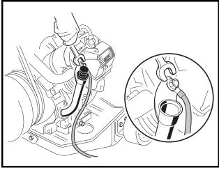
Figure 16-46 Connect Shifter Cable
