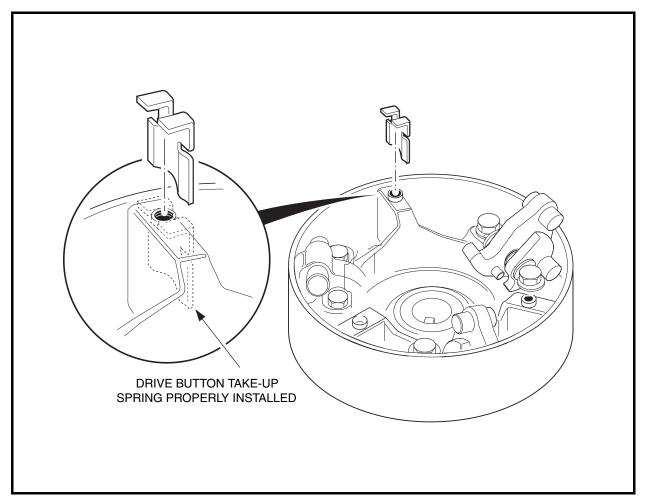
Figure 17-15 Correct Orientation of Drive Button Take-up Springs
