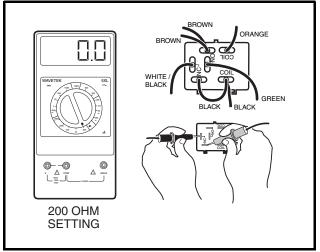
Figure 11-43 Engine Kill Circuit Relay Test
