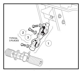
Figure 14-10 Compound Steering Joint
