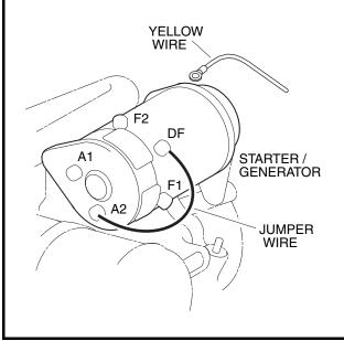
Figure 11-20 Check Starter Terminal Continuity
