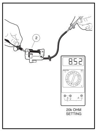
Figure 11-34 Secondary Coil Resistance - Bench Test
