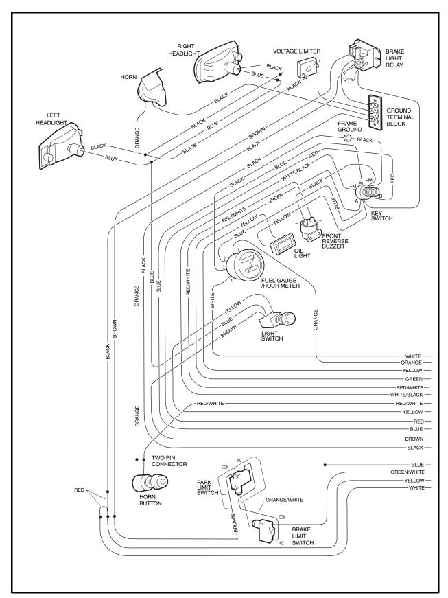
Figure 11-3 Wiring Diagram for Carryall 6, Villager, and TransPorter Vehicles (Front)
