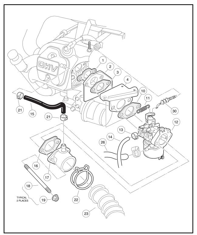
Figure 14-1 Carburetor Installation
