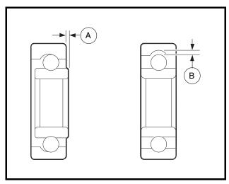
Figure 12-8 Bearing Play Inspection
