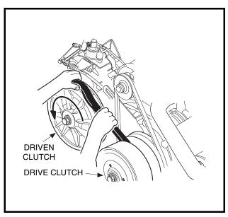
Figure 17-2 Drive Belt Removal
