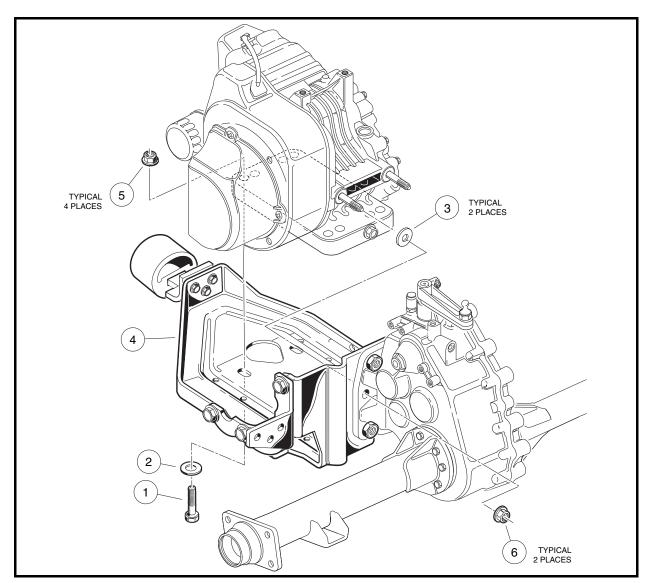
Figure 13-2 Engine Mounting Plate
