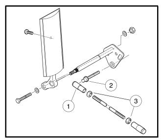
Figure 14-3 Accelerator Rod
