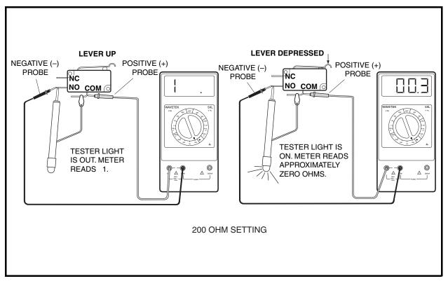
Figure 11-19 Neutral Lockout Limit Switch Test
