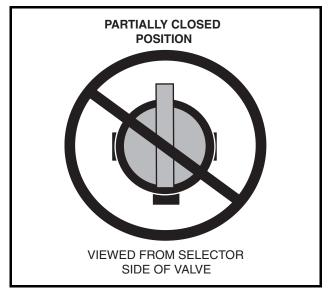
Figure 14-18 Incorrect Fuel Shut-off Valve
