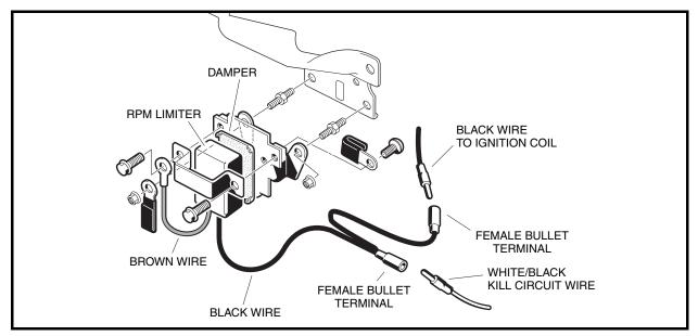
Figure 12-25 RPM Limiter
