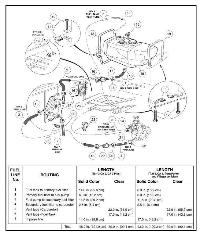
Figure 14-11 Fuel and Vent Lines
