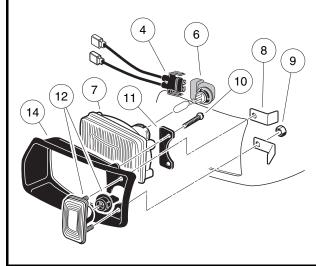
Figure 12-31 Relay Assembly – Key-Start Vehicles
