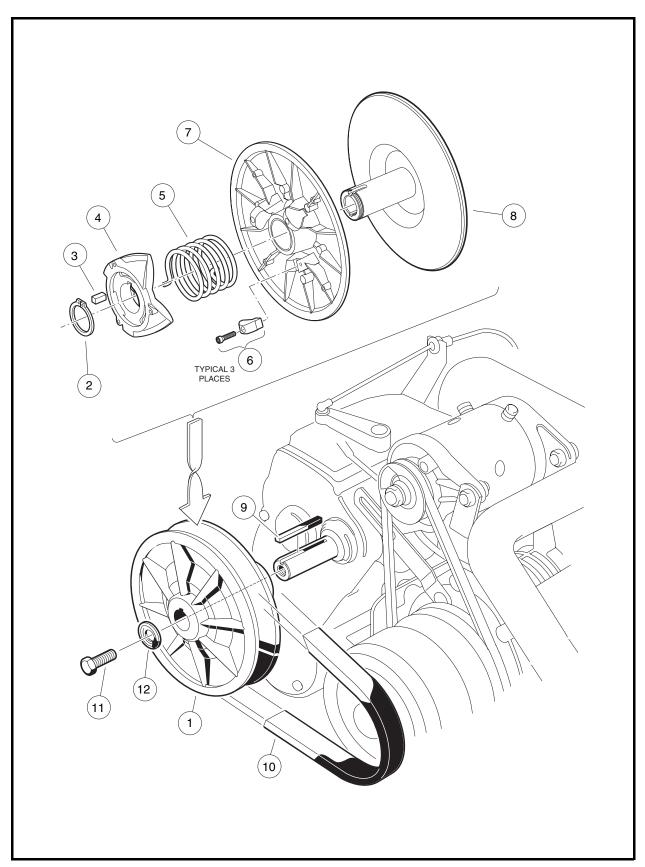
Figure 17-18 Driven Clutch Assembly
