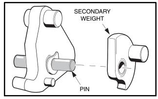
Figure 17-11 Install Secondary Weight
