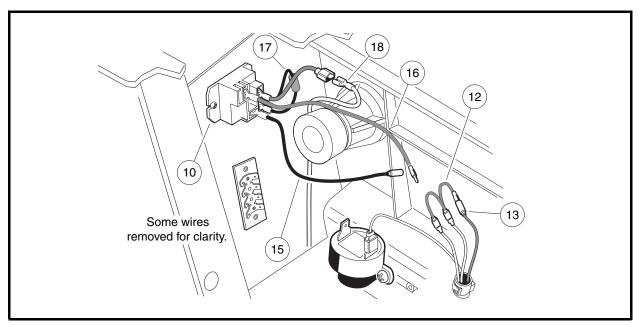
Figure 11-48 Bypassed Brake Light Relay
