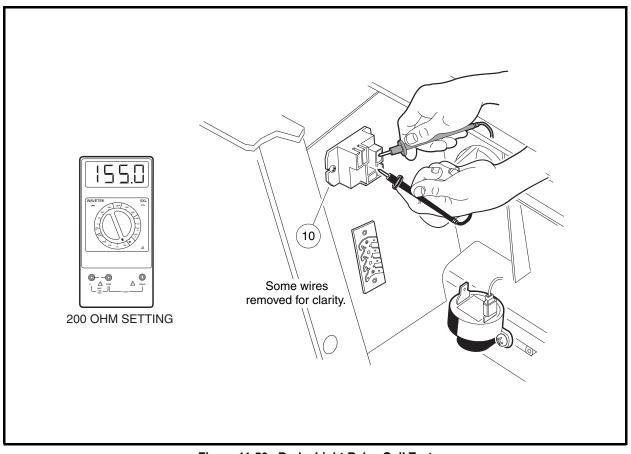
Figure 11-50 Brake Light Relay Coil Test
