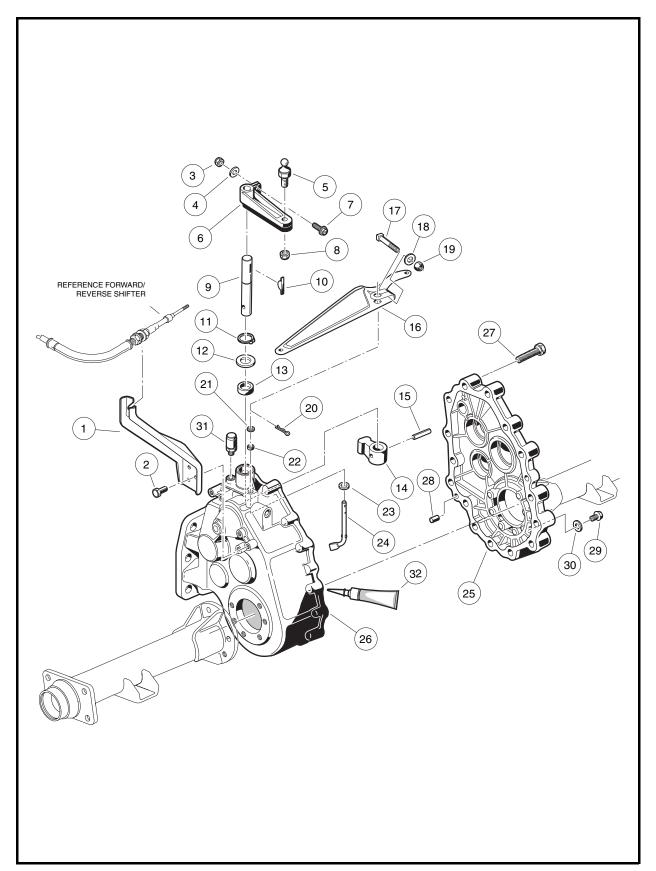
Figure 16-35 Transaxle Gear Casing and Brackets
