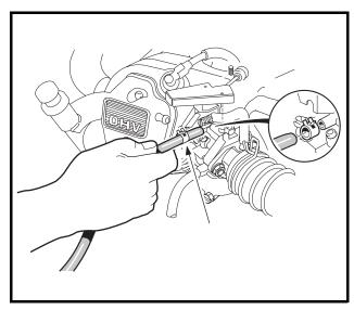
Figure 16-52 Carburetor Tube
