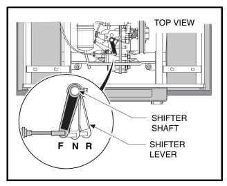
Figure 16-54 Forward/Reverse Shifter Positions
