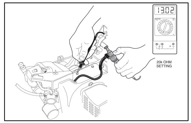
Figure 11-27 Secondary Coil Test – In Vehicle Test
