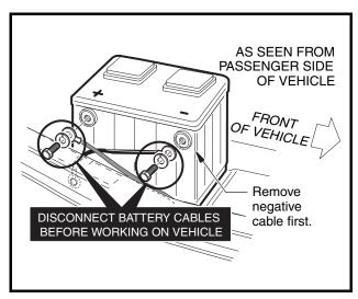
Figure 10-1 Battery Cable Removal
