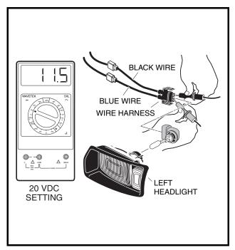
Figure 11-53 Headlight Socket Voltage Test
