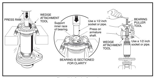
Figure 12-9 Bearing Removal
