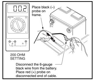
Figure 11-12 Battery Ground Cable Test
