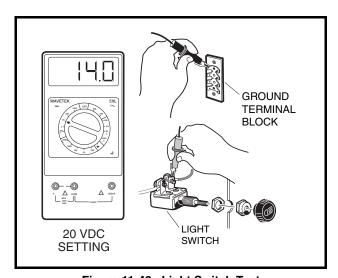
Figure 11-46 Light Switch Test
