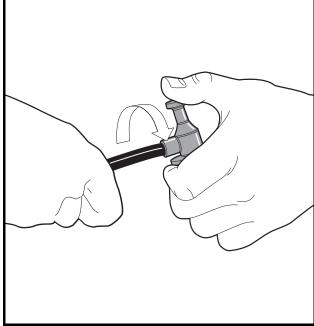
Figure 11-28 Ignition Coil and Cap
