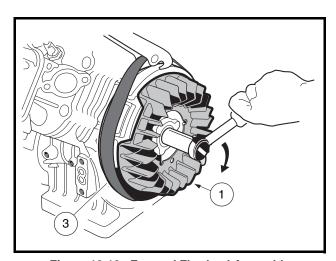
Figure 13-12 Fan and Flywheel Assembly
