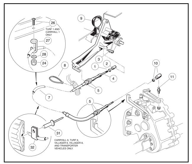
Figure 16-53 Forward/Reverse Shifter Cable
