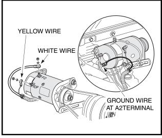
Figure 16-16 Generator Wires
