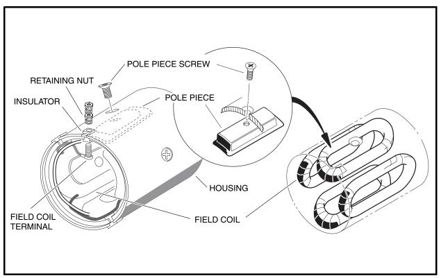
Figure 12-10 Field Coil Assembly
