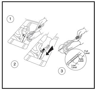
Figure 13-13 Check Engine Oil Level
