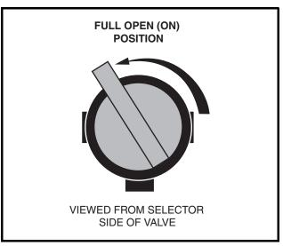
Figure 14-17 Open Fuel Shut-off Valve
