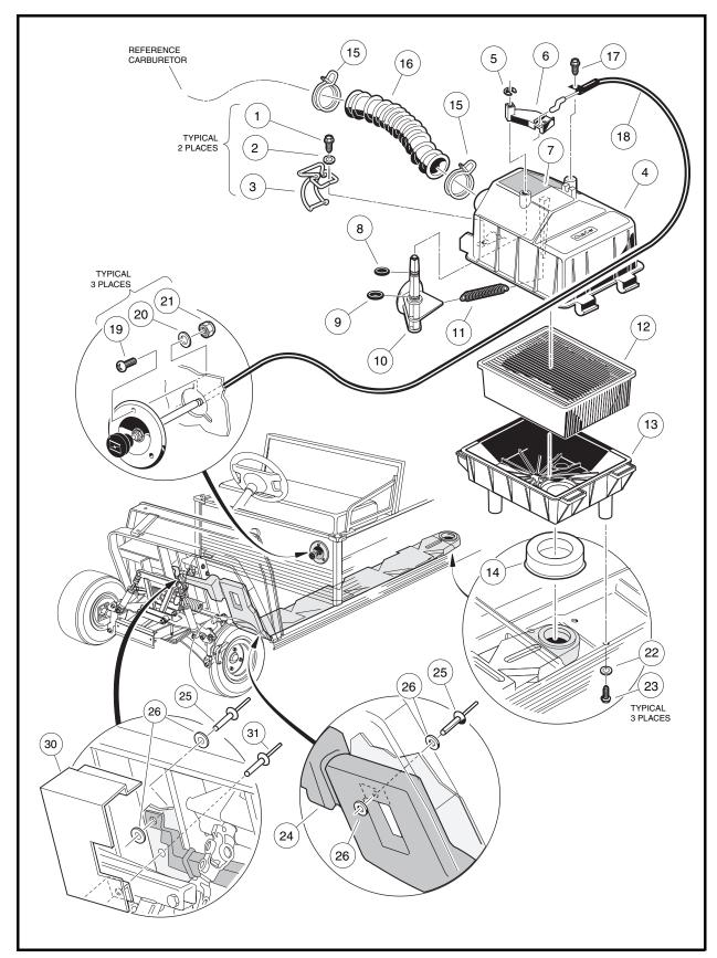
Figure 14-8 Turf 2, Carryall 2 and Carryall 2 Plus Air Intake and Choke Assemblies
