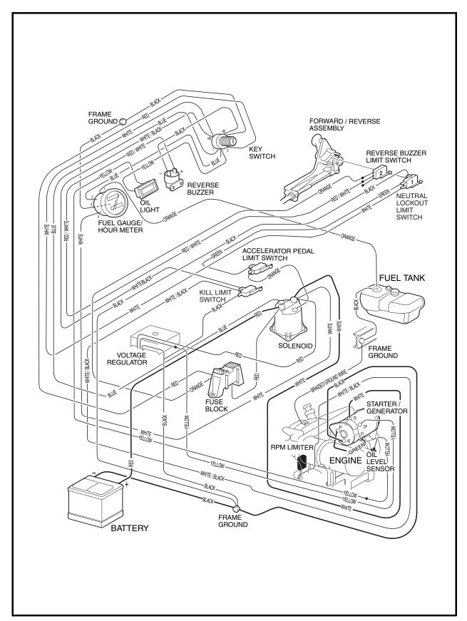
Figure 11-2 Wiring Diagram for Carryall 2
