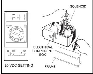
Figure 11-17 Solenoid Continuity Test
