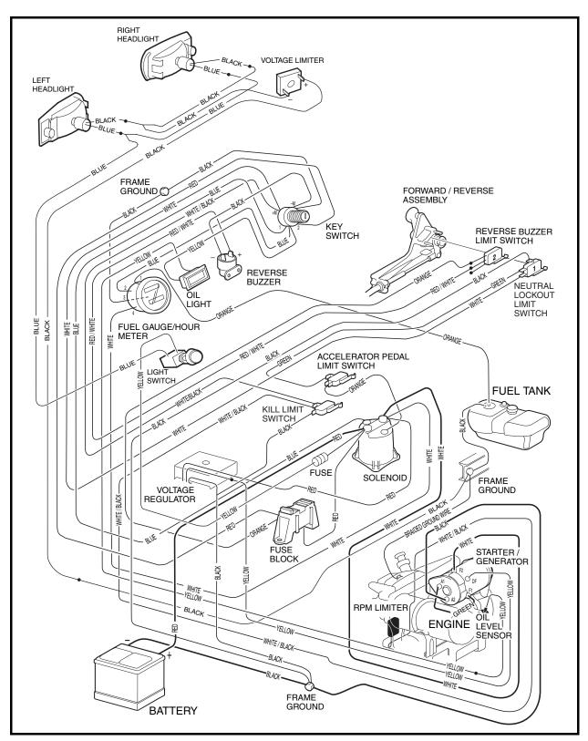
Figure 11-1 Wiring Diagram for Turf 2
