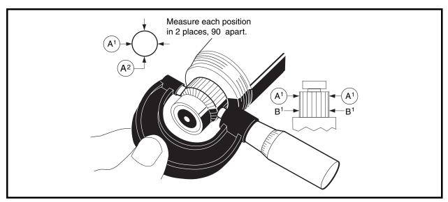
Figure 12-11 Inspect Commutator
