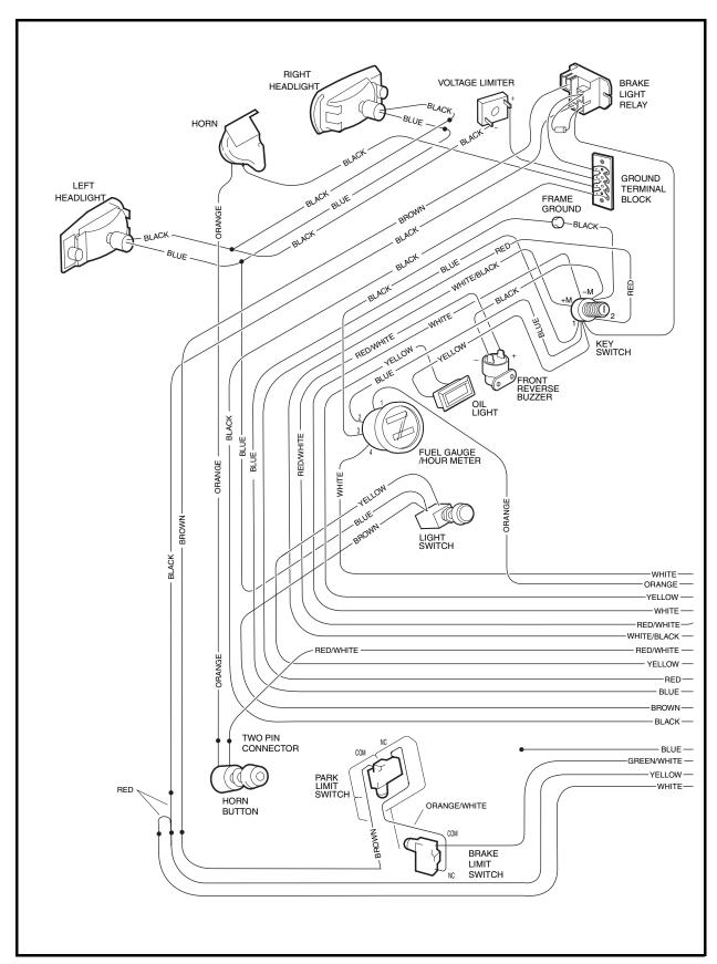
Figure 11-5 Wiring Diagram for Turf 6 Vehicle (Front)
