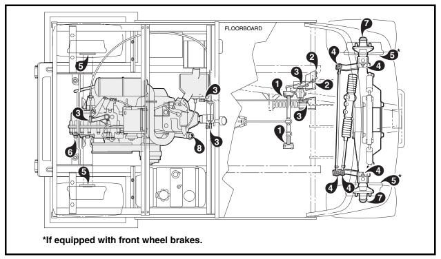
Figure 10-2 Lubrication Points
