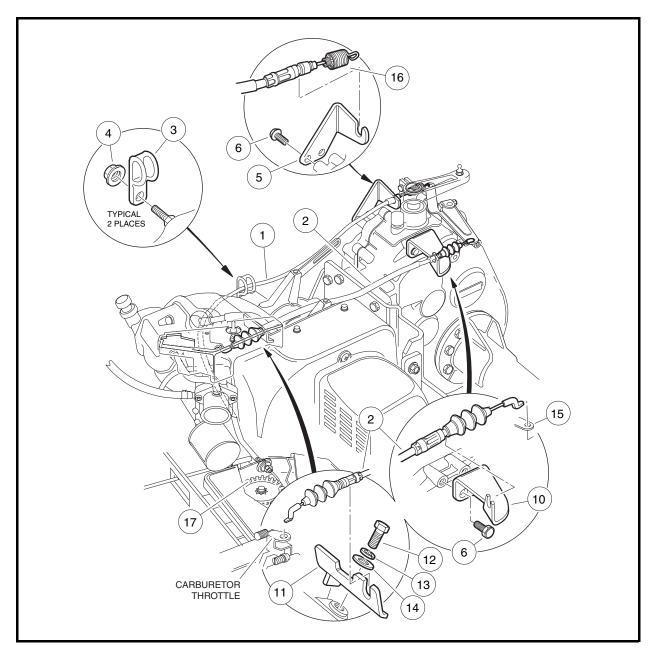
Figure 14-6 Governor and Accelerator Cables
