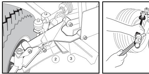
Figure 9-7 Adjust Steering Alignment
