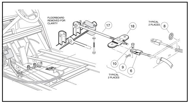
Figure 6-36 Brake Equalizer
