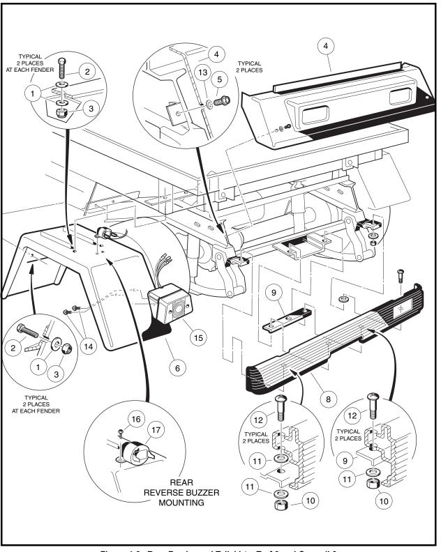
Figure 4-6 Rear Fender and Tailskirt – Turf 6 and Carryall 6
