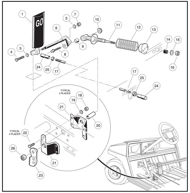
Figure 5-6 Accelerator Pedal – Gasoline Vehicles
