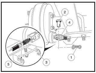
Figure 6-39 Disconnect Cables at Rear Brakes
