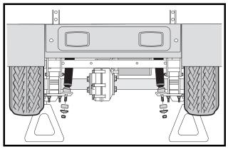
Figure 8-1 Shock Absorber Removal
