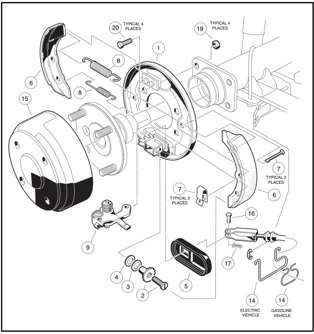
Figure 6-11 Self-Adjusting Brake Assembly
