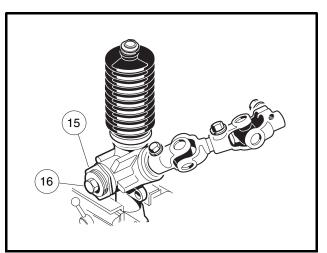
Figure 9-14 Rack and Pinion Adjustment
