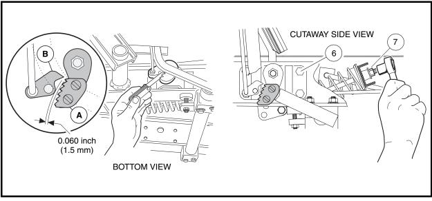
Figure 5-24 Park Brake Ratchet/Pawl Gap Adjustment
