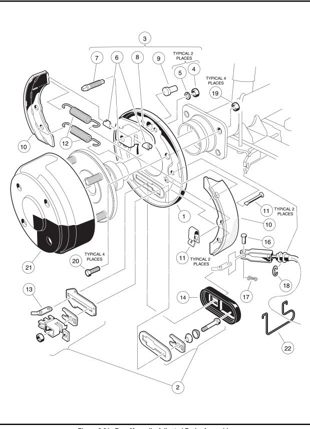
Figure 6-31 Rear Manually-Adjusted Brake Assembly
