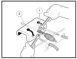
Figure 6-1 Loosen Equalizer Nut
