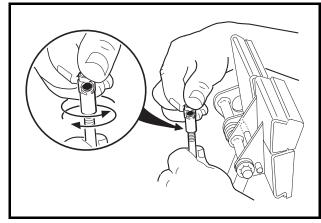
Figure 5-16 Brake Rod Adjustment
