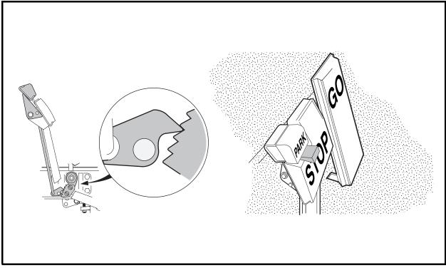
Figure 6-33 Set Park Brake and Insert Wedge
