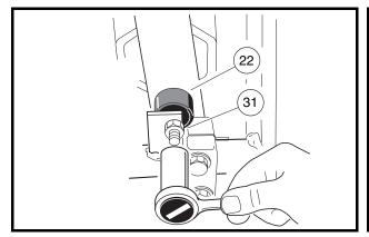
Figure 5-11 Brake Pedal Height Adjustment
