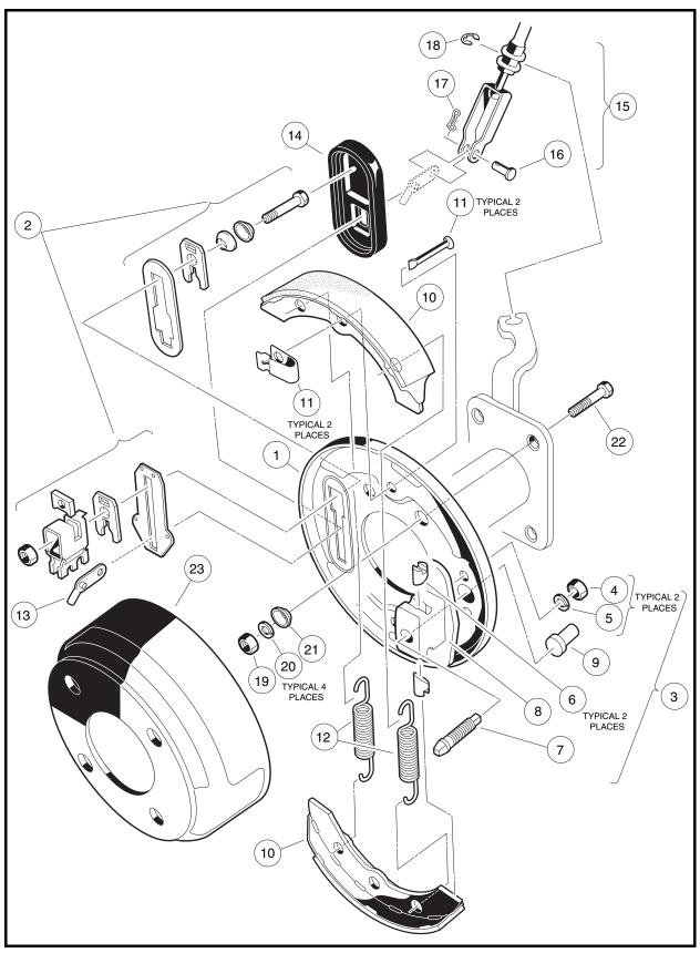
Figure 6-32 Front Manually-Adjusted Brake Assembly
