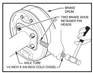
Figure 6-2 Shoe Retainer Pins
