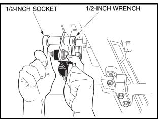
Figure 5-28 Accelerator Pedal Height Adjustment
