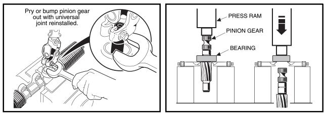
Figure 9-9 Remove Pinion from Housing
