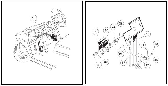
Figure 5-3 Brake Pedal Weldment Through Floor
