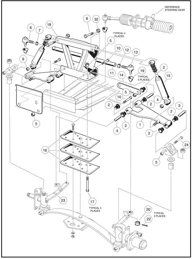
Figure 9-23 Four-Wheel Brake Vehicle – Upper Portion
