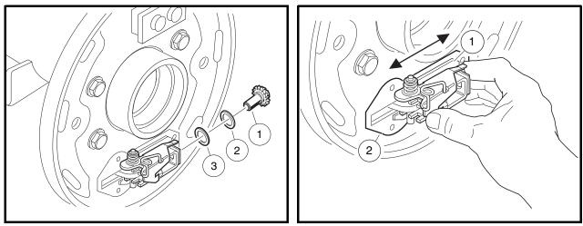
Figure 6-6 Remove Adjuster Wheel
