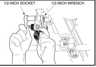
Figure 5-17 Accelerator Pedal Height Adjustment
