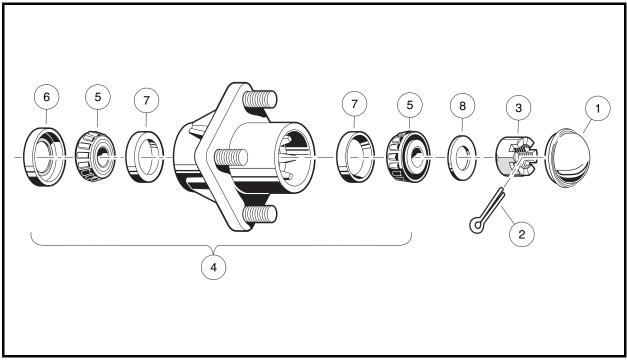
Figure 9-25 Front Wheel Bearings and Hub - Four-Wheel Brake Vehicles
