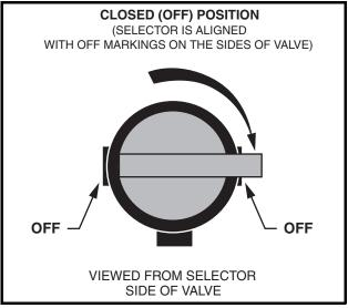
Figure 3-3 Fuel Shut-off Valve – Closed Position
