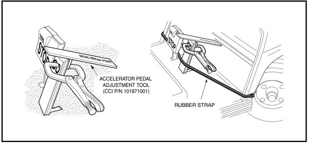
Figure 5-29 Accelerator Pedal Height Adjustment
