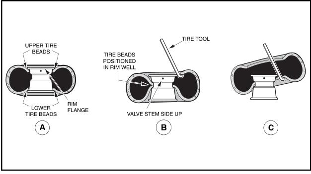
Figure 7-1 Tire Removal
