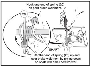
Figure 5-5 Torsion Spring Installation
