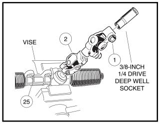
Figure 9-15 Rack and Pinion Resistance
