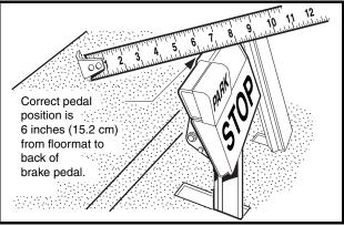
Figure 5-12 Brake Pedal Height Measurement
