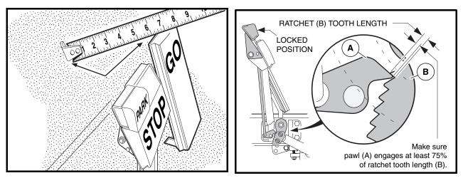
Figure 5-14 Accelerator Pedal Height Measurement
