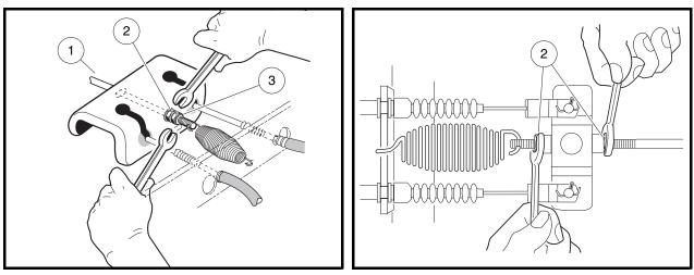
Figure 5-20 Loosen Rear Brake Equalizer Rod Nuts
