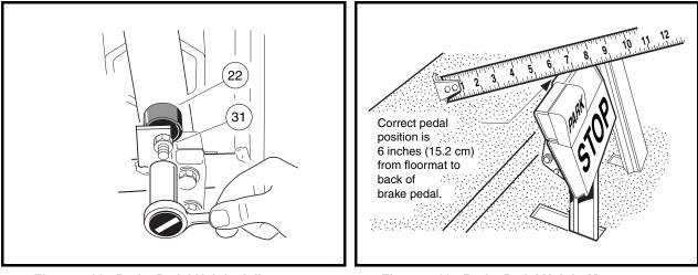
Figure 5-22 Brake Pedal Height Adjustment
