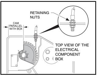
Figure 5-19 Accelerator Cable
