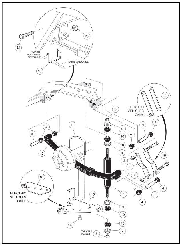
Figure 8-4 Rear Suspension – All Turf and Carryall Vehicles Except Turf 1 and Carryall 1
