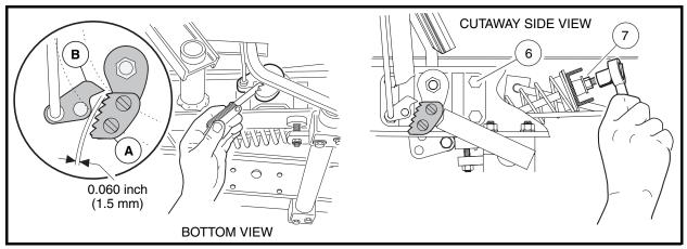
Figure 5-13 Park Brake Ratchet/Pawl Gap Adjustment
