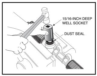
Figure 9-13 Press In Dust Seal
