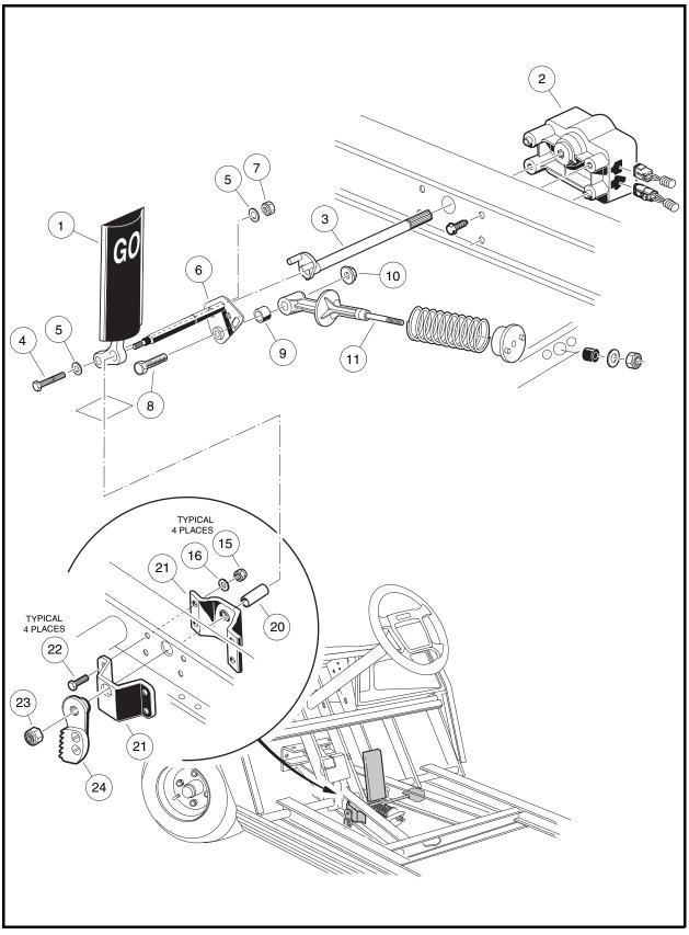
Figure 5-8 Accelerator Pedal – Electric Vehicle
