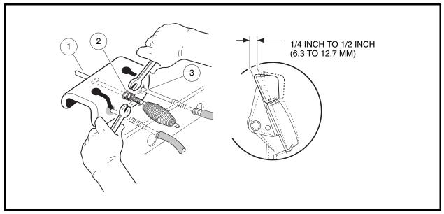
Figure 6-18 Brake Pedal Free Play Adjustment
