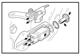
Figure 6-10 Lubricate Adjuster
