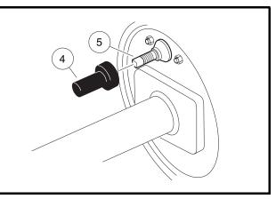
Figure 6-30 Rear Brake Adjustment Bolt
