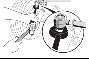
Figure 9-8 Ball Joint Tool
