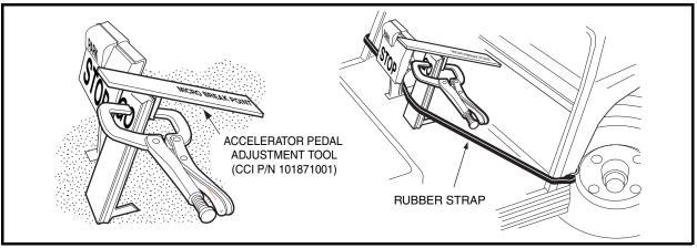
Figure 5-18 Accelerator Pedal Height Adjustment
