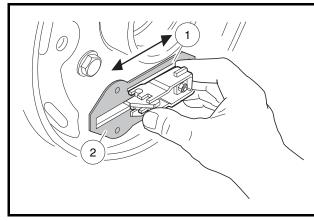
Figure 6-19 Lubricate Slide
