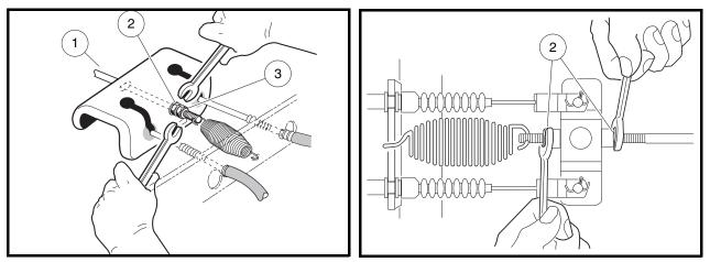
Figure 5-9 Loosen Rear Brake Equalizer Rod Nuts
