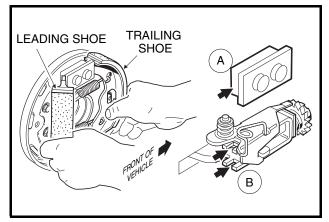
Figure 6-15 Install Leading Shoe
