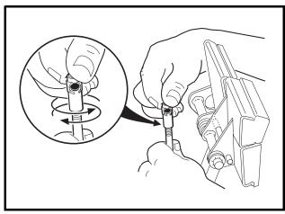
Figure 5-27 Brake Rod Adjustment
