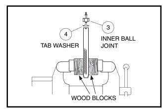
Figure 9-11 Secure Rack in Vise
