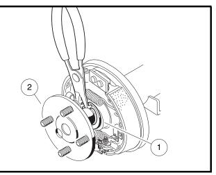
Figure 6-3 Remove Axle Retaining Ring
