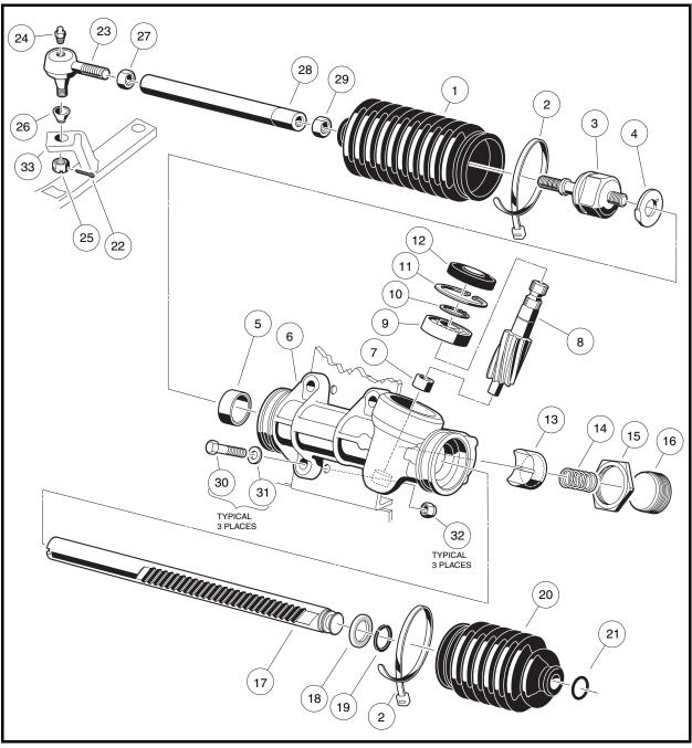
Figure 9-12 Steering Gear
