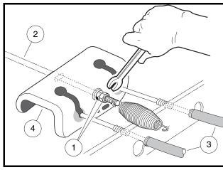
Figure 6-38 Loosen Equalizer Nut
