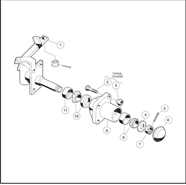
Figure 6-34 Front Spindle Assembly (Four-Wheel Brake Vehicles)
