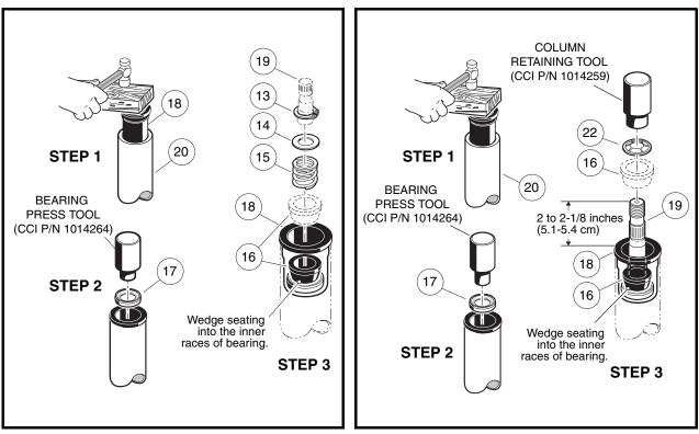
Figure 9-5 Steering Shaft – Bottom End
