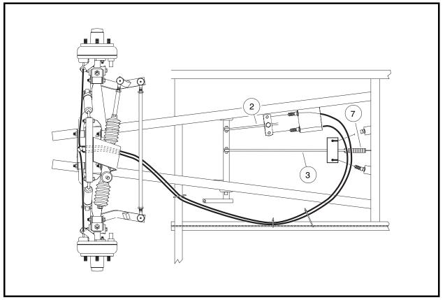
Figure 6-37 Front Brake Cable Routing
