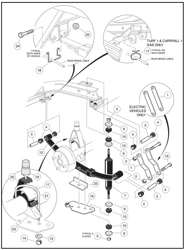
Figure 8-3 Rear Suspension – Turf 1 and Carryall 1 Vehicles
