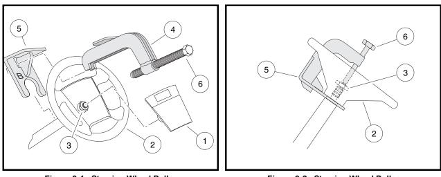
Figure 9-1 Steering Wheel Puller
