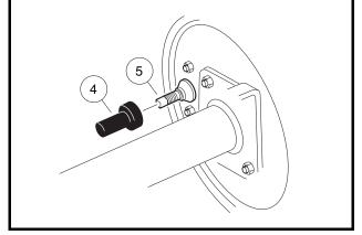
Figure 6-29 Front Brake Adjustment Bolt
