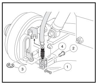
Figure 9-20 Connect Front Brake Cables
