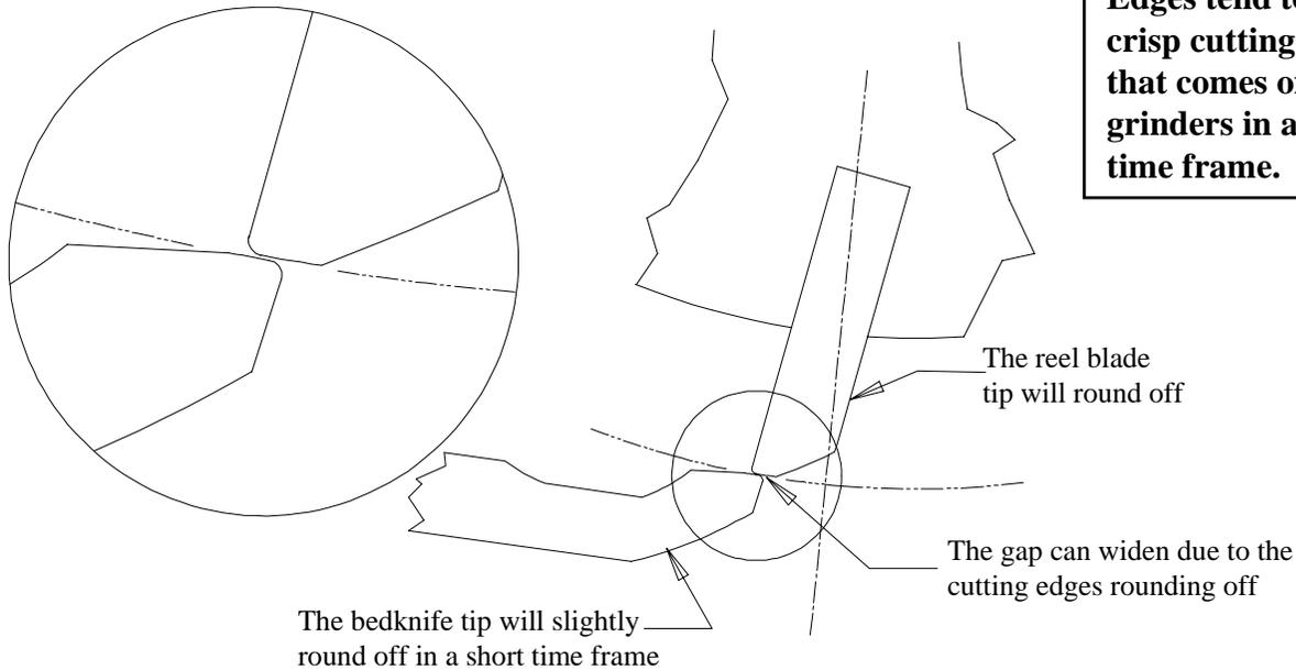
Edges tend to lose their crisp cutting corners that comes off the grinders in a very short time frame.
