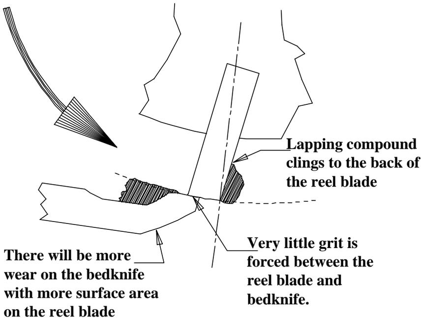
On a flat ground or worn reel, there is so much surface area and metal to remove on the reel blade that it makes the lapping process ineffective and time consuming. This will also cause excess wear to the bedknife and will induce more stress time on the drive systems.
