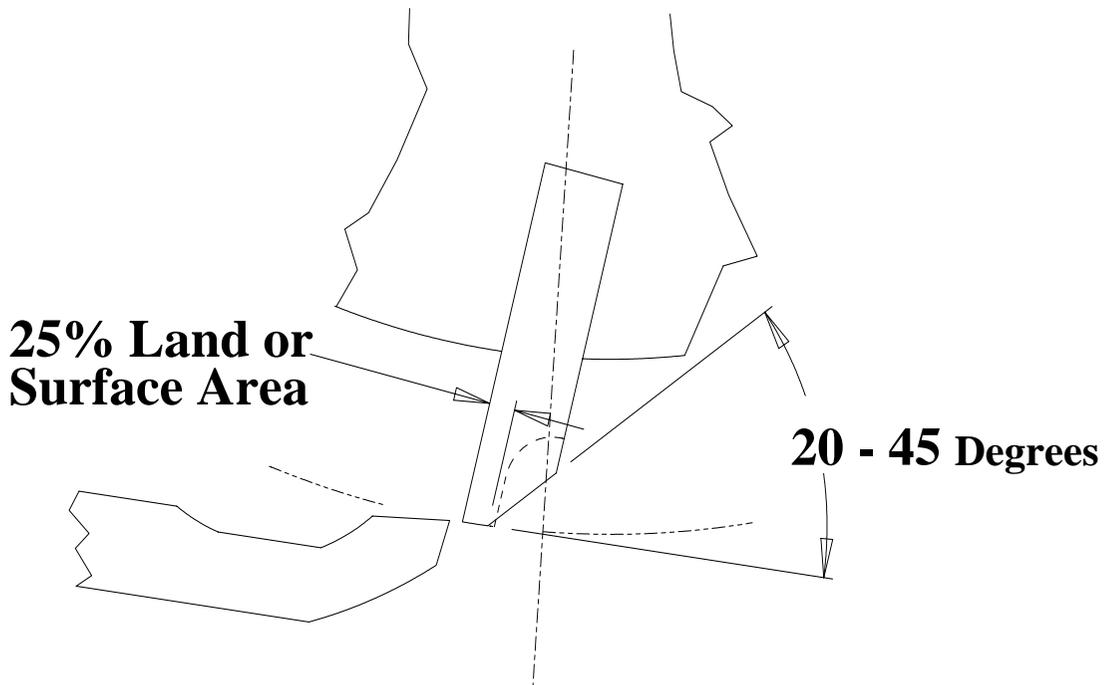
*Reel blades have a back “RELIEF ANGLE” where approximately 75% of the blade is removed. The OEM reel blade configuration has two basic process designs :*
