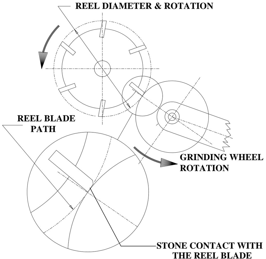
This picture shows how the edge of a reel blade is ground on spin grinders to achieve a sharp edge. Note that both the reel and the grinding wheel rotate in the same direction, causing opposite directional contact at the grind point. This will yield a better grind performance in producing a sharp edge.
