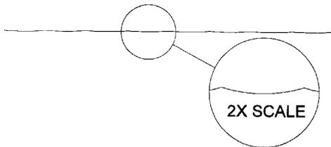
To mow roughs, the top surface can be wavy. Therefore, a 5-bladed reel at lower RPM is acceptable and a close up view might look like this picture at 2X.
