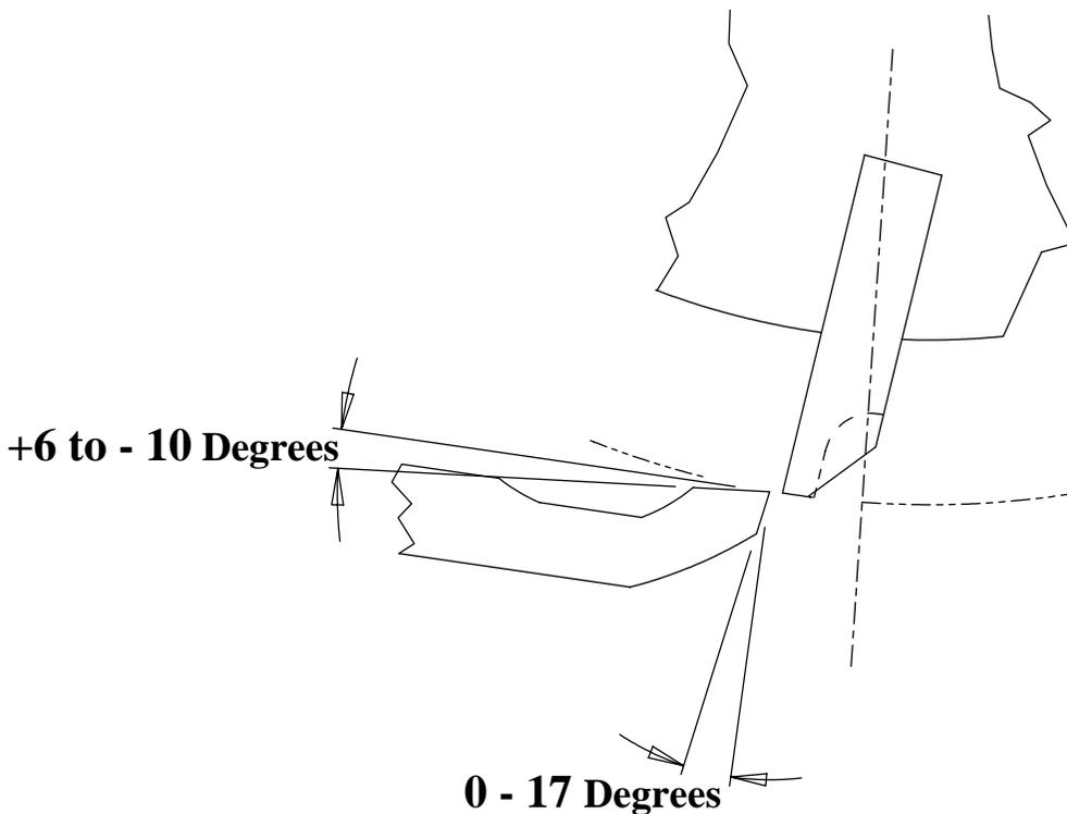
**All bedknife angles are based on the bottom surface of the bedknife. These values are industry averages - for the correct angles of specific models, refer to the mower manufacturers specifications.**
