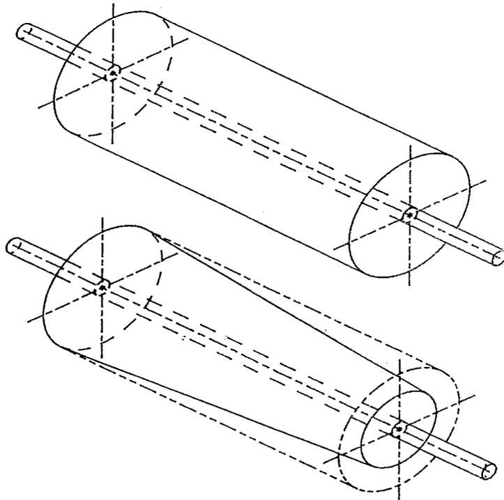
Even reels that are properly adjusted can start to lose their cylindrical shapes and become coned or tapered. As the "relief" wears away through the season and more surface of the reel blade passes the bedknife, the adjustments may accentuate inaccurate wear patterns.
