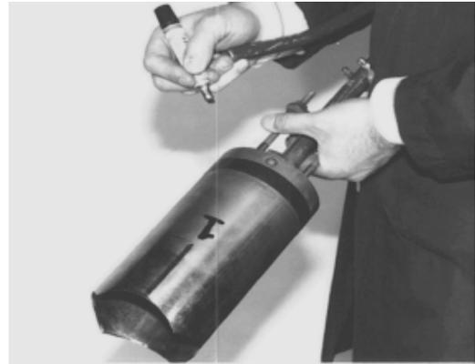
NOTE: The entire hole cutter cutting edge is hardened. When grinding aggressively on the cutting edge, it causes heat buildup. Excess heat buildup causes a softening of the metal and permits a burr to roll over to the outside diameter of the cup. Take quick grinding strokes to minimize heat buildup. Excessive and/or rapid stock removal in one pass creates excessive heat and can also soften the hardened shell.
