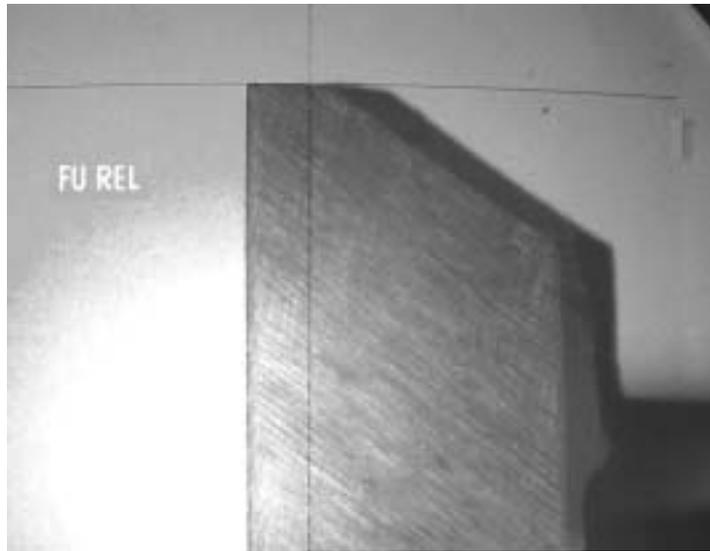
Photo # 3 above is an aftermarket Foley United grind. The reel was spun ground to a sharp edge and the secondary relief was reground in. This shape is one of the primary objectives when taking the time to grind.
