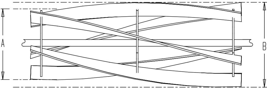
**If diameters A and B are not equal, the reel is CONICAL.**
