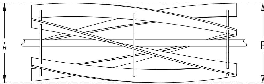
**If diameters A and B are equal, the reel is CYLINDRICAL.**
