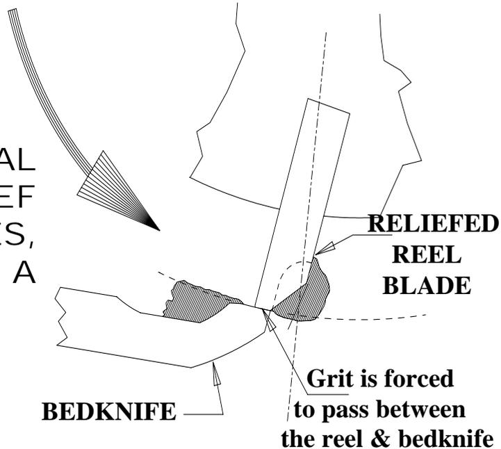
**REASON:** The relief area on the reel blade provides a landing area for the lapping compound to adhere to. This enables the grit to be suspended on the relieved area and is pushed between the reel and the bedknife, thus “effectively” removing metal.
