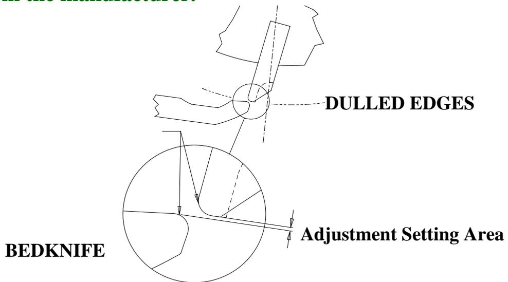
A microscopic review of the reel and bedknife reveals that it takes only **SIX to TEN HOURS** of operation for a crisp sharp edge to begin to round off. This can result in a widening of the gap between the cutting edges when the machine is through cutting for the day.
