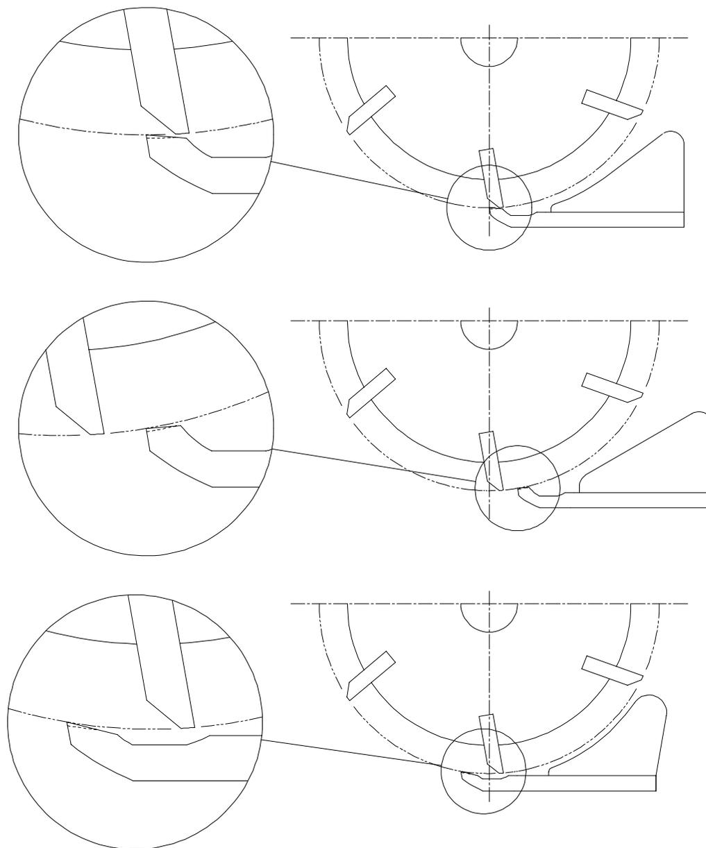
The bedknife position has a specific wear pattern as the reel blade sweeps over the bedknife, and the wear angle depends on the position and attitude of the knife. The pictures above illustrate the three primary positions of the bedknife cutting edge in relation to the centreline of the reel: even, behind or forward of the centreline.
