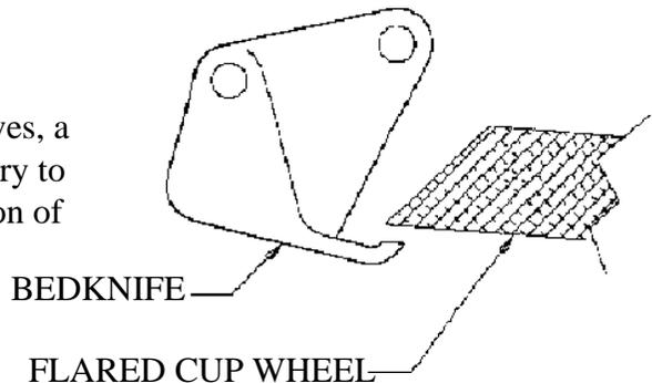
**Dressing the grinding wheel is important to the quality of grind. A grinding wheel which is loaded will cause excessive heat build up and can cause an irregular grind. The best dressing method is a diamond dresser rigidly mounted in relation to the grinding wheel. Other methods which can be used are hand held diamond dressers and hand held dressing bricks. Hand held dressers are difficult to use and makes it more difficult to achieve an accurate wheel dressing.**
