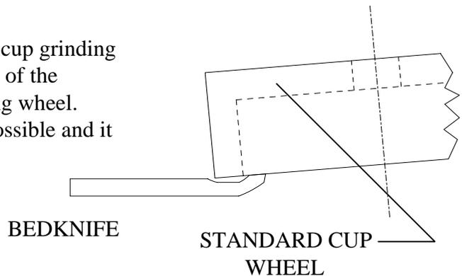
This picture shows that on some bedknives, a special flared cup wheel may be necessary to avoid hitting the “ears”, or casting portion of the bedbar.
