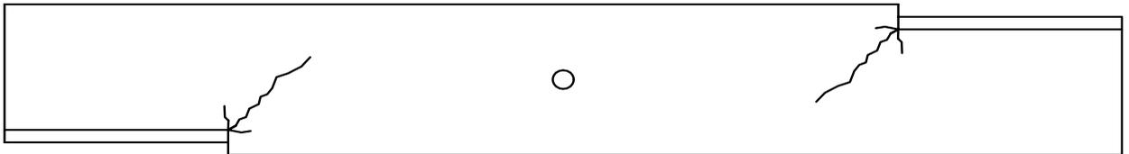
A step grind in which the cutting edge is ground at a perpendicular angle can create stress points, making the blade tip area more susceptible to cracking. A “hook” grind can have this same effect where if the tip hit something hard, it is more prone to cracking and/or breaking off.
