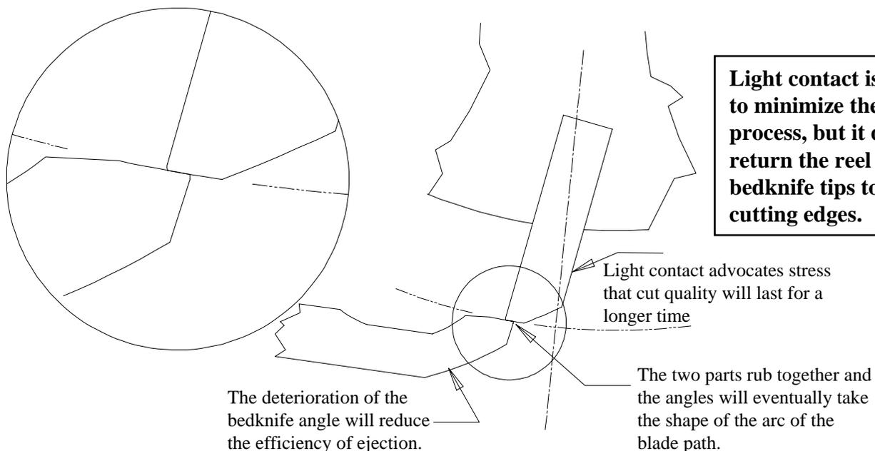
Light contact is thought to minimize the dulling process, but it does not return the reel blade or bedknife tips to crisp cutting edges.
