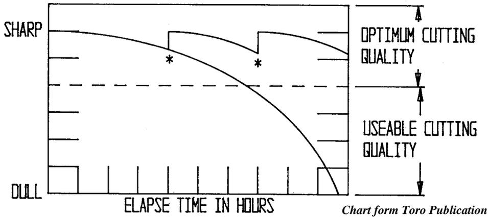
*Note that you want to take corrective action prior to dropping out of the “OPTIMUM CUTTING QUALITY” range.*
