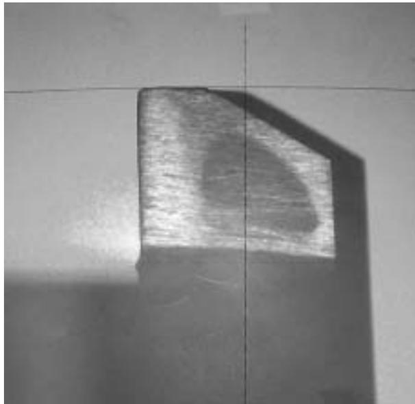
Photo # 4 above is a NEW OEM DESIGNED blade as it looks from the manufacturer. The relief portion of the reel reduces friction and stress on the hydraulic, engine and drive systems, and will reduce the grind frequency through the course of a season.
