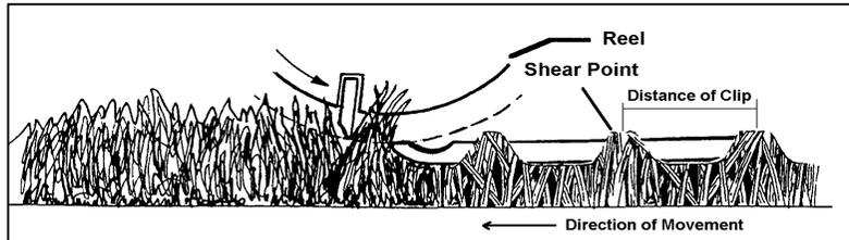
As the reel rotates, the front edge of the reel travels along a "BLADE PATH" and gathers the grass in a clump as illustrated above. The end result of this cutting action leaves 20-30% of grass mass that is not cut at the "shear" point. Different diameter reels will have their own unique "blade path", thus a unique surface clip based on blade count, reel diameter, RPM, and mow speed.
