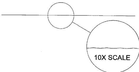
To mow greens, the desired surface is smooth and an 11-bladed reel at a high RPM is best. A closer view at 10X illustrates a flatter surface is achieved for putting purposes.
