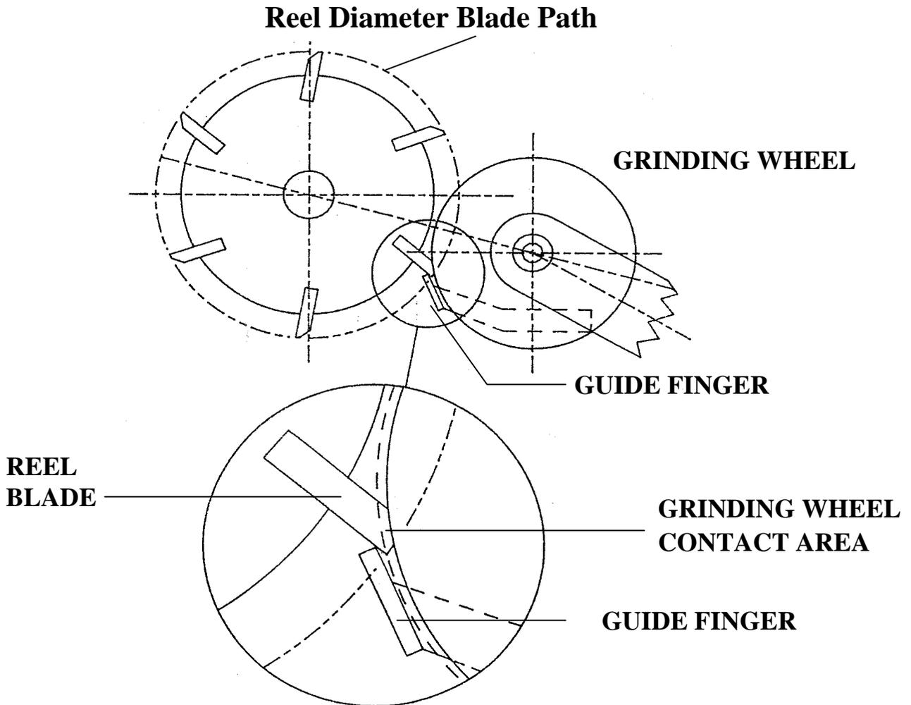
These pictures demonstrate how a reel is set up on a single blade grinder to achieve the desired angle on the edge of the blade. The grinding wheel turns and the reel does not as each reel blade is ground separately. The height of the grinding wheel will dictate the angle on the reel blade, as the reel blade rests on the guide finger.
