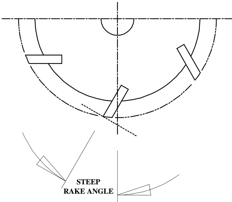
A closer inspection of a spun ground reel will illustrate that the ground surface is at an angle with the blade body. This visual angle should not be confused with “relief”, as relief will always require a secondary grind process. Note the angle of the blade face in relation to cutting path of the reel blade and the blade body. The entire blade face surface will pass over the cutting edge of the bedknife.
