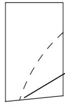
**Figure 6:** The dashed line on the reel blade illustrates the “milled-in” relief area of a greens or tee mower. The solid line shows the secondary relief that can be attained by lowering the grinding head after grinding to a sharp edge with the near flat grind as illustrated in figure 5.
