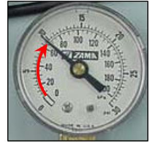
Step 3: Attach tester to primer return hose. Push primer bulb; gauge should indicate pressure and hold. If not, purge primer is faulty.
