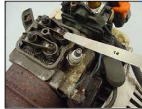
10. Set valve clearance to 0.1 mm (0.004") when cold. 0.1 to 0.3 mm (0.004" to 0.012") is acceptable.
