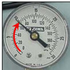
Step 1: Attach primer line to primer line fitting and attach tester to fuel line fitting. Pressurize carburetor to 10 psi (0.7 bar). If pressure holds, the fuel pump components and inlet needle are sealing. Go to step 2.
