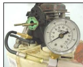
Connect carburetor tester to impulse hose while performing pressure and vacuum tests. Gauge should move while performing tests.
