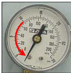
Step 2: With pressure present from step 1, push primer bulb until gauge indicates a slight vacuum. Vacuum should hold for minimum of 1 second. If not, carburetor has an internal leak.
