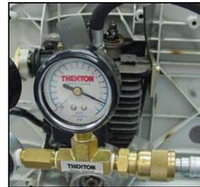
11. Perform cylinder leak down test. Maximum of 10% leakage is acceptable.
