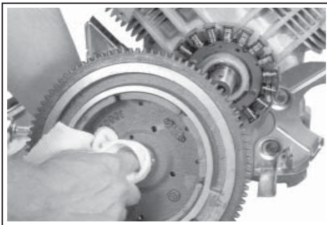
Figure 11-27. Clean and Dry Flywheel Hub.
