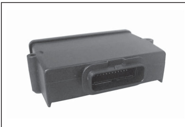
Figure 5B-2. “24 Pin” (MSE 1.0) Plastic-Cased ECU.
