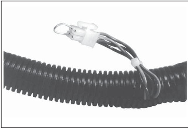
Figure 5B-8. Service Connector Plug, Metal-Cased ECU Harness.
