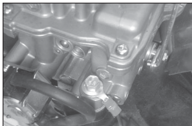
Figure 11-77. Ground Lead on Carburetor Mounting Screw (One-Barrel Carburetor).
