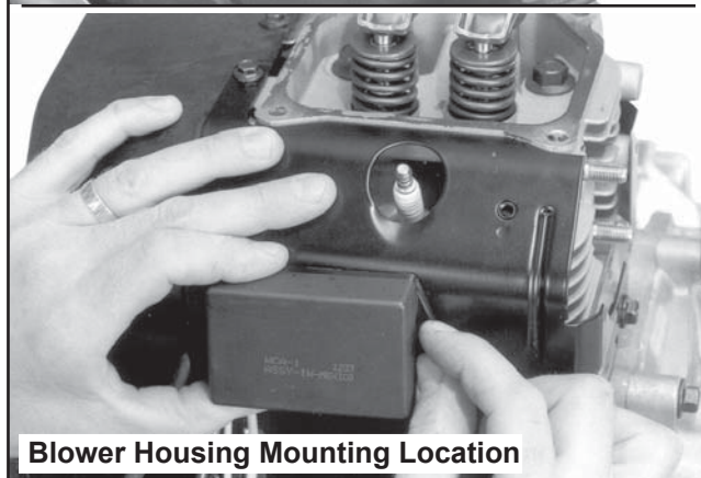
Figure 11-72. Reinstalling SAM Module.
