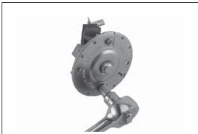
Figure 8-63. Removing Brush Holder.
