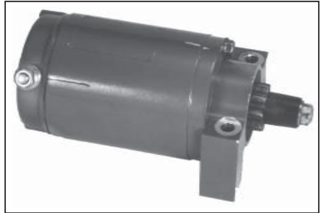
Figure 8-45. Starter Assembly Match Marks.
