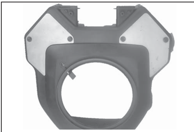
Figure 4-15. Cleanout Kit Installed on Blower Housing.
