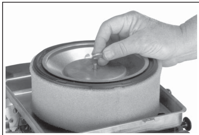
Figure 4-5. Removing Element Cover Wing Nut.
