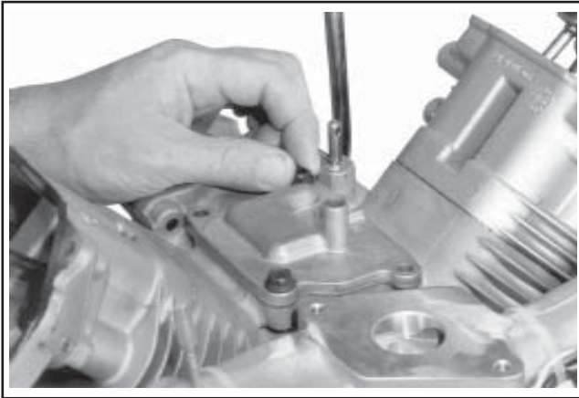
Figure 11-58. Installing Screws (Locations 3 and 4).
