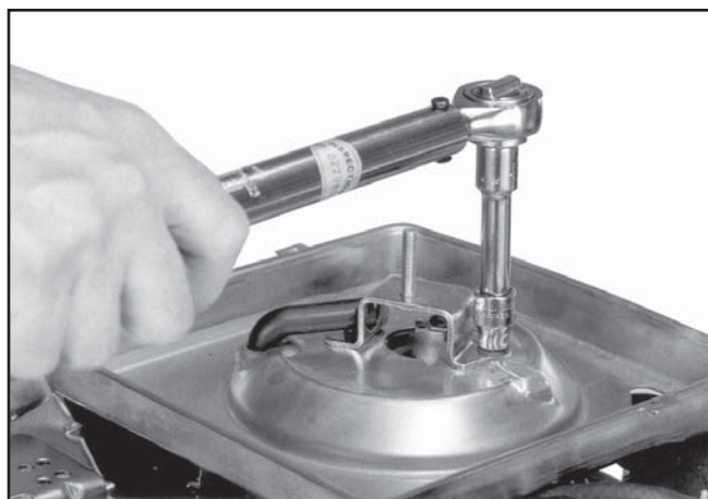
Figure 11-94. Torquing Base Screws.
