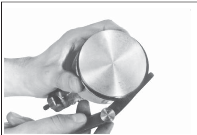
Figure 10-10. Measuring Piston Ring Side Clearance.
