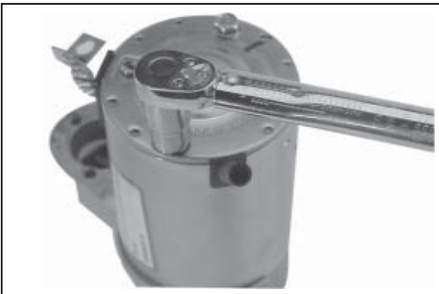
Figure 8-75. Torquing Thru Bolts.
