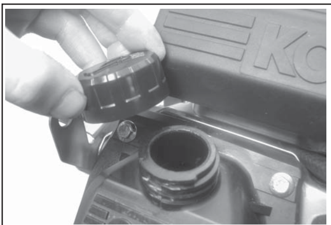
Figure 9-3. Removing Oil Fill Cap from Cover.
