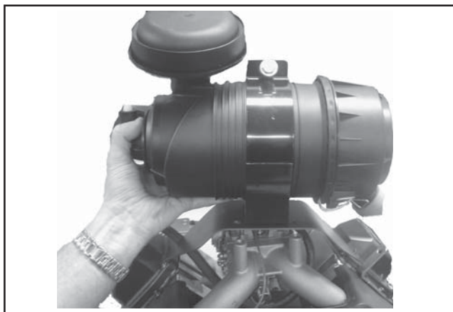
Figure 9-14. Removing Heavy Duty Air Cleaner Assembly (Two-Barrel Model Pictured).
