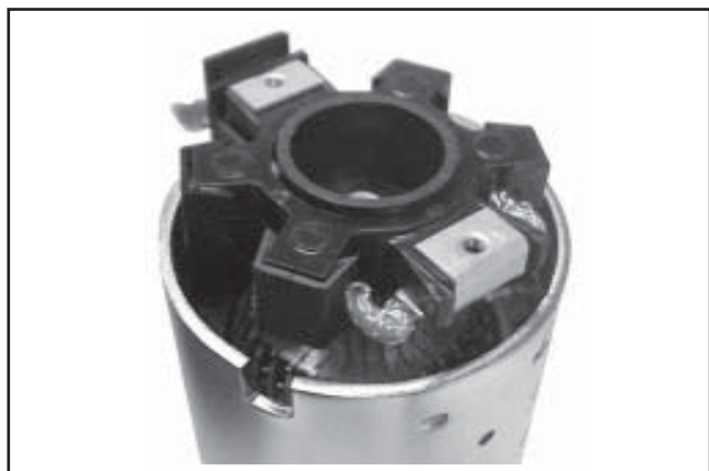
Figure 8-71. Installing Brush Holder Assembly with Supplied Tube.
