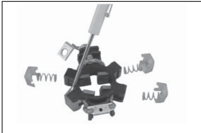
Figure 8-72. Removing Retaining Clips.
