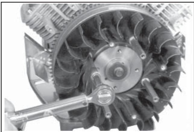
Figure 11-33. Torquing Supports for Metal Screen (Some Models).
