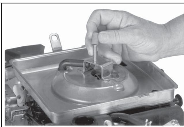
Figure 4-7. Removing Rubber Seal from Bracket.
