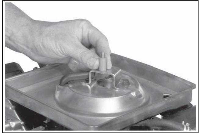
Figure 9-8. Removing Air Cleaner Base Retainer.
