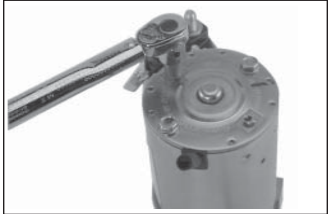
Figure 8-76. Torquing Brush Holder Screws.
