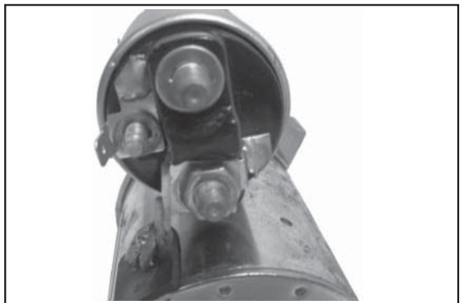
Figure 8-77. Positive (+) Brush Lead Connection.
