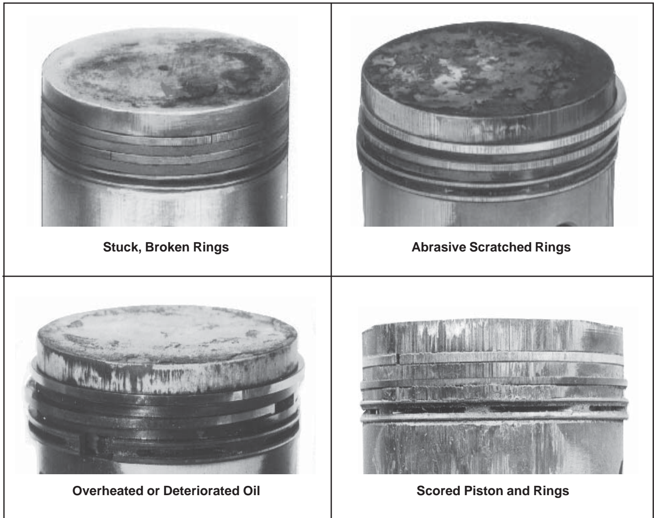
Figure 10-8. Common Types of Piston Damage.
