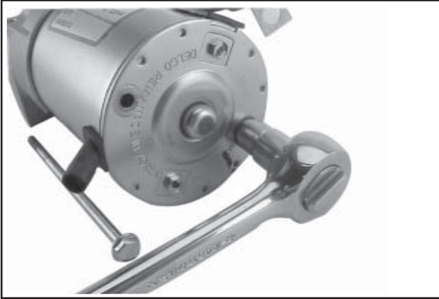
Figure 8-52. Removing Thru Bolts.
