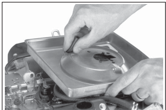
Figure 9-10. Removing Breather Tube from Base.
