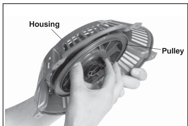
Figure 7-6. Removing Pulley from Housing.
