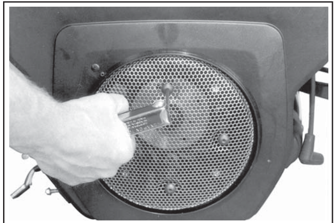
Figure 9-36. Removing Metal Grass Screen.
