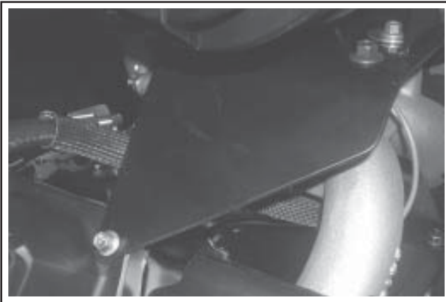
Figure 11-97. Mounted Air Cleaner Bracket (Two-Barrel Carburetor).
