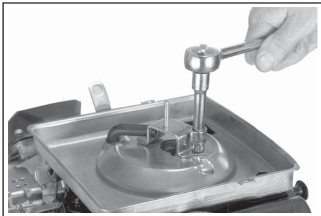
Figure 4-9. Bracket Retaining Screw.
