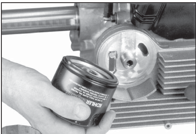
Figure 11-101. Installing New Oil Filter.
