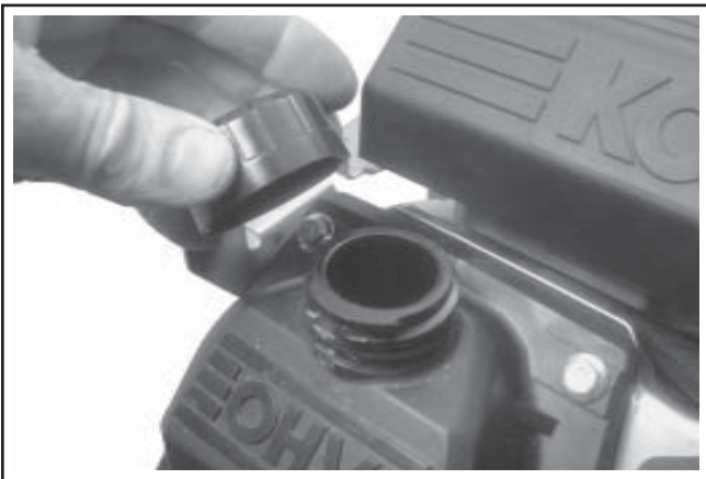
Figure 11-105. Reinstalling Oil Fill Cap (Some Models).
