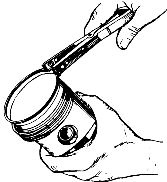
FIGURE 13. REMOVING PISTON RINGS
