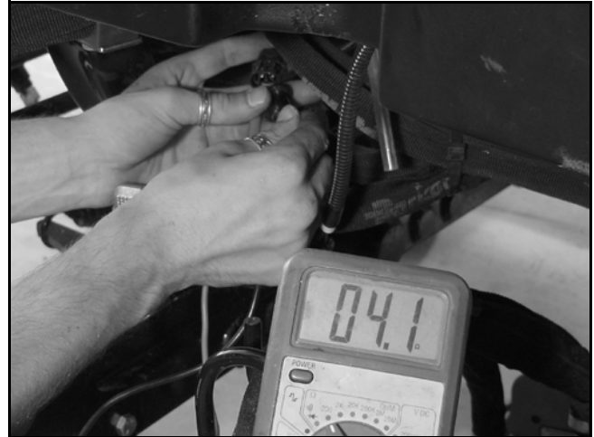
Figure 10I-9. Coil Resistance Test
