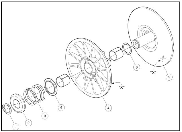
Figure 13a-32 Driven Clutch Assembly
