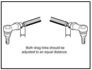
Figure 7-23 Adjust Both Drag Links
