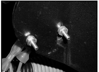
Figure 12a-8 Reverse Warning Buzzer Limit Switch Adjustment Slot
