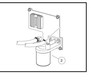
Figure 10a-9 Replace Engine Oil Filter – Gasoline Vehicles
