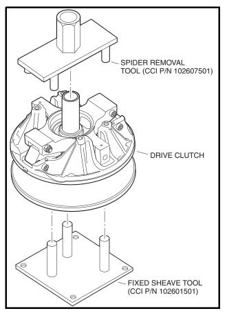
Figure 13c-31 Drive Clutch Service Tools
