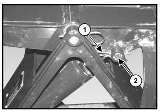
Figure 16-39 Remove Rod End Pins
