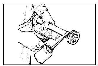
Figure 16-69 Lubricate Piston Seal
