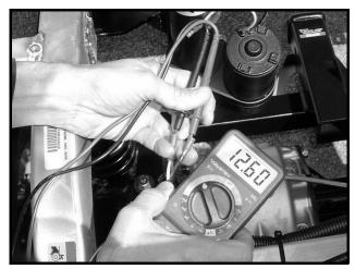
Figure 11c-49 Bed Lift Motor Voltage Reading with Switch in UP position
