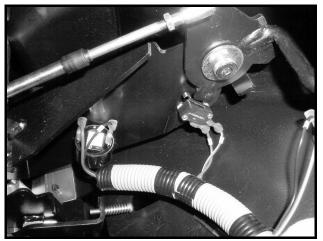
Figure 12b-6 Reverse Warning Buzzer and Limit Switch
