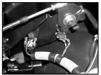
Figure 12c-7 Reverse Warning Buzzer and Limit Switch
