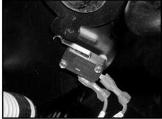
Figure 12a-9 Reverse Warning Buzzer Limit Switch (Properly Adjusted)
