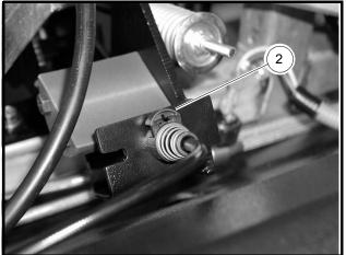
Figure 13a-15 Accelerator Cable Pedal Bracket (Gasoline Vehicles)
