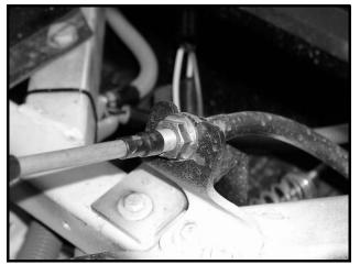
Figure 14-23 Forward/Reverse Shifter Cable Flanged Nuts At Shifter Handle Bracket
