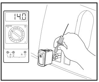
Figure 11b-30 Light Switch Test
