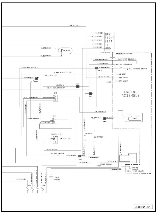
Figure 11a-2 Wiring Diagram – Kawasaki Powered Gasoline Carryall 295 and XRT 1550 Vehicles (Rear)
