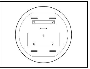
Figure 11a-30Fuel Gauge/Hour Meter – Late 20071. Black(Jumper Wire From 6 2. Blue 4. Orange 6. Black 7. White
