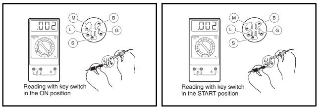
Figure 11a-8 Key Switch Test – Accessory Terminal
