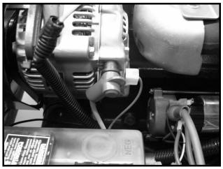
Figure 11c-35 60-Amp Fusible Link
