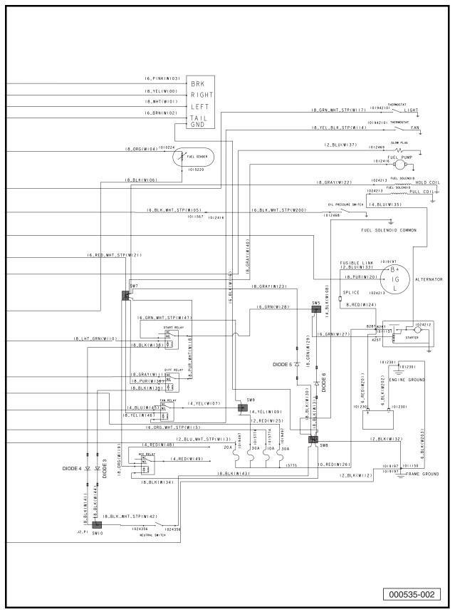
Figure 11c-2 Wiring Diagram (2 Piece Harness) for Diesel Carryall 295 and XRT 1550 Vehicles (Rear)
