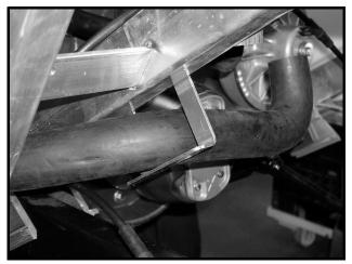
Figure 13b-27 Air Intake Support Bracket
