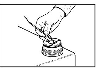
Figure 16-48 Remove O-ring and Back-up Washer
