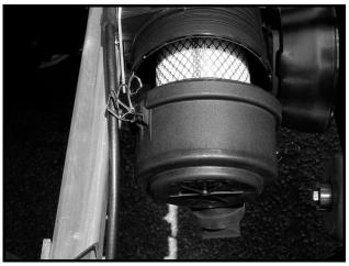
Figure 13b-24 Air Filter Cartridge
