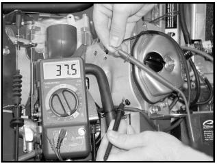
Figure 11b-26 Carburetor Solenoid Coil Resistance
