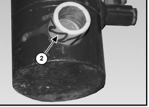
Figure 16-74 Apply LOCTITE and Install Bushings Into Base
