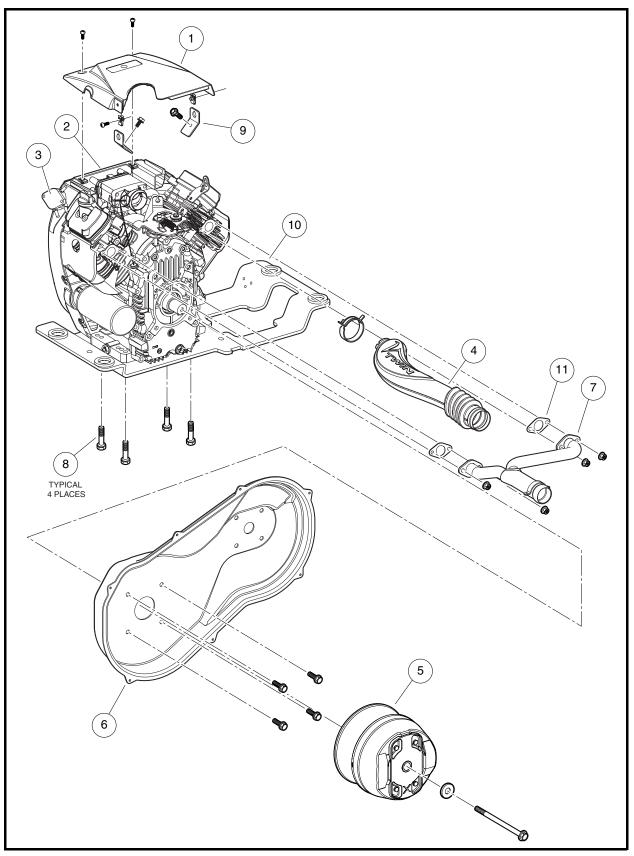
Figure 13a-1 Engine Removal and Installation Components
