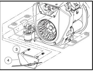
Figure 13a-18 Choke Cable on Engine
