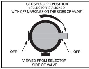
Figure 13b-9 Closed Fuel Shut-Off Valve
