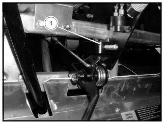
Figure 13b-23 High-speed Adjustment Screw
