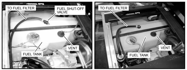
Figure 3-2 Fuel Tank – Gasoline Vehicles
