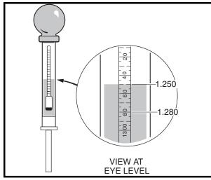
Figure 11c-7 Hydrometer Test
