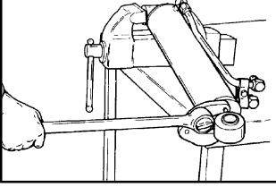
Figure 16-43 Loosen the Head
