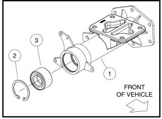
Figure 14-27 Rear Wheel Bearing
