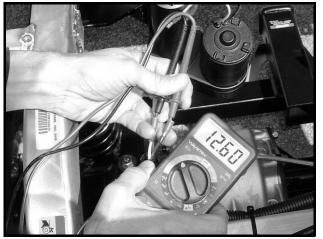
Figure 11b-33 Bed Lift Motor Voltage Reading with Switch in UP position
