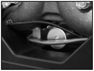
Figure 12a-3 Carburetor Solenoid Connector
