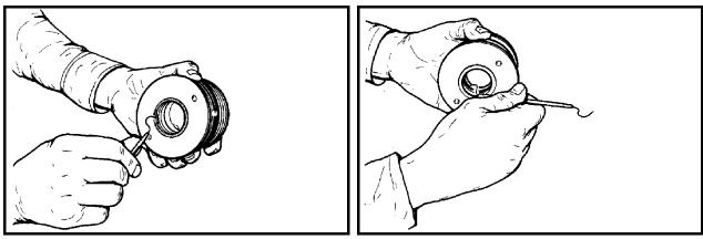
Figure 16-49 Remove Wiper Seal
