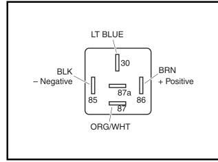
Figure 16-26 Relay 1 Wiring and Testing
