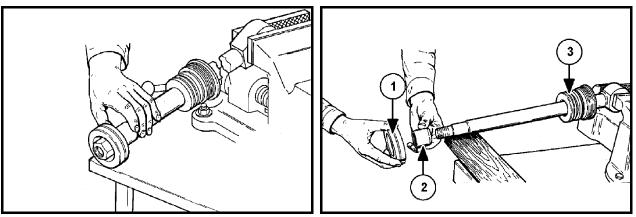
Figure 16-45 Remove Nut from Piston
