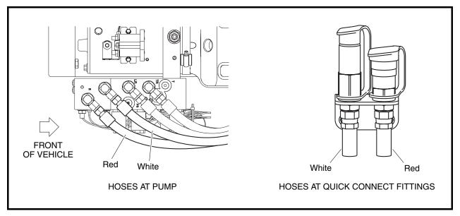
Figure 16-35 Auxiliary Circuit Hoses
