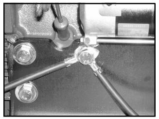
Figure 11c-11 Engine Ground (Under Starter)
