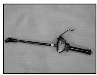
Figure 7-3 Steering Column Assembly
