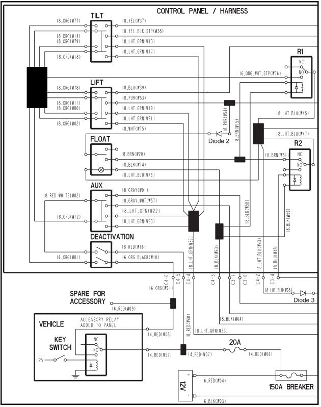
Figure 16-18 Wiring Diagram for Hydraulic Attachment System Vehicles (Front)
