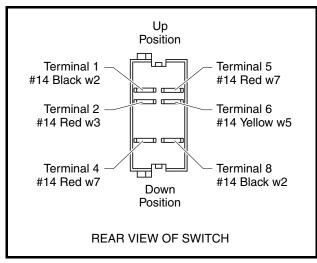
Figure 11c-51 Bed Lift Switch Terminals
