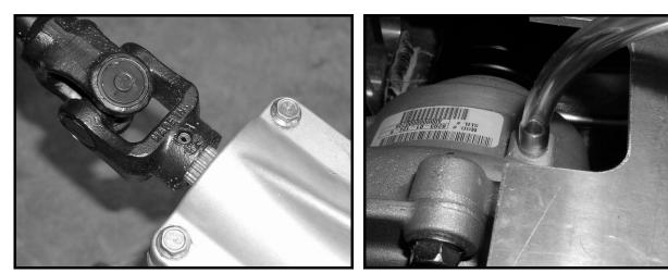
Figure 14-8 Roll Pin in Driveshaft and Pinion Shaft
