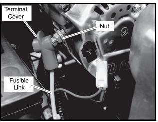
Figure 12c-5 60-Amp Fusible Link
