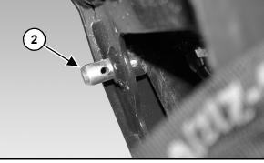
Figure 16-41 Remove Pivot Pin
