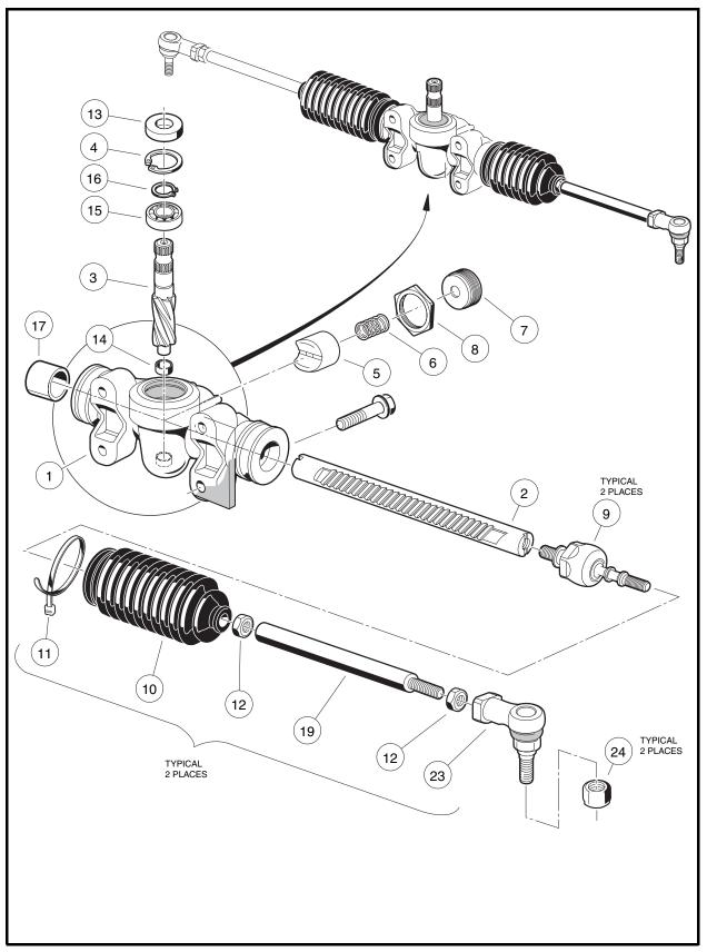
Figure 7-16 Steering Gear Assembly
