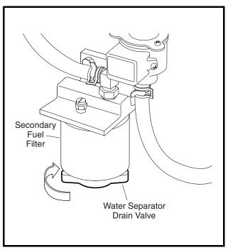
Figure 13c-9 Water Separator Drain Valve
