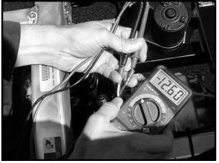
Figure 11b-34 Bed Lift Motor Voltage Reading with Switch in DOWN position
