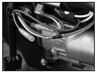
Figure 11a-16 Carburetor Solenoid Bullet Connector
