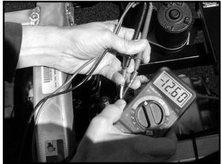
Figure 11c-50 Bed Lift Motor Voltage Reading with Switch in DOWN position
