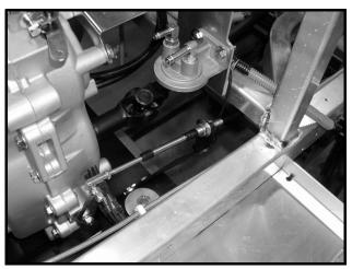
Figure 14-24 Forward/Reverse Shifter Cable at Transmission
