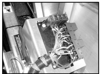
Figure 11c-28 Differential Relay Removed – Early 2007 Only
