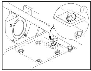
Figure 10b-8 Engine Oil Drain Plug and Pan – Gasoline Vehicles
