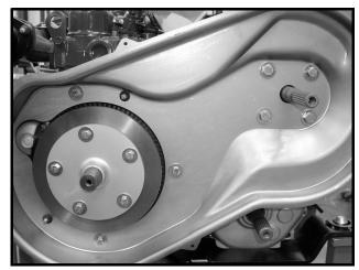
Figure 13c-35 Diesel Inner Cover Assembly
