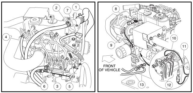
Figure 13c-1 Disconnect Coolant Hoses, Fuel Lines, Accelerator Cable and Fuel Solenoid Valve Connector
