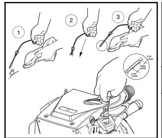
Figure 10b-6 Engine Oil Level Check – Kawasaki Powered Gasoline Vehicles
