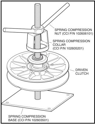
Figure 13c-33 Driven Clutch Service Tools
