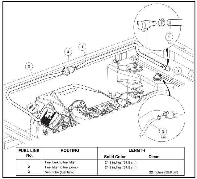
Figure 13a-5 Fuel System (Kawasaki Powered Gasoline Vehicles)
