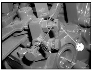
Figure 13c-23 High-Speed Throttle Adjustment Screw
