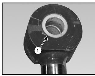
Figure 16-75 Remove Bushings from Rod End
