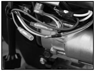
Figure 11a-27 Carburetor Solenoid Bullet Connector
