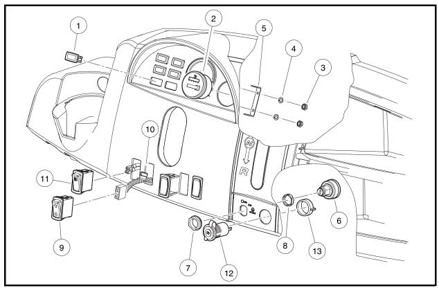
Figure 12b-5 Instrument Panel Electrical Components
