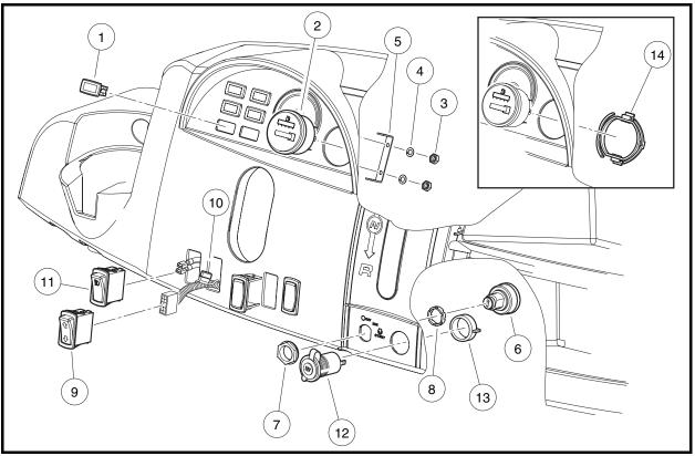
Figure 12a-6 Instrument Panel Electrical Components
