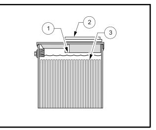
Figure 11c-8 Battery Electrolyte Level 1. Level Indicator 2. Cap 3. Plates Electrolyte level at least 1/2 inch (13 MM) above plates or to level indicator.
