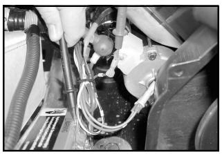
Figure 11b-11 Starter Circuit Test
