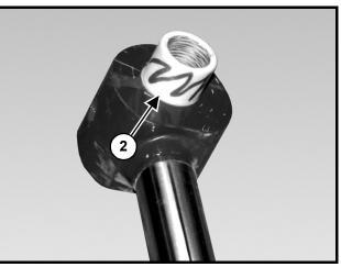
Figure 16-76 Apply LOCTITE and Install Bushings Into Rod End
