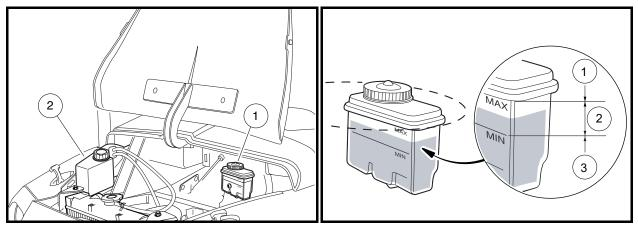
Figure 10a-4 Brake Fluid and Engine Coolant Access
