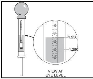
Figure 11a-3 Hydrometer Test
