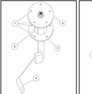
Figure 13b-5 Fuel Level Sending Unit Alignment
