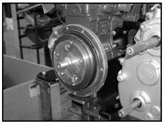
Figure 13c-36 Diesel Inner Cover Spacer
