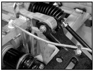
Figure 6-19 Front Brake Line Support Brackets
