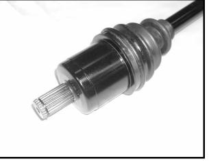
Figure 14-6 Compression Ring on Spline
