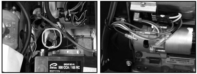
Figure 11a-23 Engine Harness Connector
