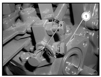
Figure 13c-22 Idle Throttle Adjustment Screw
