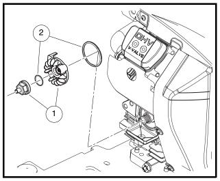
Figure 13a-2 Secure Oil Adapter to Engine
