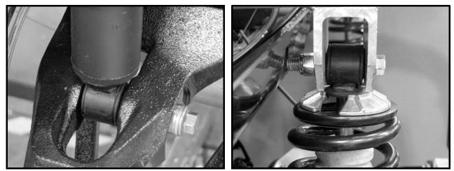
Figure 7-35 Front Shock Bottom Mount
