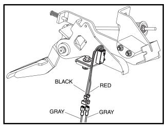
Figure 11c-34 Front Differential Switch
