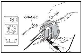
Figure 11c-42 Fuel Gauge Voltage Test - Terminal 2
