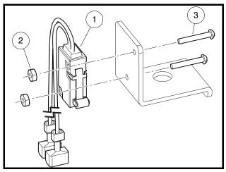
Figure 12c-10 Front Differential Limit Switch Removal
