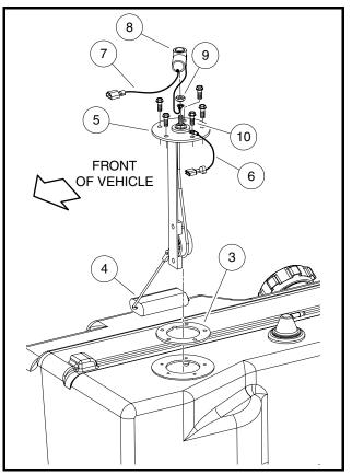
**NOTE:** The rheostat arm and float should be positioned toward the outside surface of the fuel tank.
