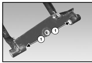
Figure 16-79 Remove Four Pivot Bushings
