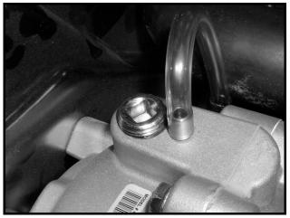
Figure 14-21 Lubrication Fill Plug and Vent Tube
