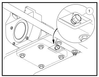
Figure 10a-8 Engine Oil Drain Plug and Pan – Gasoline Vehicles
