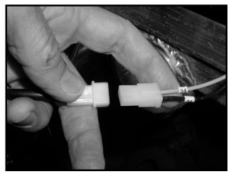
Figure 14-10 Differential Clutch Connector
