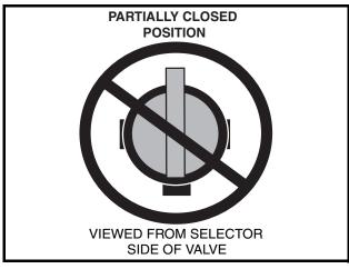
Figure 13a-13 Incorrect Fuel Shut-Off Valve
