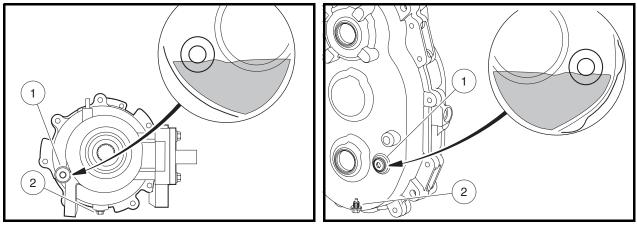
Figure 10a-17 Front Differential Lubrication Level
