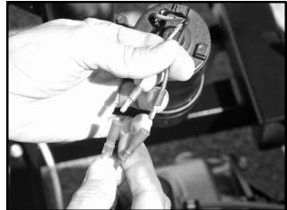
Figure 11c-48 Bed Lift Motor Wires
