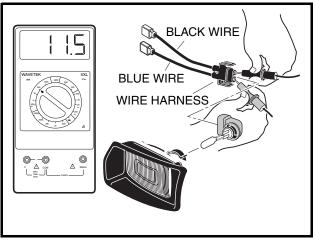
Figure 11a-36 Voltage Measurement at Headlight Socket
