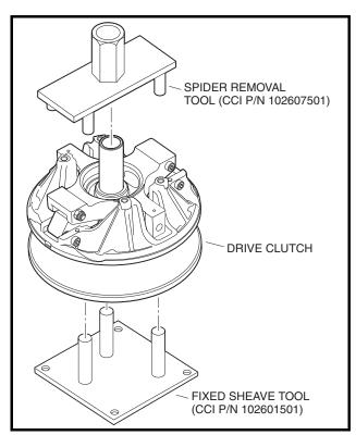
Figure 13a-29 Drive Clutch Service Tools
