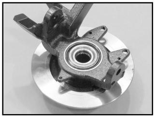
Figure 6-15 Upright, Bearing and Shaft Assembly
