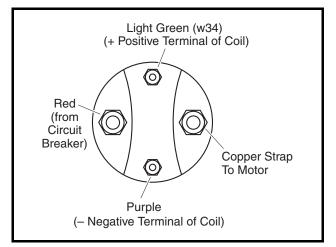
Figure 16-30 Solenoid Wiring and Testing
