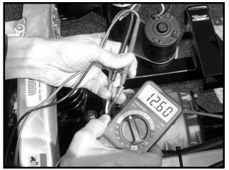
Figure 11a-38 Bed Lift Motor Voltage Reading with Switch in UP position
