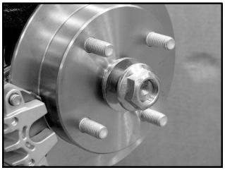
Figure 14-2 Axle Spindle Nut And Washer
