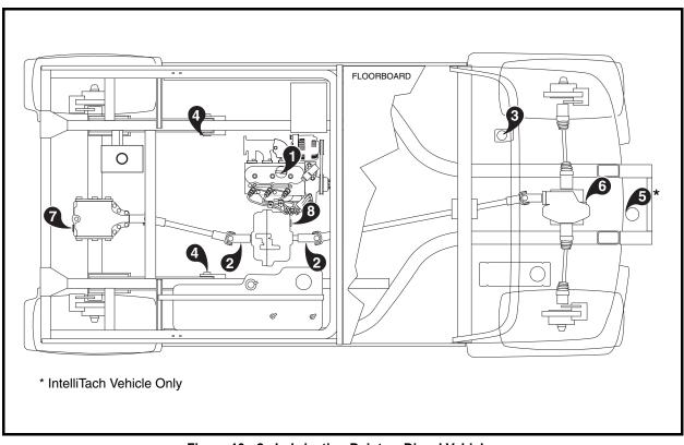
Figure 10a-2 Lubrication Points – Diesel Vehicles
