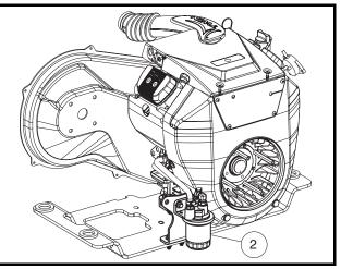
Figure 10b-9 Replace Engine Oil Filter – Kawasaki Powered Gasoline Vehicles
