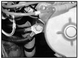
Figure 11b-7 Engine Ground (Under Starter)
