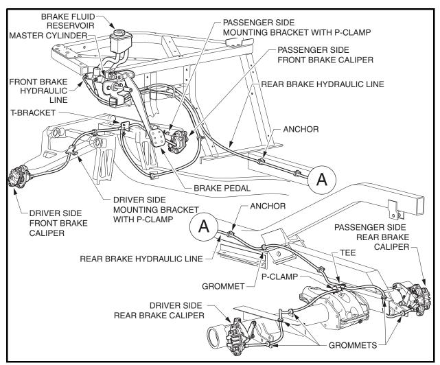
Figure 6-1 Hydraulic Disc Brake System
