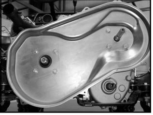
Figure 13b-36 Clutch Inner Cover
