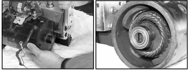
Figure 16-93 Remove Motor Bolts
