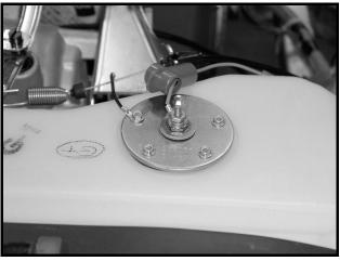
Figure 13a-10 Fuel Level Sensor
