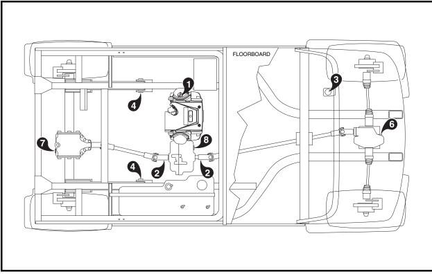
Figure 10b-1 Lubrication Points – Gasoline Vehicles
