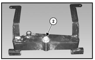
Figure 16-78 Apply LOCTITE and Install Angle Pivot Bushings
