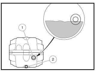
Figure 10b-18 Rear Differential Lubrication Level
