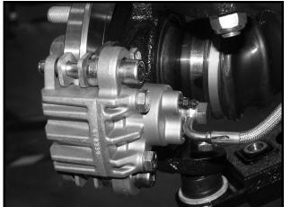
Figure 6-3 Front Brake Pad and Caliper
