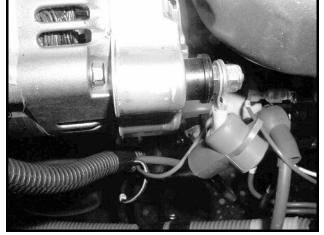
Figure 12c-12 12-Gauge Blue Fusible Link at Alternator (40 Amp Shown)
