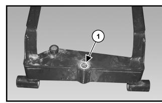
Figure 16-77 Remove Snow Blade Angle Pivot Bushings
