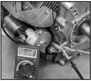
Figure 11b-21 Charge Coil Test (At Voltage Regulator Figure 11b-22 Charge Coil Test (At Bullet Connectors) Multi-Pin Connector)
