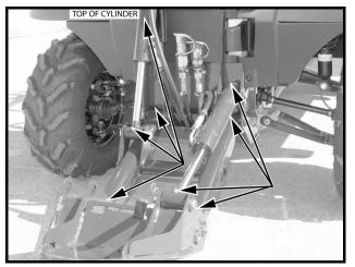
Figure 10b-3 Lubricate Grease Zerks located on Cylinder and Attachment Arm Ends
