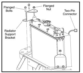
Figure 15-4 Radiator Bracket Attachment
