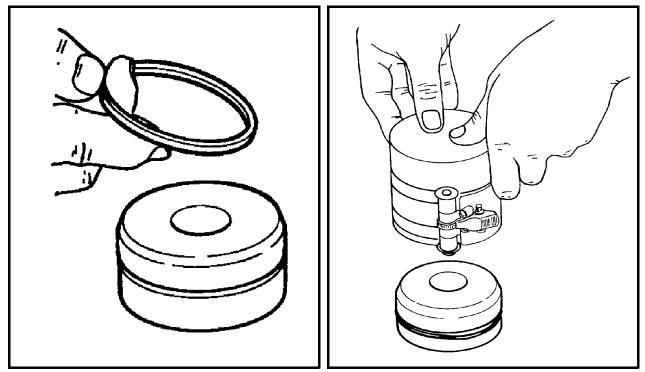
Figure 16-55 Install Piston Seal
