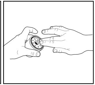
Figure 10a-12 Coat Rubber Seal
