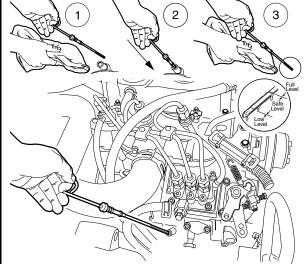
Figure 10b-7 Engine Oil Level Check – Diesel Vehicles
