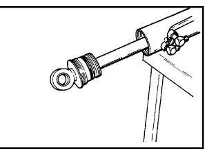
Figure 16-70 Install Rod Assembly
