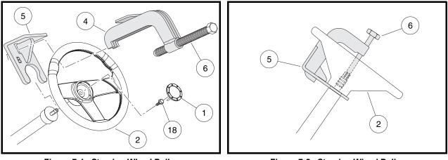
Figure 7-1 Steering Wheel Puller
