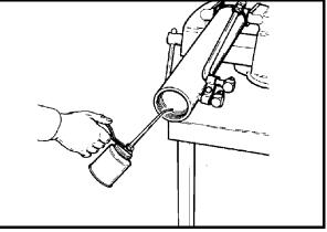
Figure 16-68 Lubricate Seal
