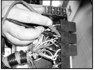
Figure 11c-18 Differential Relay Contact Test
