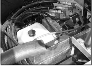
Figure 10a-21 Hydraulic Fluid Tank, Pump and Control Valves
