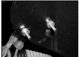
Figure 12b-7 Reverse Warning Buzzer Limit Switch Adjustment Slot
