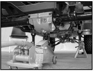
Figure 14-16 Position Floor Jack Under Differential
