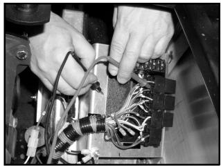
Figure 11c-15 Start Relay Coil Circuit Test
