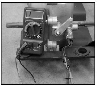
Figure 11c-33 Neutral Switch – Reverse Position
