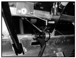
Figure 13a-21 High-speed RPM Adjustment Screw
