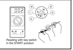
Figure 11b-8 Key Switch Test – Accessory Terminal
