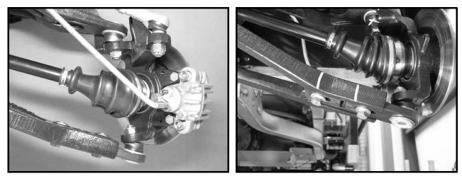
Figure 14-3 Front Caliper and Discs
