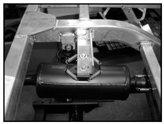
Figure 13a-4 Muffler Bracket and Inlet Pipe
