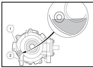
Figure 10b-16 Front Differential Lubrication Level
