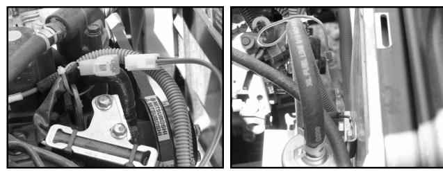
Figure 11c-29 Fuel Solenoid Three-Pin Connector
