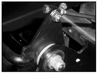
Figure 14-22 Forward/Reverse Shifter Cable Ball Socket At Shifter Handle Ball Stud
