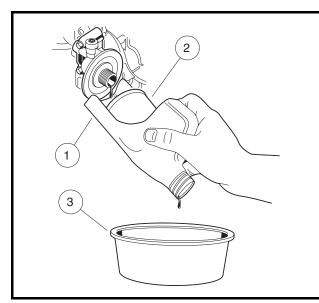
Figure 10a-11 Remove Engine Oil Filter
