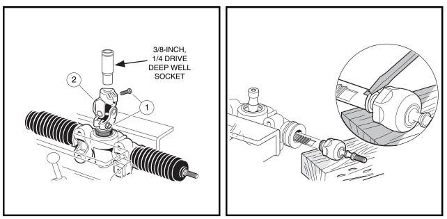
Figure 7-19 Adjust Rack and Pinion Resistance
