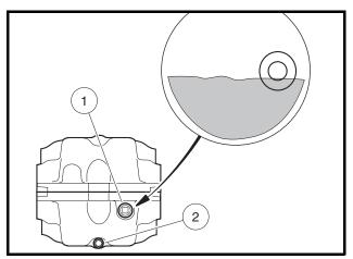
Figure 10a-19 Rear Differential Lubrication Level
