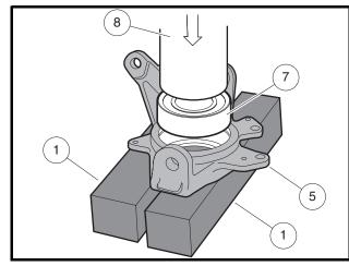
Figure 6-13 Position Upright for New Bearing
