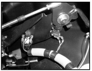
Figure 11b-25 Reverse Warning Buzzer and Limit Switch
