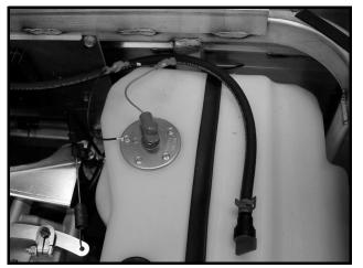
Figure 13b-7 Gasoline Fuel Tank
