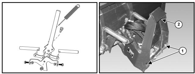
Figure 16-3 Hand Lever Linkages and Pins
