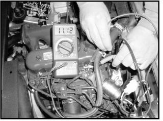
Figure 11c-37 Glow Plug Circuit Test
