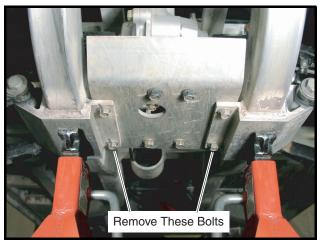
Figure 14-11 Front Differential Plate
