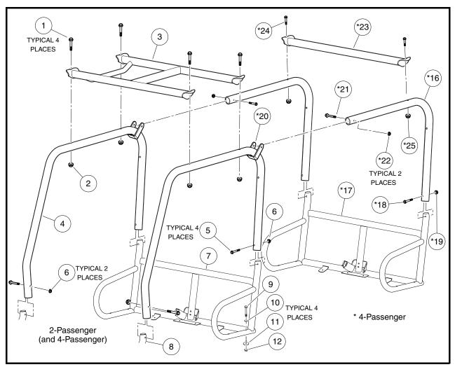
Figure 4-1 Roll-Over Protective Structure (ROPS)
