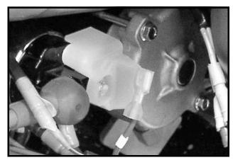
Figure 11b-10 Solenoid Coil Wire (w127) Removed
