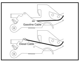
Figure 13c-17 Z-Shaped Cable End in Hole at Pedal
