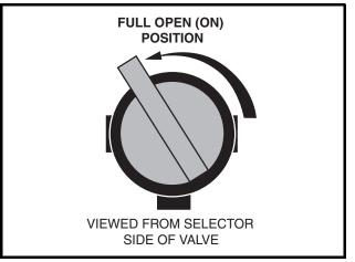
Figure 13b-10 Open Fuel Shut-Off Valve
