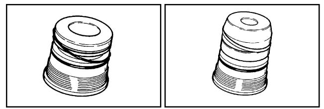
Figure 16-61 Install O-ring on Head
