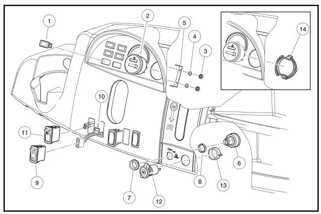
Figure 12c-6 Instrument Panel Electrical Components
