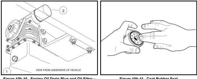
Figure 10b-10 Engine Oil Drain Plug and Oil Filter – Diesel Vehicles
