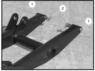
Figure 16-11 Attachment Arm Pins and Retaining Rings
