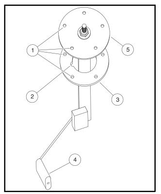
Figure 13c-11 Fuel Level Sending Unit Alignment
