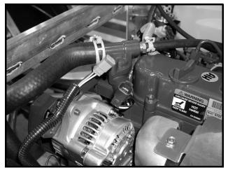
Figure 11c-24 Thermostat Switch Connector
