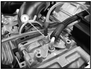
Figure 12a-4 Carburetor Heater
