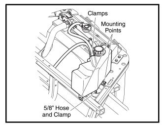
Figure 15-3 Reservoir Hoses And Mounting Points
