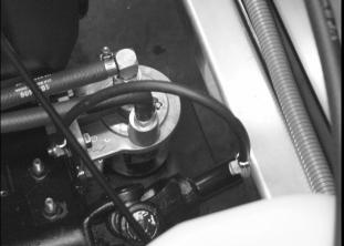
Figure 11a-7 Engine Ground to Frame
