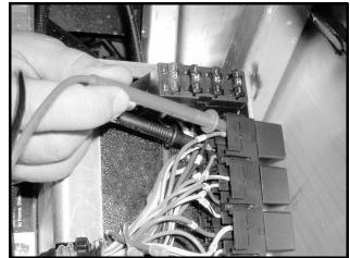
Figure 11c-16 Start Relay Contact Test
