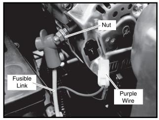
Figure 12c-11 18-Gauge Purple Wire and 12-Gauge Blue Fusible Link at Alternator (60 Amp Shown)
