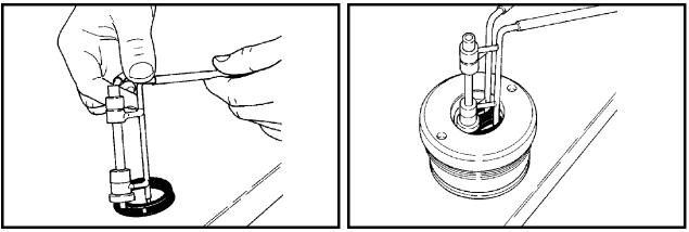
Figure 16-57 Rod Seal Tool
