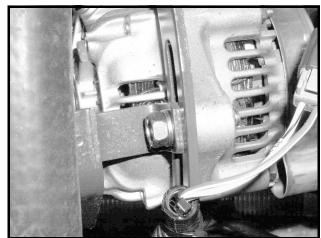
Figure 12c-13 Belt Tension Adjustment Bolt
