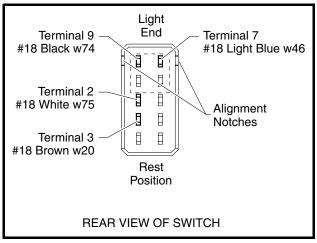
Figure 16-24 Float Switch Test
