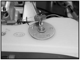
Figure 13c-14 Fuel Level Sensor
