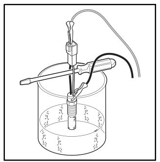
Figure 11c-22 Fan Thermostat Switch Test Setup
