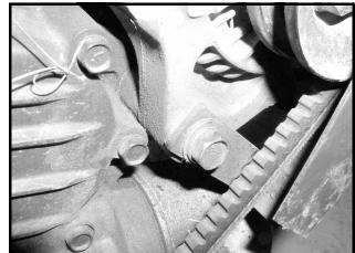
Figure 12c-14 Alternator Mounting Bolt
