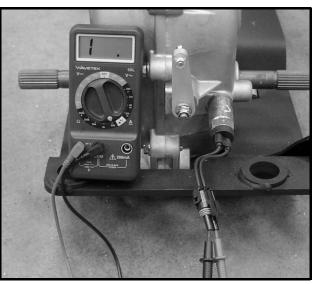
Figure 11a-18 Neutral Switch – Forward Position
