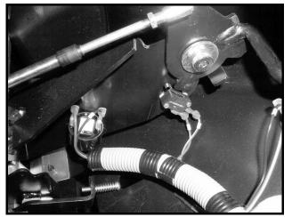
Figure 11a-26 Reverse Warning Buzzer and Limit Switch
