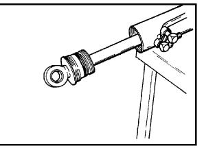
Figure 16-44 Remove Rod Assembly
