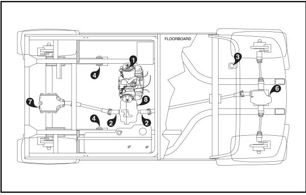
Figure 10a-1 Lubrication Points – Gasoline Vehicles
