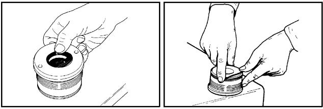
Figure 16-59 Install Wiper Seal
