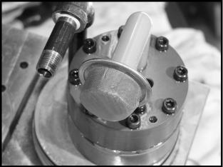
Figure 16-92 Suction Tube Filter
