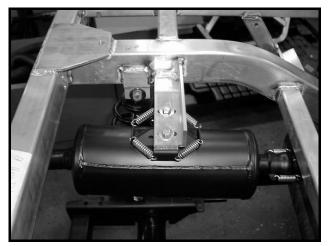
Figure 13c-5 Muffler Bracket and Inlet Pipe
