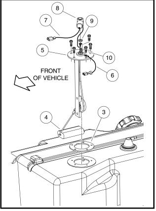
Figure 13c-10 Fuel Level Sending Unit Removal
