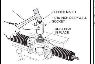
Figure 7-17 Press In Dust Seal
