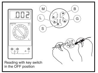
Figure 11b-24 Key Switch Test – Engine Kill Circuit
