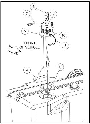
Figure 13b-4 Fuel Level Sending Unit Removal
