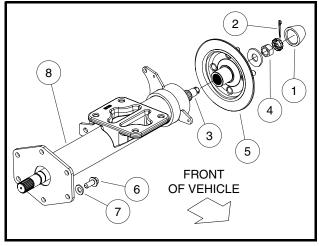
Figure 14-25 Axle Shaft and Brake Rotor
