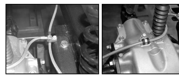
Figure 14-13 Receiver Hitch Brake Line T-Fitting and Bracket
