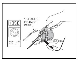
Figure 11b-28 Fuel Gauge Voltage Test - Terminal 2
