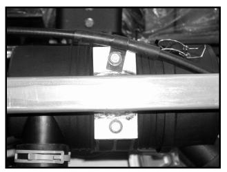
Figure 6-23 Air Filter and Park Brake Cable Clamp
