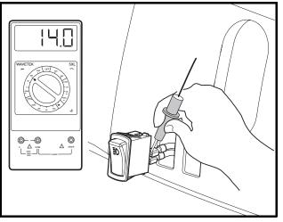
Figure 11c-46 Light Switch Test
