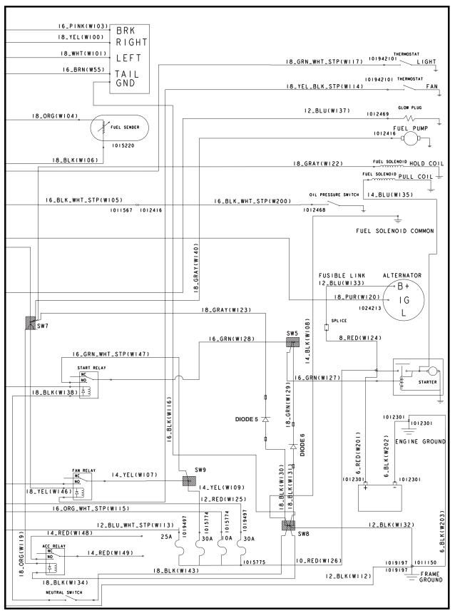
Figure 11c-4 Wiring Diagram (1 Piece Harness) for Diesel Carryall 295 and XRT 1550 Vehicles (Rear)
