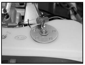
Figure 13b-8 Fuel Level Sensor
