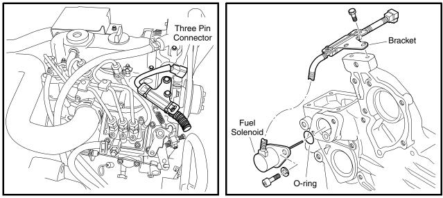
Figure 12c-3 Fuel Solenoid Three-Pin Connector
