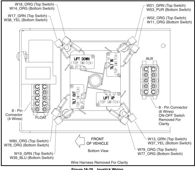
Figure 16-20 Joystick Wiring
