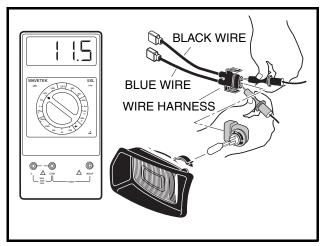
Figure 11c-47 Voltage At Headlight Socket
