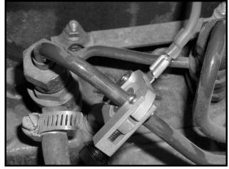
Figure 13c-20 Diesel Probe Fuel Line Clamp On Engine
