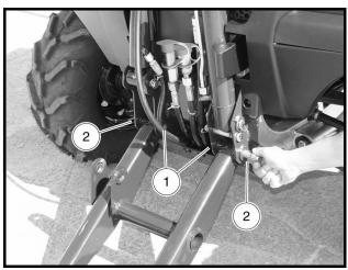
Figure 16-13 Align the Attachment Arm Holes
