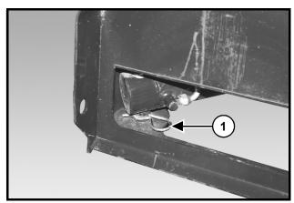
Figure 16-40 Remove Retaining Pin
