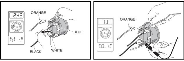
Figure 11a-31 Fuel Gauge Voltage Test - Terminal 2
