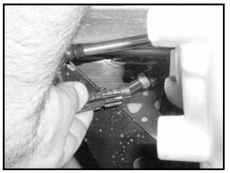
Figure 11c-26 Neutral Switch Two-Pin Connector
