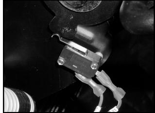
Figure 12b-8 Reverse Warning Buzzer Limit Switch (Properly Adjusted)
