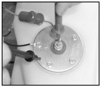
Figure 11b-27 Fuel Level Sending Unit Test
