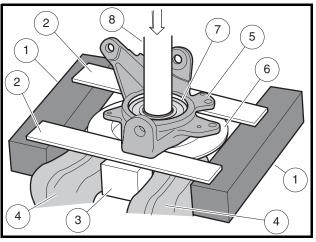
Figure 6-11 Position Steel Blocks and Upright on Press
