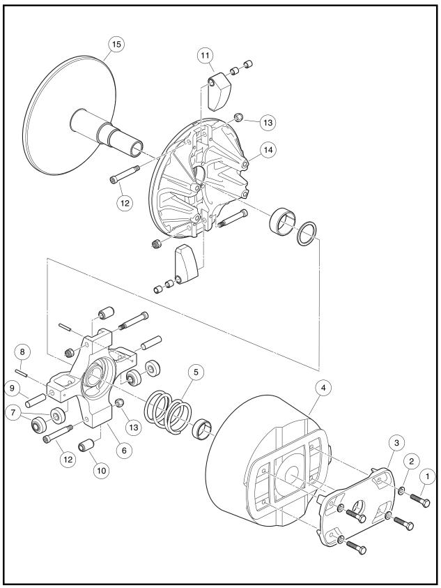
Figure 13b-33 Drive Clutch Assembly
