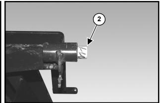
Figure 16-80 Apply LOCTITE and Install Four Pivot Bushings
