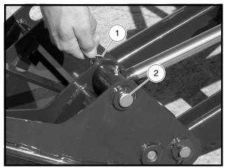
Figure 16-17 Raise Interface, Install Pin and Retainer Ring
