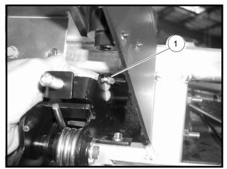
Figure 13a-14 Z-Shaped Cable End (Gasoline Vehicles)
