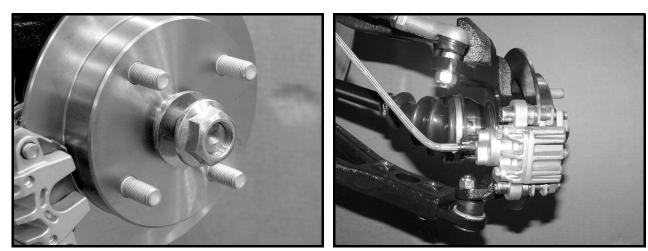
Figure 6-7 Axle Spindle Nut and Washer
