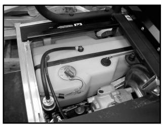
Figure 13c-13 Diesel Fuel Tank
