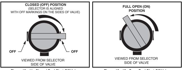
Figure 13a-11 Closed Fuel Shut-Off Valve
