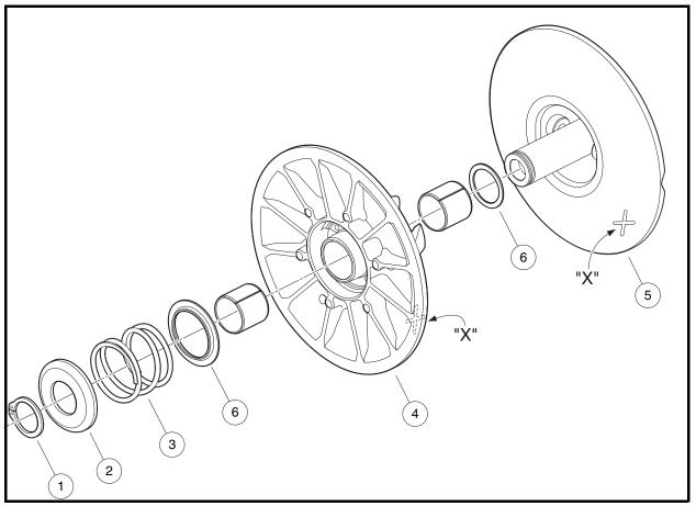
Figure 13b-35 Driven Clutch Assembly
