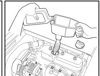
Figure 10b-13 Add Engine Oil – Diesel Vehicles
