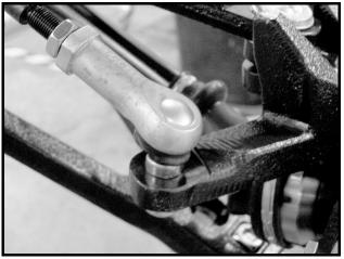
Figure 7-26 Drag Link Ball Joint
