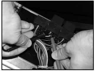
Figure 11a-13 Carburetor Heater Relay Coil Circuit Test
