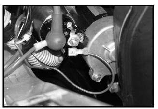
Figure 11a-10 Solenoid Coil Wire (w127) Removed
