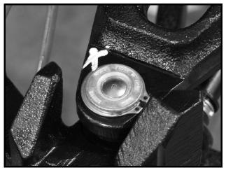
Figure 7-31 Ball Joint C-Clip
