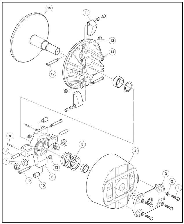
Figure 13c-32 Drive Clutch Assembly
