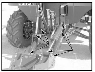
Figure 10a-3 Lubricate Grease Zerks located on Cylinder and Attachment Arm Ends
