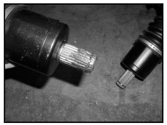
Figure 14-7 Apply Anti-Seize to Splined Ends
