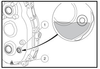
Figure 10b-17 Transmission Lubrication Level
