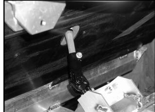
Figure 7-4 Steering Universal Joint
