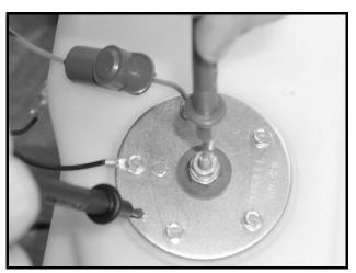
Figure 11a-28 Fuel Level Sending Unit Test
