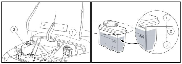
Figure 10b-4 Brake Fluid and Engine Coolant Access
