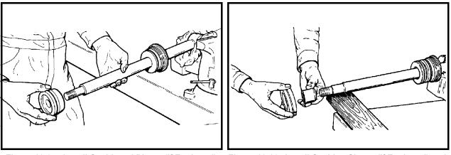
Figure 16-65 Install Cushioned Piston (If Equipped)
