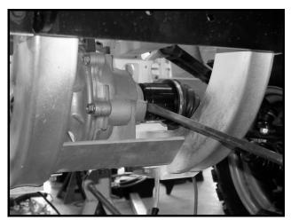
Figure 14-5 Separate Half Shaft from Differential
