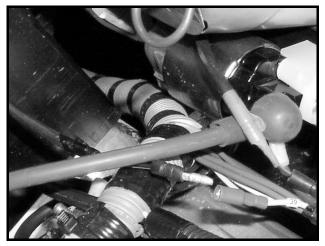
Figure 12b-3 Carburetor Coil Bullet Connector
