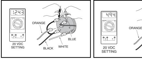
Figure 11c-44 Fuel Gauge Voltage Test - Terminal 2
