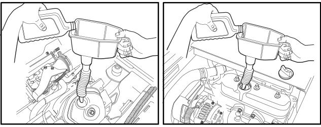
Figure 10a-13 Add Engine Oil – Gasoline Vehicles
