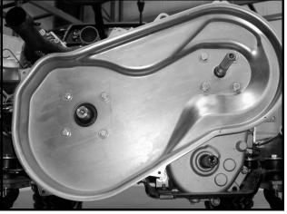
Figure 13a-33 Clutch Inner Cover
