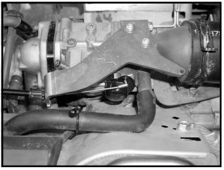
Figure 13b-25 Choke Cable on Engine
