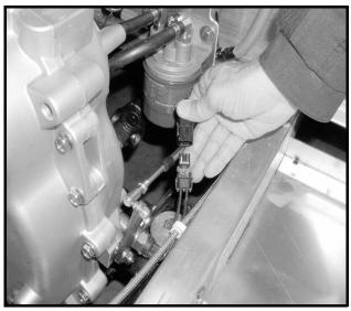
Figure 11a-17 Neutral Switch Two-Pin Connector
