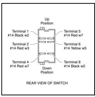
Figure 11a-40 Bed Lift Switch Terminals
