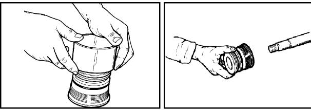
Figure 16-63 Compress Seal
