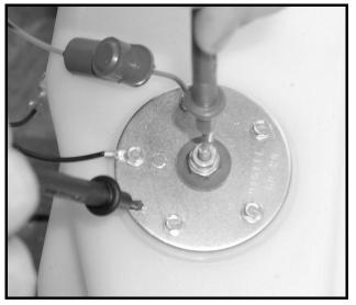
Figure 11c-39 Fuel Level Sending Unit Test
