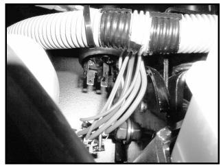
Figure 11c-27 Disconnected Multi-Pin Connector at Key Switch
