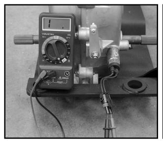
Figure 11b-18 Neutral Switch – Forward Position
