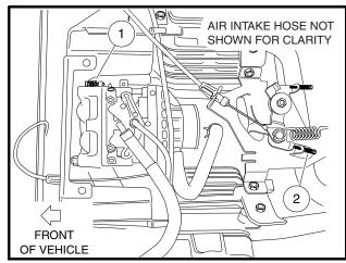
Figure 13a-20 Idle RPM Adjustment Screws
