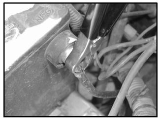
Figure 13c-21 Diesel Probe Battery Cable Clamp
