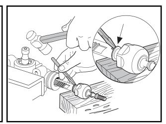
Figure 7-15 Remove Inner Ball Joints
