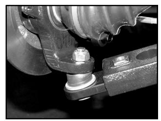
Figure 6-9 Lower Ball Joint and Upright
