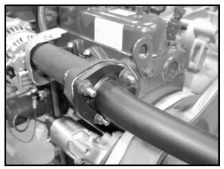
Figure 13c-6 Diesel Manifold Pipe Flange
