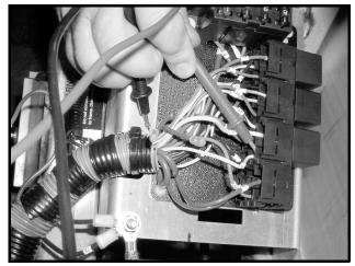
Figure 11c-19 Check Power To Fan Relay
