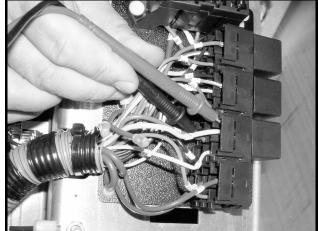
Figure 11c-20 Fan Relay Contact Test
