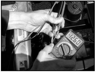
Figure 11a-39 Bed Lift Motor Voltage Reading with Switch in DOWN position
