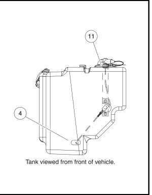
Figure 13b-6 Fuel Level Sending Unit Position
