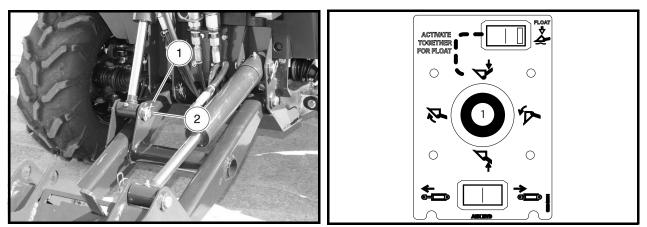
Figure 16-7 Remove Attachment Cylinder Retaining Pin
