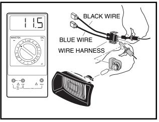
Figure 11b-31 Voltage Measurement at Headlight Socket
