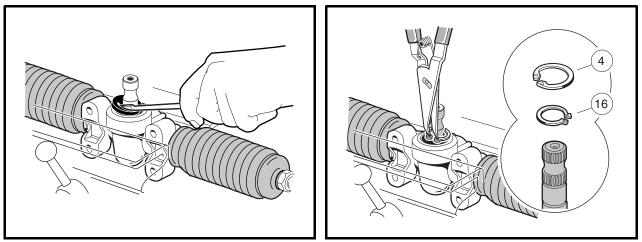
Figure 7-10 Remove Dust Seal
