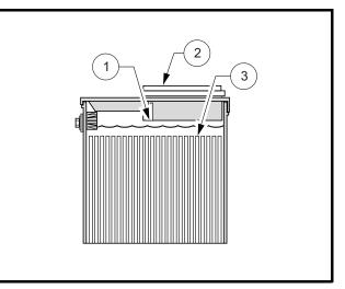
Figure 11a-4 Battery Electrolyte Level 1. Level Indicator 2. Cap 3. Plates Electrolyte level at least 1/2 inch (13 MM) above plates or to level indicator.
