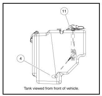
Figure 13c-12 Fuel Level Sending Unit Position
