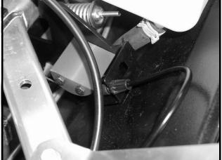
Figure 13c-16 Accelerator Cable Pedal Bracket (Diesel Vehicles)
