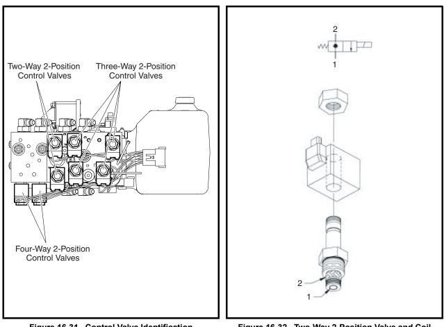
Figure 16-31 Control Valve Identification
