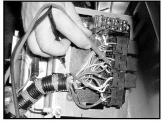
Figure 11c-17 Differential Relay Coil Circuit Test
