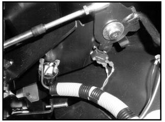
Figure 12a-7 Reverse Warning Buzzer and Limit Switch
