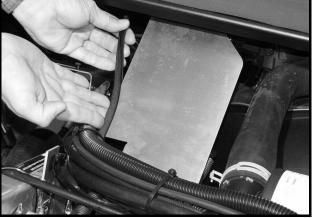
Figure 16-88 Cover Edge of Heat Shield
