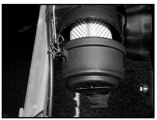
Figure 13a-22 Air Filter Cartridge
