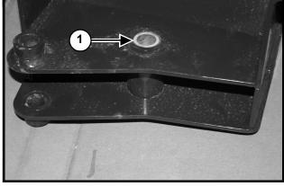
Figure 16-81 Remove Whisk Broom Pivot Bushings
