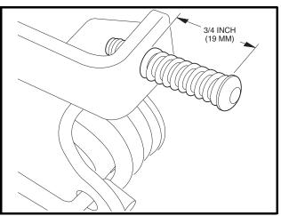
Figure 5-3 Ground Speed Set Screw Adjustment
