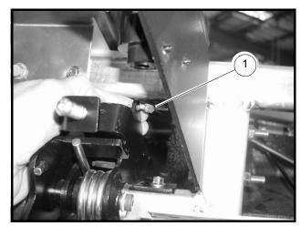
Figure 13c-15 Z-Shaped Cable End
