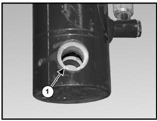
Figure 16-73 Remove Bushings From Base
