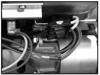
Figure 11a-22 Charge Coil Test (At Voltage Regulator Multi-Pin Connector)
