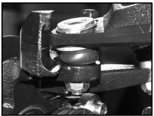
Figure 6-10 Upper Ball Joint and Upright
