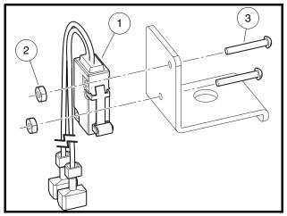
Figure 12a-10 Front Differential Limit Switch Removal
