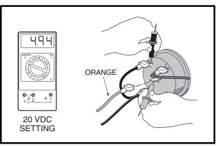
Figure 11a-33 Fuel Gauge Voltage Test - Terminal 2
