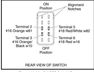
Figure 16-23 ON/OFF Switch Test
