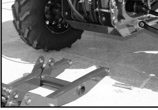
Figure 16-12 Align the Vehicle to Attachment Arms
