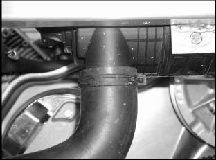
Figure 13a-26 Air Filter Inlet Hose
