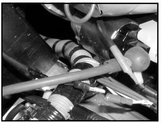
Figure 11b-16 Carburetor Coil Bullet Connector
