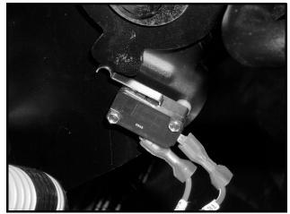
Figure 12c-8 Reverse Warning Buzzer Limit Switch Adjustment Slot
