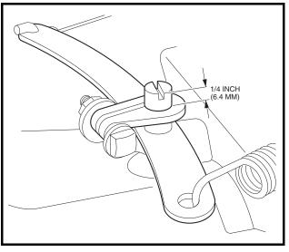
Figure 13b-22 Pin Measurement at (Transmission) Governor Arm
