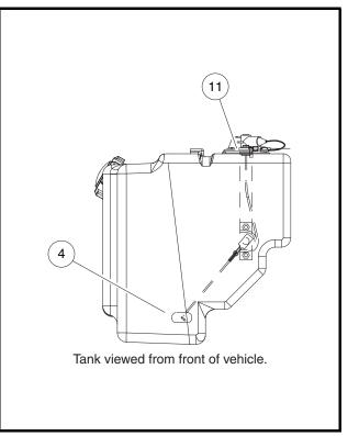
Figure 13a-8 Fuel Level Sending Unit Position
