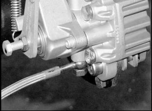
Figure 6-6 Rear Brake Line and Banjo Bolt
