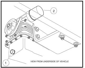
Figure 10a-10 Engine Oil Drain Plug and Oil Filter – Diesel Vehicles
