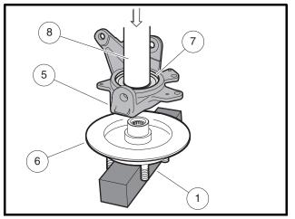
Figure 6-14 Press Disc and Hub into Bearing
