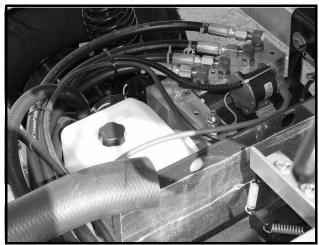
Figure 10b-20 Hydraulic Fluid Tank, Pump and Control Valves
