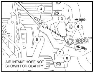
Figure 13a-16 Accelerator Cable at Engine
