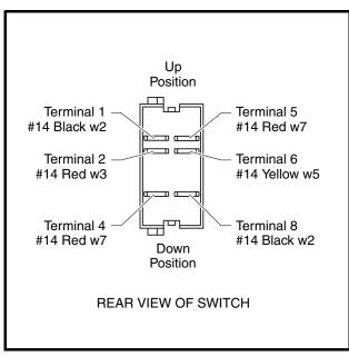
Figure 11b-35 Bed Lift Switch Terminals
