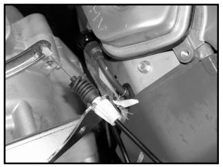
Figure 13b-18 Governor Cable on Transmission
