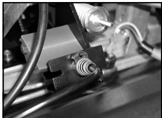
Figure 13b-13 Accelerator Cable Pedal Bracket (Gasoline Vehicles)
