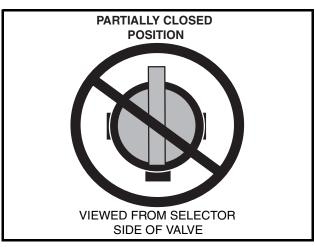
Figure 13b-11 Incorrect Fuel Shut-Off Valve
