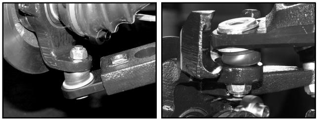
Figure 7-27 Lower Ball Joint
