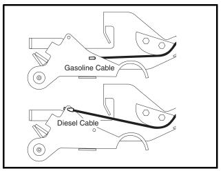
Figure 13b-15 Z-Shaped Cable End in Hole at Pedal
