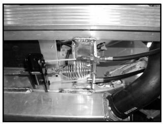
Figure 6-22 Park Brake Frame Bracket
