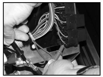
Figure 11a-11 Start Relay Coil Circuit Test
