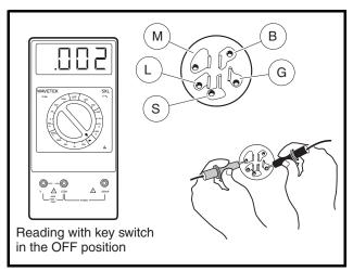
Figure 11a-25 Key Switch Test – Engine Kill Circuit
