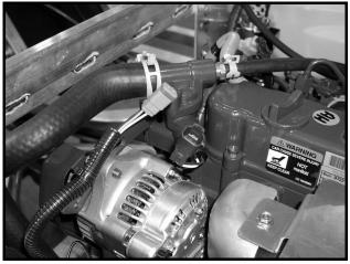
Figure 12c-16 Thermostat Switch
