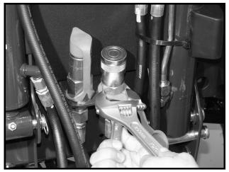
Figure 16-36 Quick Connect Fitting Removal
