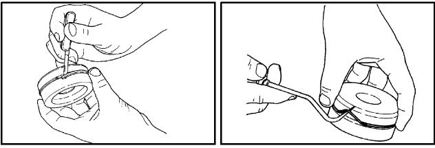
Figure 16-51 Remove Piston Seal
