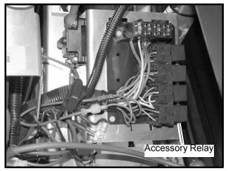
Figure 16-28 Accessory Relay Location
