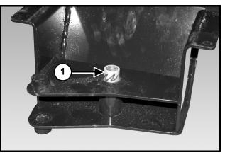
Figure 16-82 Apply LOCTITE and Install Pivot Bushings
