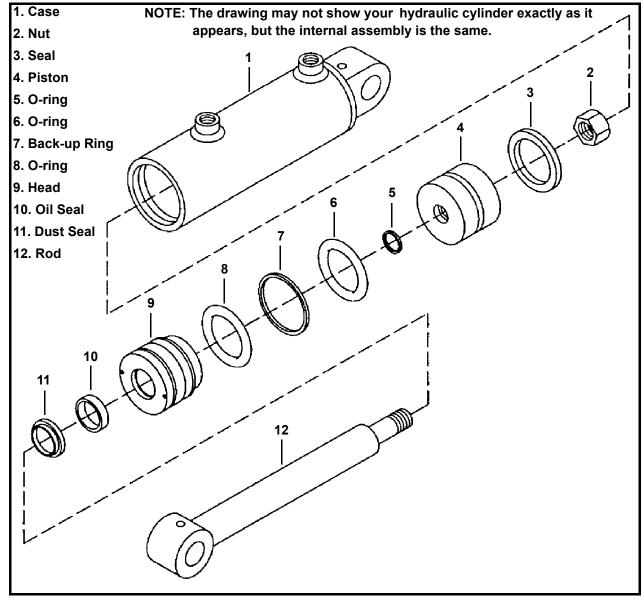
Figure 16-42 Cylinder Exploded View
