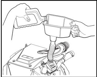
Figure 10b-12 Add Engine Oil – Kawasaki Powered Gasoline Vehicles
