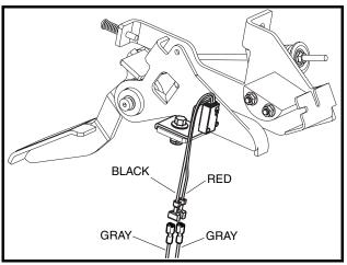
Figure 11a-21 Front Differential Switch
