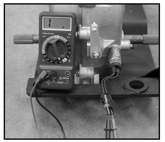
Figure 11c-31 Neutral Switch – Forward Position
