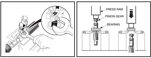
Figure 7-12 Remove Pinion from Housing
