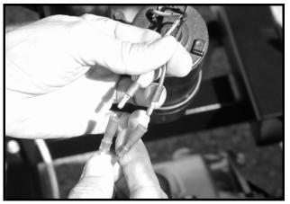
Figure 11b-32 Bed Lift Motor Wires
