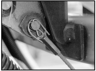
Figure 6-25 Park Brake Cable Attachment
