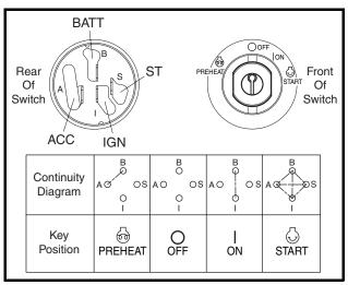
Figure 11c-12 Key Switch Terminals and Continuity Diagram
