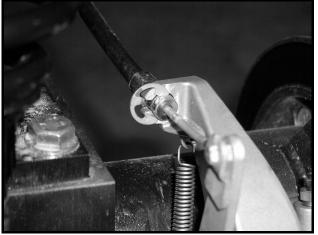
Figure 6-21 Park Brake Cable Attachment
