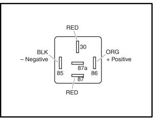
Figure 16-29 Accessory Relay Wiring and Testing
