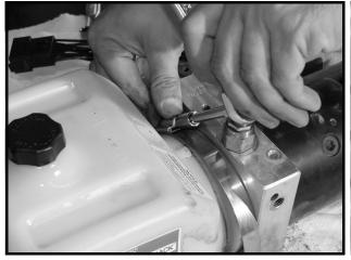
Figure 16-91 Loosen Band Clamp
