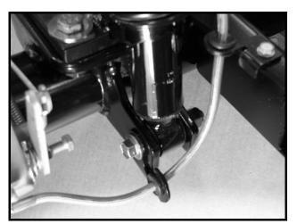
Figure 14-17 Lower Driver Side Shock Mount
