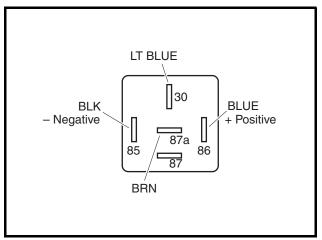
Figure 16-27 Relay 2 Wiring and Testing
