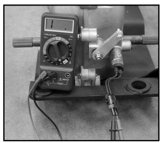
Figure 11b-20 Neutral Switch – Reverse Position
