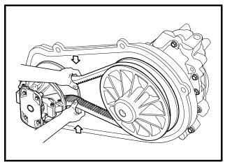
Figure 13c-30 Drive Belt Removal
