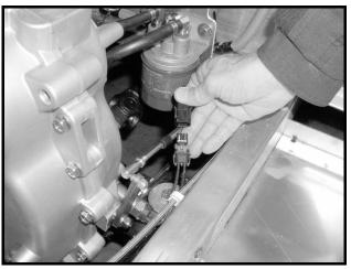
Figure 11b-17 Neutral Switch Two-Pin Connector
