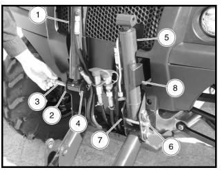
Figure 16-14 Remove Retainer Pins from Both Cylinders
