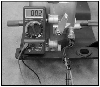
Figure 11c-32 Neutral Switch – Neutral Position
