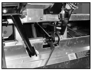
Figure 5-2 Accelerator Pedal Assembly
