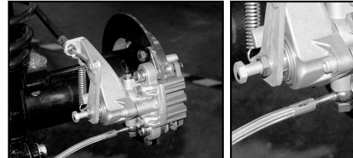
Figure 6-5 Rear Brake Pad and Caliper
