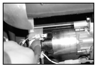
Figure 11c-13 Solenoid Coil Wire (w127) Removed
