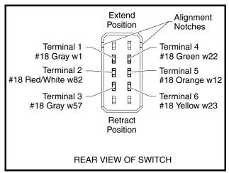
Figure 16-25 Auxiliary Hydraulic Switch Test
