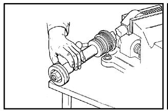
Figure 16-67 Install and Tighten Piston Nut
