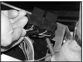
Figure 11a-12 Start Relay Contact Test
