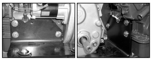
Figure 13c-3 Driver Side Diesel Engine Mount
