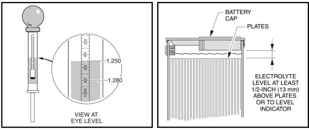
Figure 11b-3 Hydrometer Test
