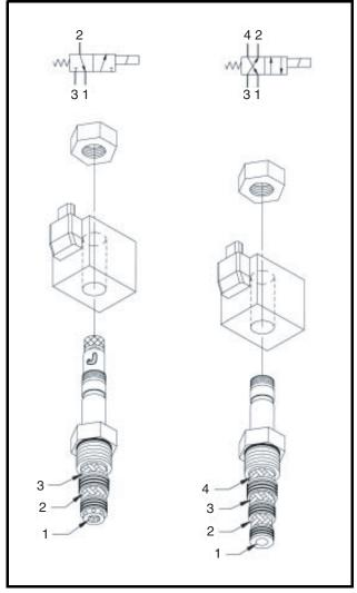
Figure 16-33 Three-Way 2-Position and Four-Way 2-Position Valve and Coil
