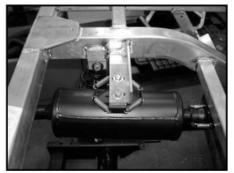
Figure 13b-2 Muffler Bracket and Inlet Pipe
