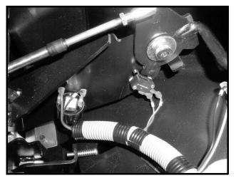
Figure 11c-38 Reverse Warning Buzzer and Limit Switch
