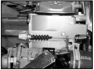
Figure 13b-19 Governor Cable on Engine
