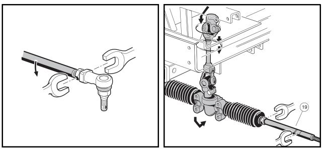
Figure 7-7 Drag Link Ball Joint
