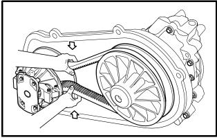
Figure 13b-31 Drive Belt Removal
