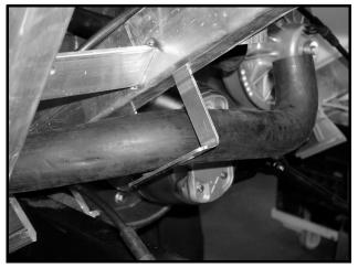
Figure 13c-26 Air Intake Support Bracket
