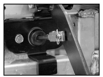
Figure 6-20 Master Cylinder Rod and Brake Pedal
