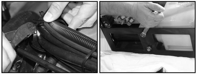
Figure 16-89 Wire Tie to Chassis
