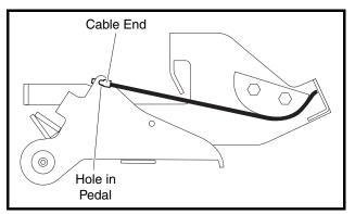
Figure 13a-17 Z-Shaped Cable End in Hole at Pedal
