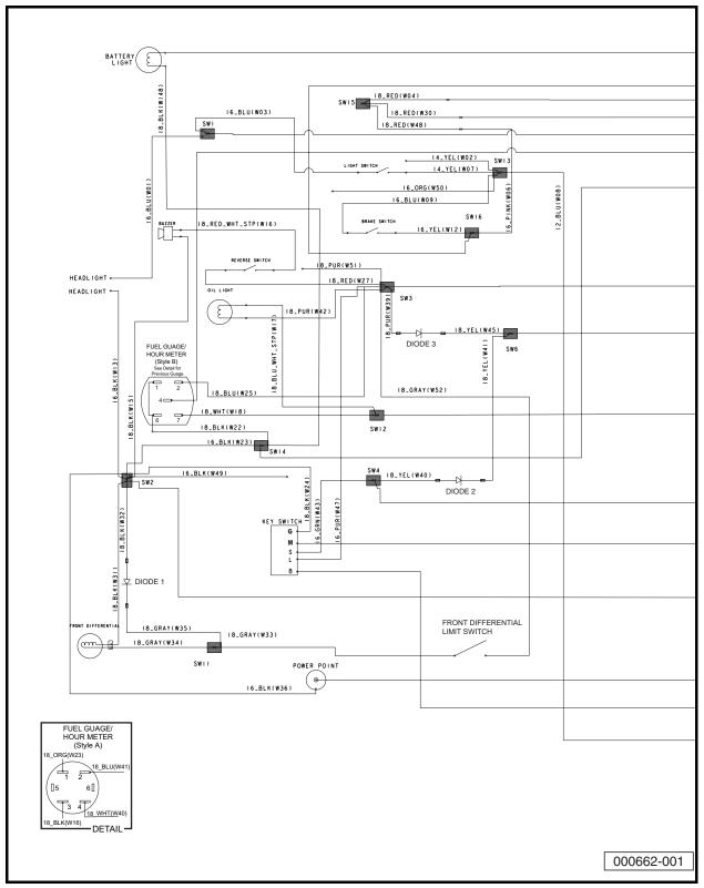
Figure 11a-1 Wiring Diagram – Kawasaki Powered Gasoline Carryall 295 and XRT 1550 Vehicles (Front)
