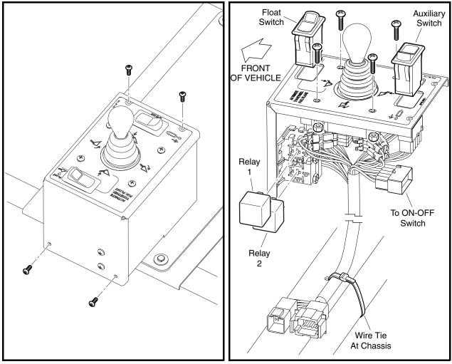
Figure 16-21 Joystick Hardware
