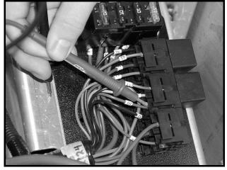
Figure 11b-14 Differential Relay Coil Circuit Test
