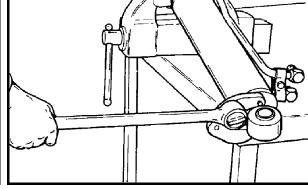
Figure 16-72 Tighten Head Against Case
