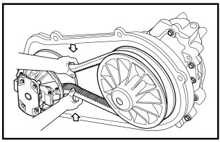
Figure 13a-28 Drive Belt Removal
