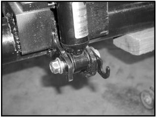
Figure 9-2 Remove Lower Driver-Side Shock Bolt
