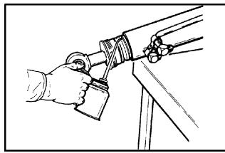
Figure 16-71 Lubricate Head Seals
