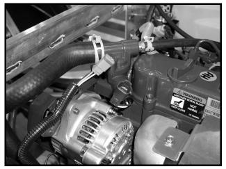
Figure 11c-36 Thermostat Switch Connector
