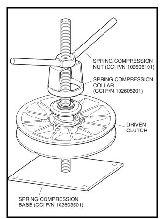
Figure 13b-34 Driven Clutch Service Tools
