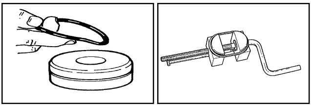
Figure 16-53 Install Piston O-ring
