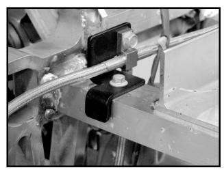
Figure 6-18 Front Brake Line T-Bracket
