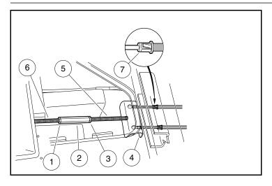
Figure 6-20 Loosen Brake Cables
