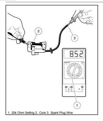
475 Figure 11-34 Secondary Coil Resistance – Bench Test
