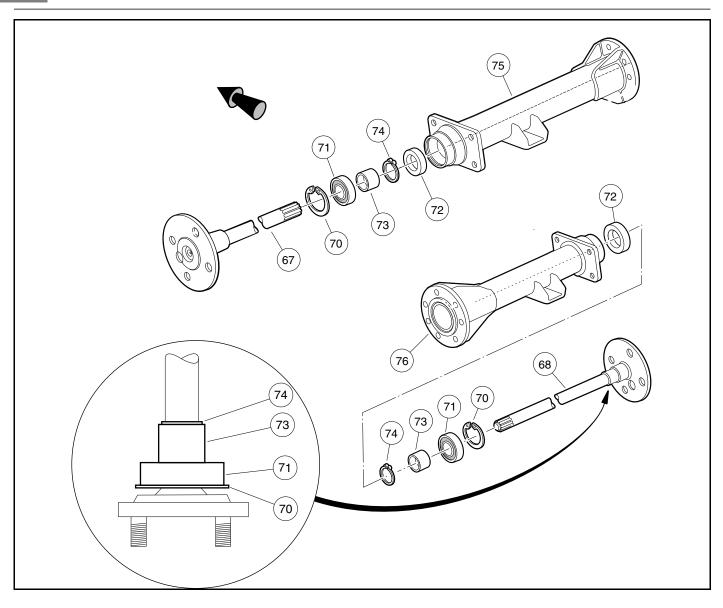
Figure 18-8 Differential Gear Case and Axle Tubes
