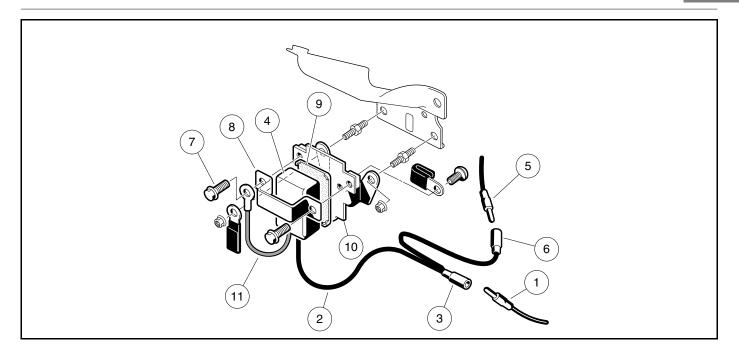
Figure 13-38 RPM Limiter Assembly
