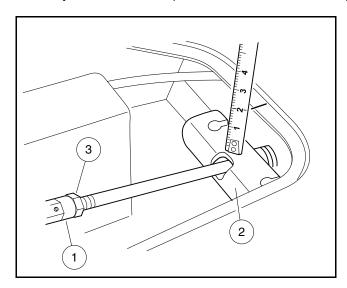
Figure 6-18 Equalizer Adjustment
