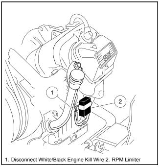
Figure 11-22 Disconnect White/Black Engine Kill Wire
