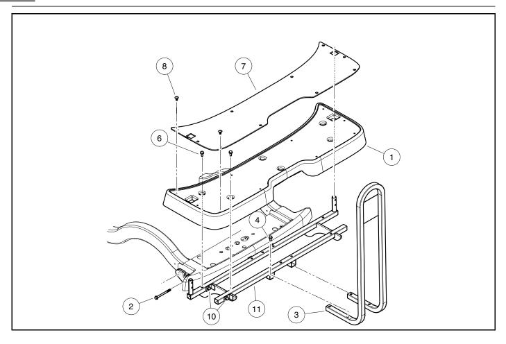
Figure 4-11 Foot Deck (Four-Passenger Vehicles)
