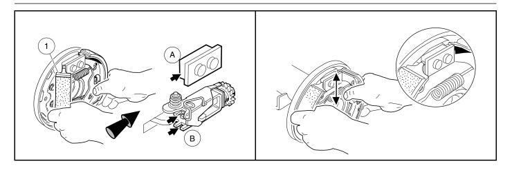
Figure 6-15 Install Leading Shoe
