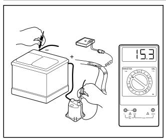
Figure 11-21 Voltage Regulator Test
