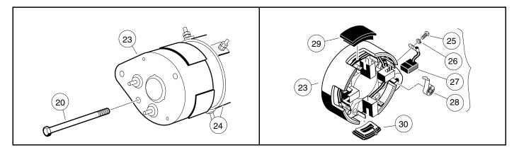
Figure 13-2 Commutator End Cover
