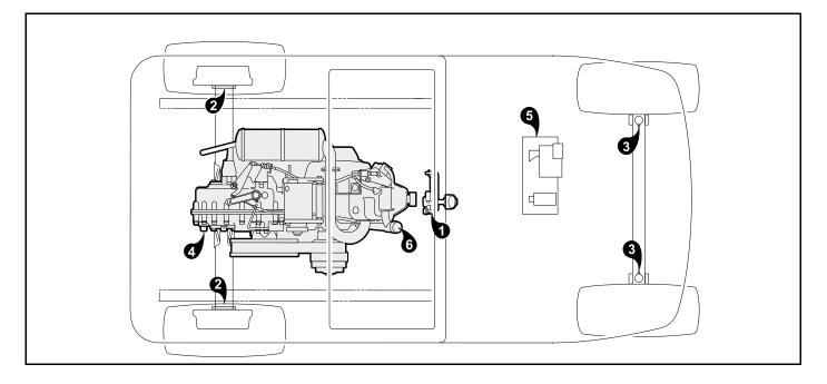
Figure 10-1 Lubrication Points – Gasoline Vehicles
