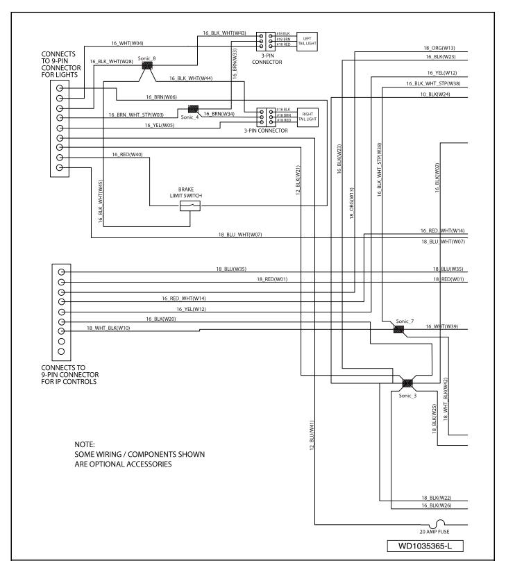
Figure 12-1 Wiring Diagram - Precedent Gasoline Vehicle with TPS
