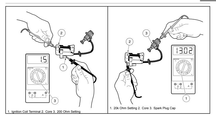
Figure 12-31 Primary Coil Resistance – Bench Test
