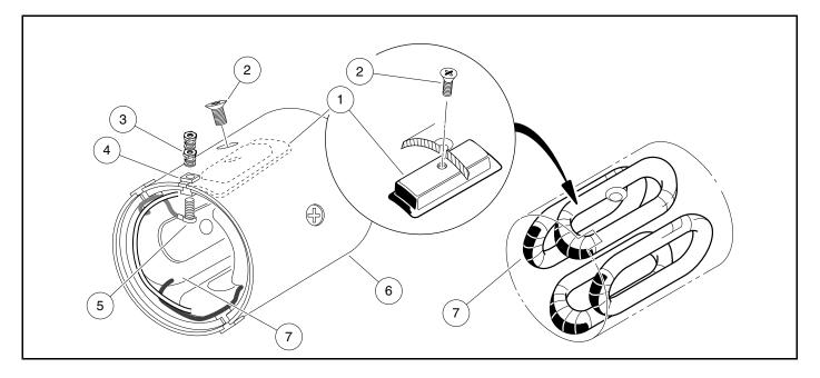
Figure 13-10 Field Coil Assembly
