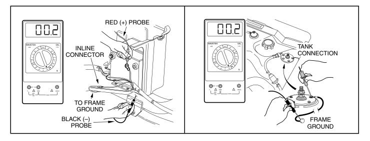
2420 Figure 12-11 Battery Ground Cable Test
