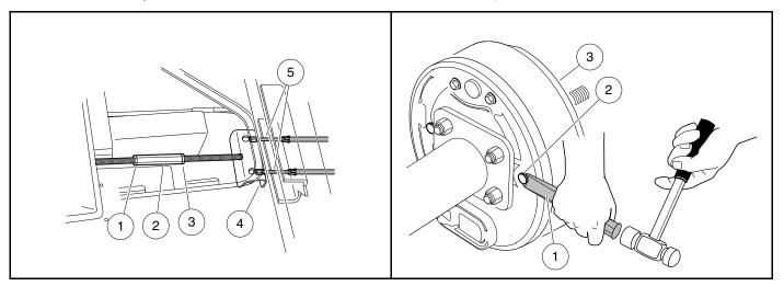
Figure 6-1 Loosen Turnbuckle
