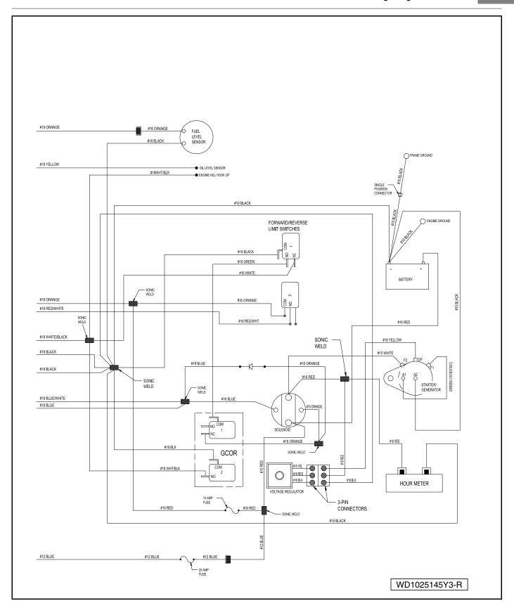
Figure 11-2 Wiring Diagram – Precedent Gasoline Vehicle with GCOR
