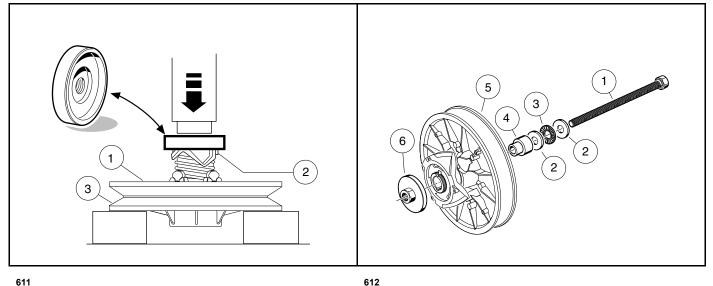
Figure 19-22 Cam Press Tool
