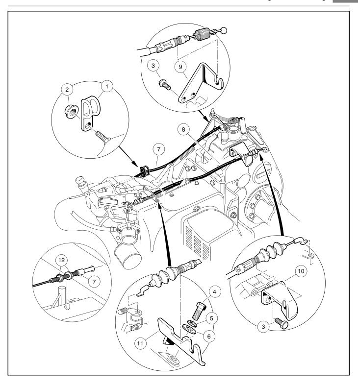
Figure 16-6 Governor and Accelerator Cables
