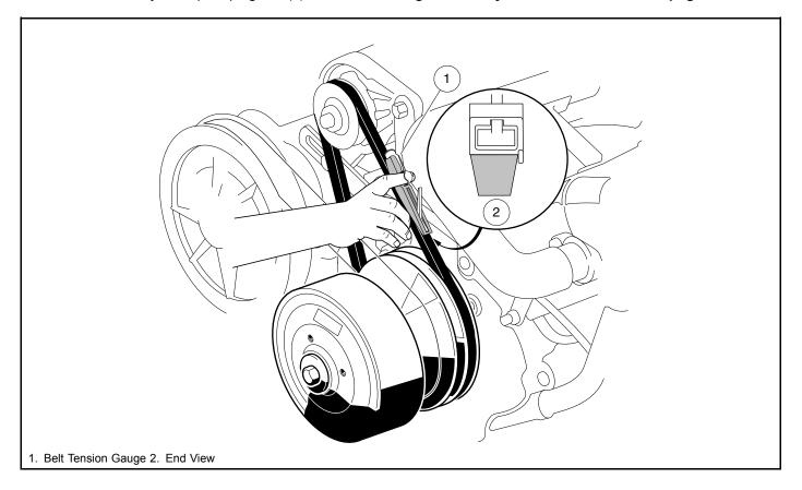
Figure 13-14 Belt Tension Gauge
