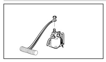
Figure 11-15 Solenoid Wire Removal
