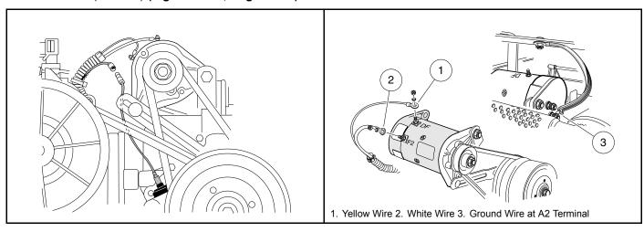
Figure 18-45 Oil Level Sensor Jumper wire
