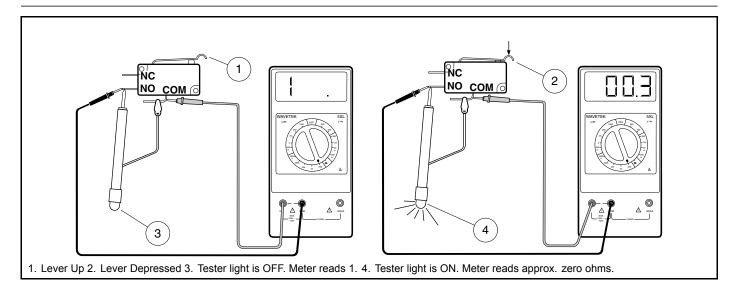
Figure 12-17 Test Neutral Lockout Switch
