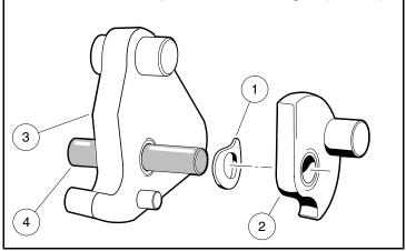
Figure 19-12 Primary and Secondary Weights, Wave Washer and Pin
