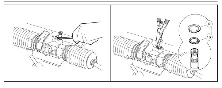
Figure 7-6 Remove Dust Seal
