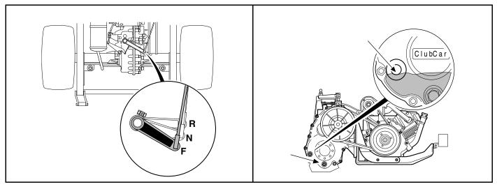
Figure 18-3 Shifter Positions (Top View)
