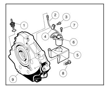
Figure 15-7 Oil Level Sensor
