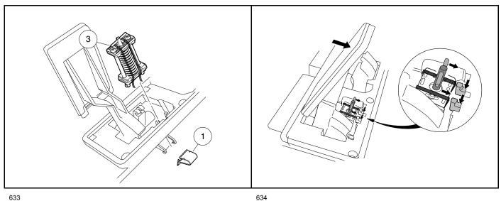
Figure 5-5 Accelerator Spring Clip
