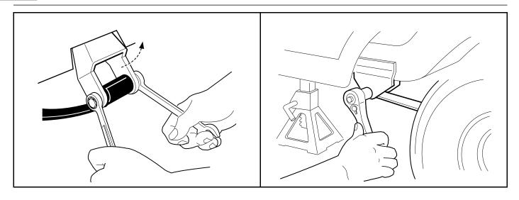
768 2401 Figure 18-24 Rear Shackles Figure 18-25 Spring Retainer Bolts
