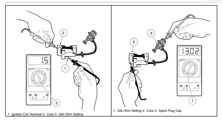
Figure 11-32 Primary Coil Resistance – Bench Test
