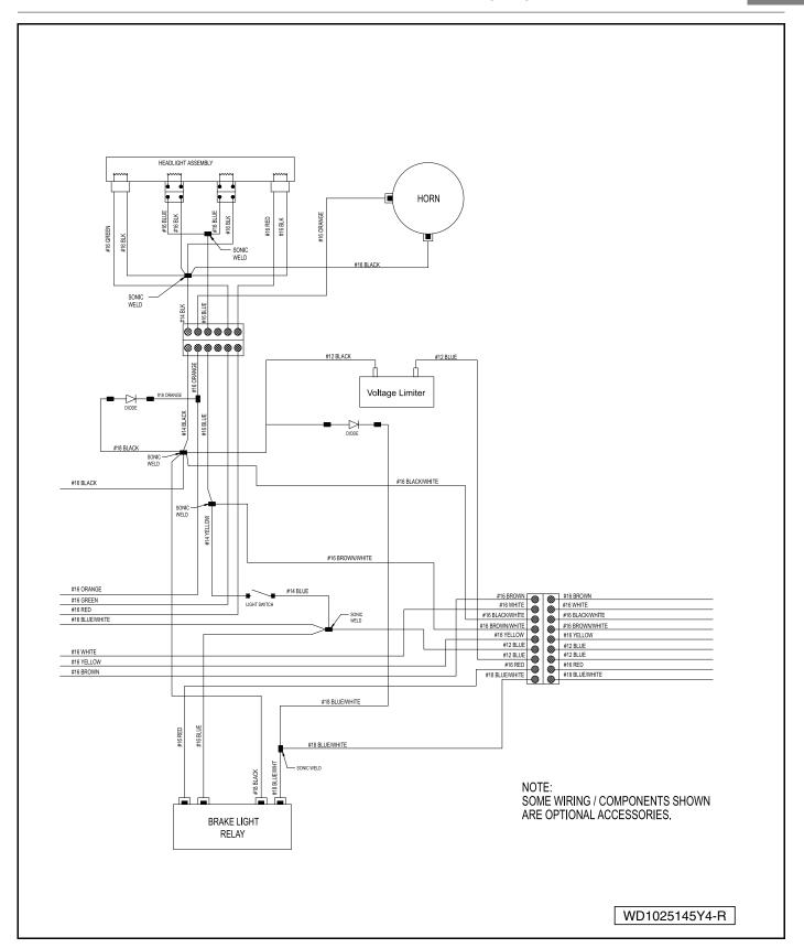
Figure 12-4 Precedent Gasoline Vehicle Accessory Wiring Diagram (Optional)
