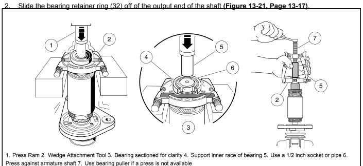
Figure 13-23 Bearing Removal
