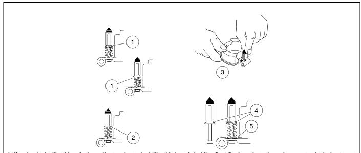
1. If spring looks like this... 2. then adjust spring to look like this by... 3. holding float firmly and rotating valve counterclockwise to seat spring in seat of float bowl 4. Check for coil located in groove above both ears. 5. Check for spring seated in recess of float.
