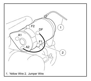
462 Figure 11-20 Jumper Wire Ground - DF to A2
