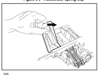
Figure 5-7 Accelerator Spring Pin Removal
