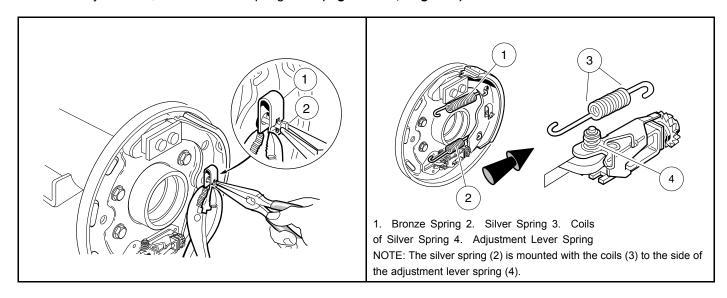
Figure 6-13 Install Trailing Shoe Retainer Clip
