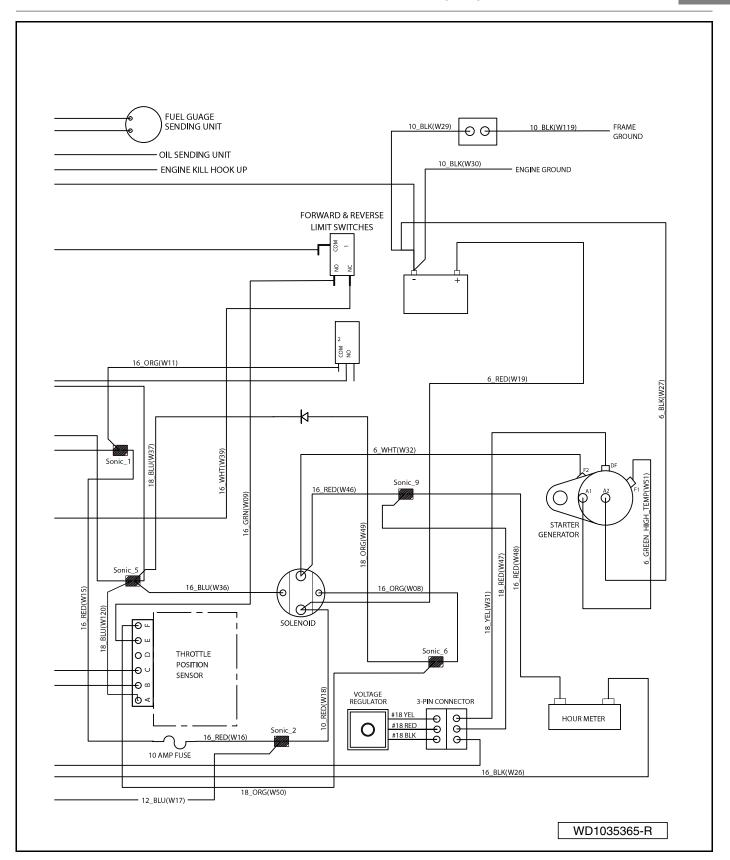
Figure 12-2 Wiring Diagram - Precedent Gasoline Vehicle with TPS
