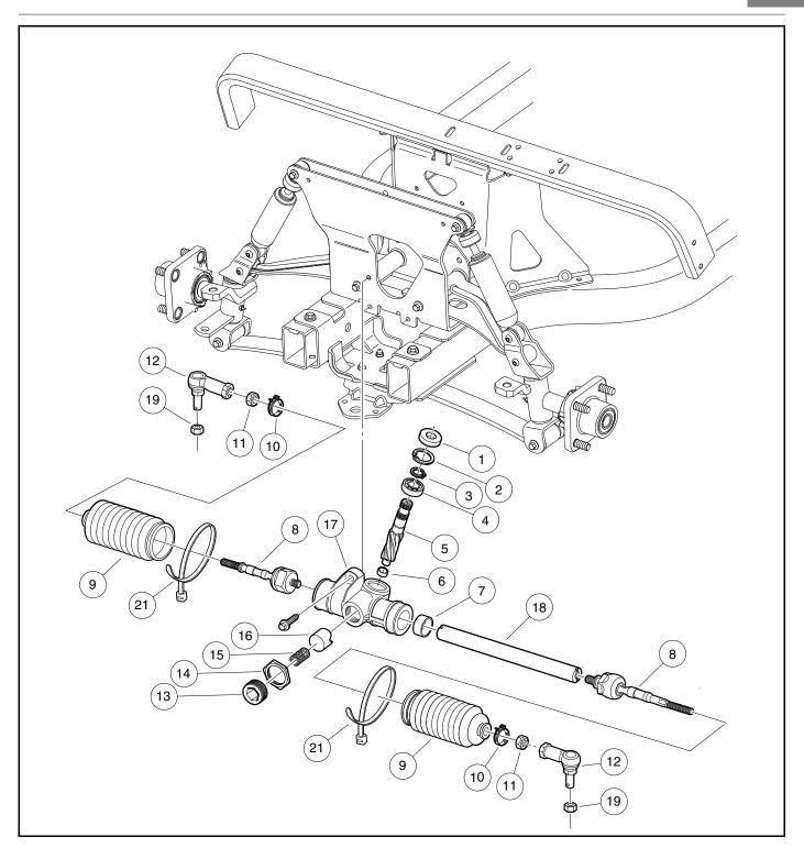
Figure 7-5 Steering Gear
