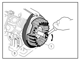
Figure 14-11 Fan and Flywheel Installation
