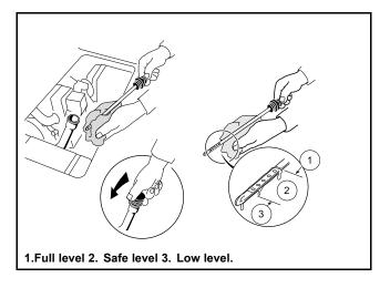
23 Figure 14-12 Check Engine Oil Level
