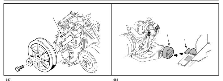
Figure 18-39 Driven Clutch and Key
