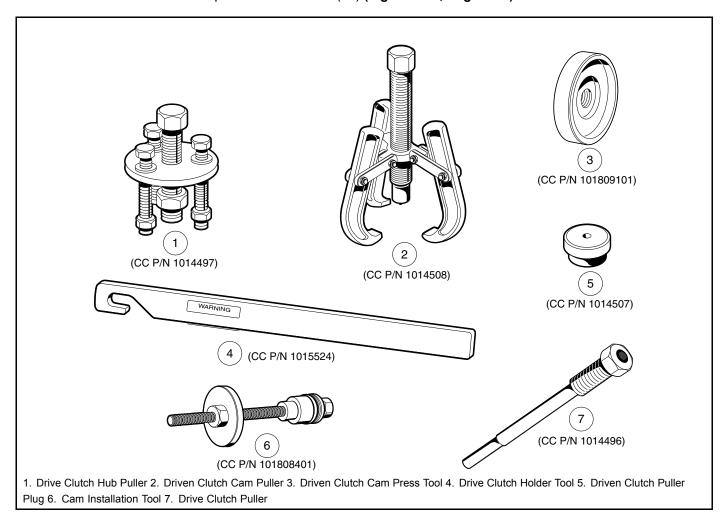
Figure 19-1 Torque Converter Tool Kit
