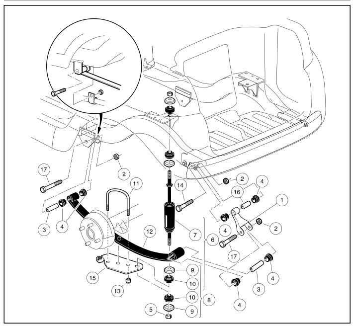
Figure 9-3 Rear Suspension Assembly and Mounting (Two-Passenger Vehicles)
