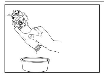
Figure 10-4 Remove Engine Oil Filter
