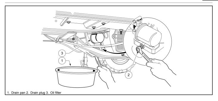
Figure 10-3 Engine Oil Drain Plug and Pan
