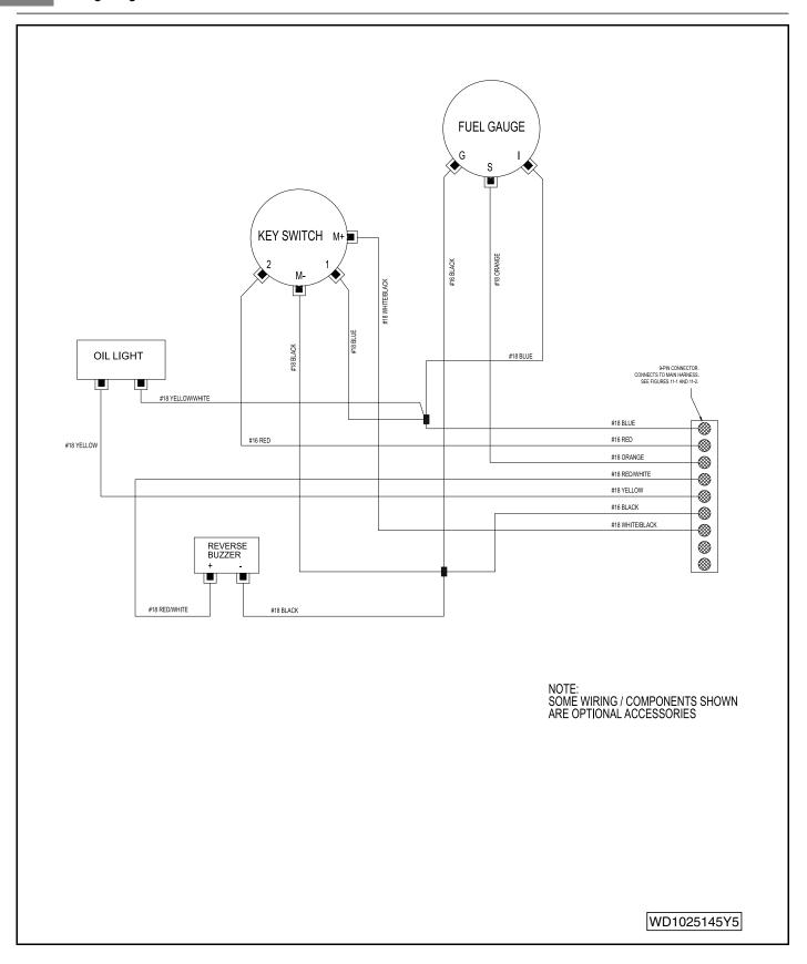
Figure 12-5 Precedent Gasoline Vehicle Instrument Panel Wiring Diagram
