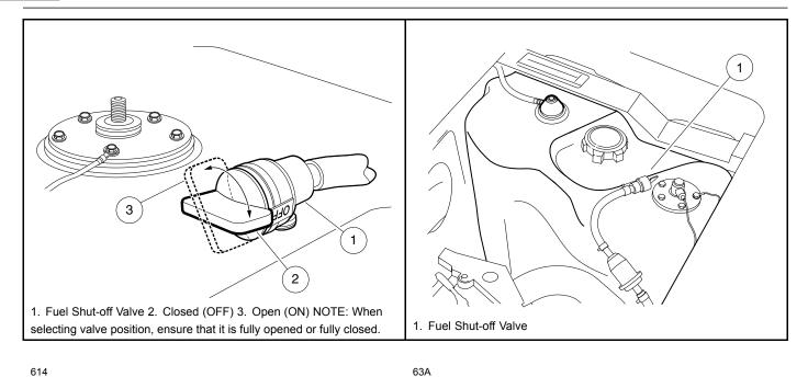
Figure 3-2 Fuel Shut-off Valve
