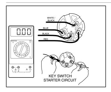
Figure 11-13 Test Key Switch - Engine Starter Circuit
