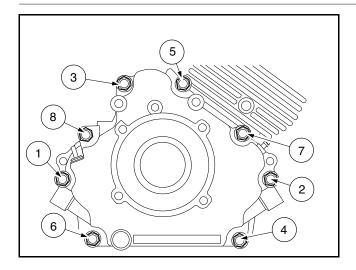
Figure 14-6 Crankcase Cover Installation
