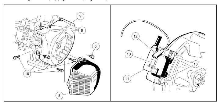
Figure 13-41 Fan Housing and Shroud Installation
