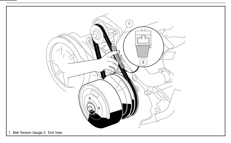
Figure 13-28 Belt Tension Gauge
