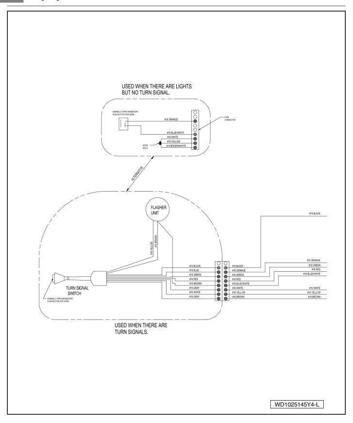
Figure 12-3 Precedent Gasoline Vehicle Accessory Wiring Diagram (Optional)
