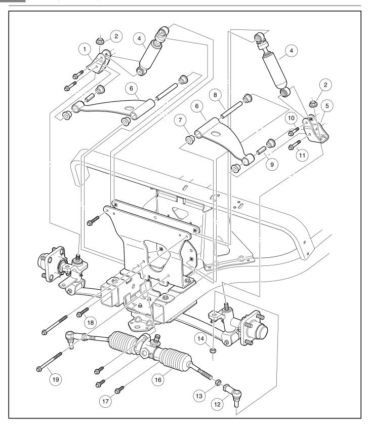
Figure 7-19 Upper Front Suspension Assembly
