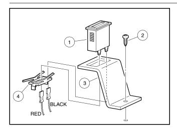
Figure 13-37 Hour Meter Installation
