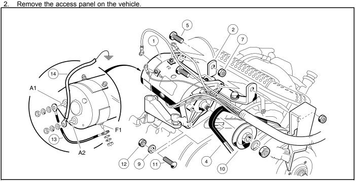
Figure 13-1 Starter/Generator Mounting
