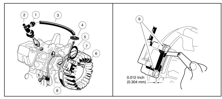
Figure 13-43 Coil Installation
