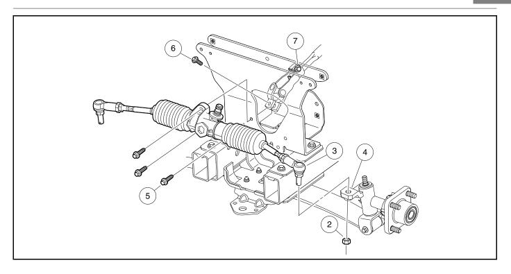
Figure 7-4 Rack and Pinion Removal
