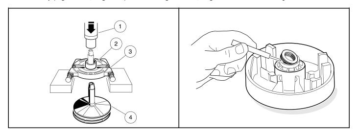
Figure 19-13 Remove Idler Bearing
