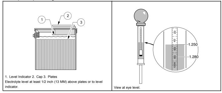
Figure 12-6 Battery Electrolyte Level
