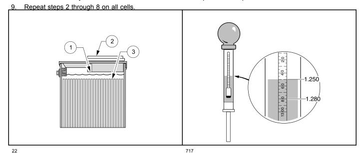
Figure 11-6 Battery Electrolyte Level
