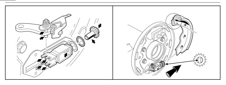
Figure 6-11 Apply Grease To Brake Adjuster
