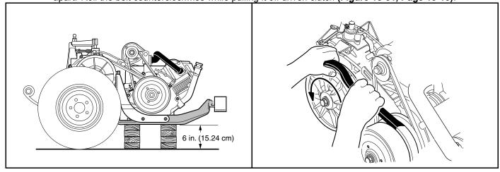
Figure 18-30 Position Powertrain on Wood Blocks
