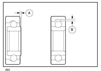
Figure 13-22 Bearing Play Inspection
