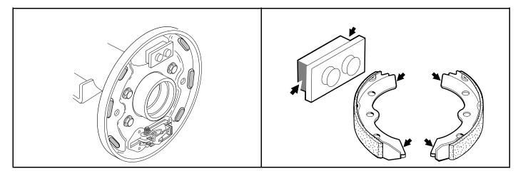
Figure 6-9 Apply Grease On Bosses
