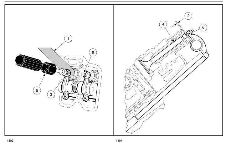
Figure 15-2 Measure Valve Clearance
