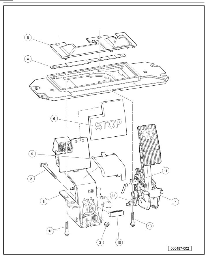
Figure 5-10 Accelerator Pedal Assembly and Brake Pedal Assembly
