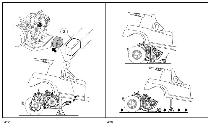
Figure 18-28 Snubber and Bracket
