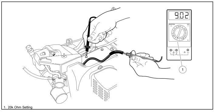
Figure 12-30 Secondary Coil Test Without Cap
