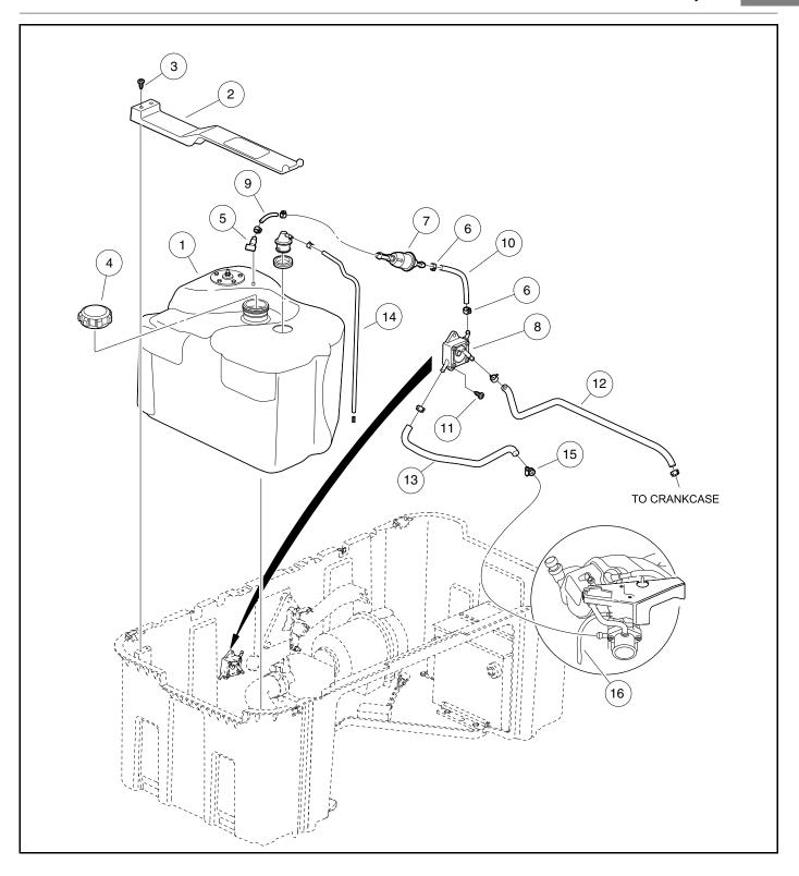
Figure 16-11 Fuel and Vent Lines
