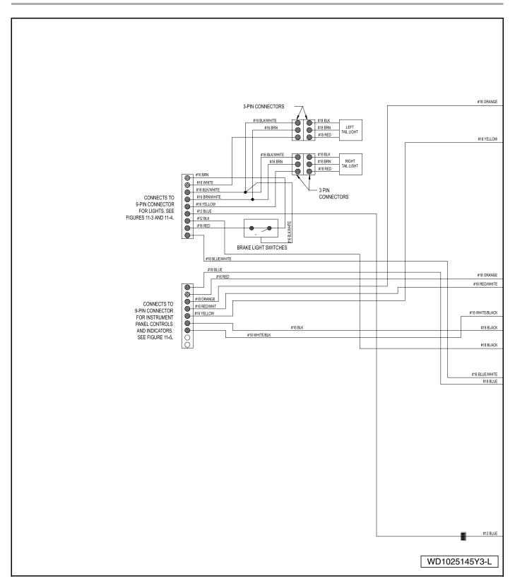
Figure 11-1 Wiring Diagram – Precedent Gasoline Vehicle with GCOR
