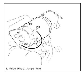
Figure 12-19 Jumper Wire Ground DF to A2 – Model G425419 shown
