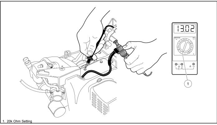
Figure 12-26 Secondary Coil Test - In Vehicle Test
