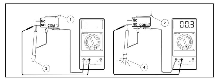
Figure 11-18 Test Neutral Lockout Switch
