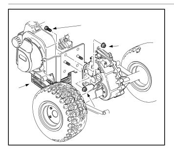
Figure 18-36 Transaxle Mounting
