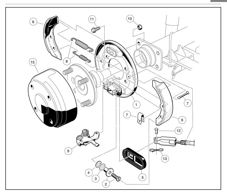
Figure 6-4 Self-adjusting Wheel Brake Assembly
