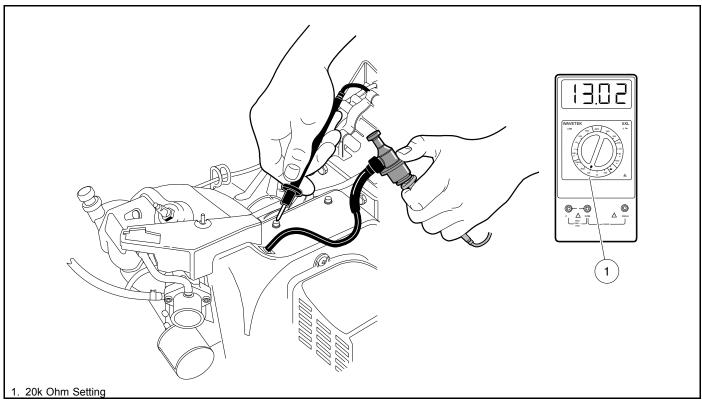
Figure 11-27 Secondary Coil Test - In Vehicle Test
