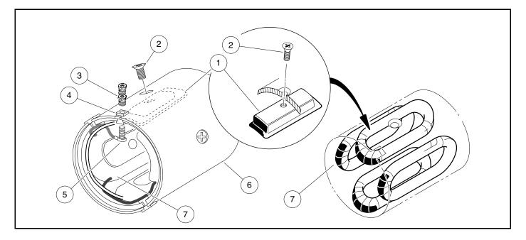
Figure 13-24 Field Coil Assembly
