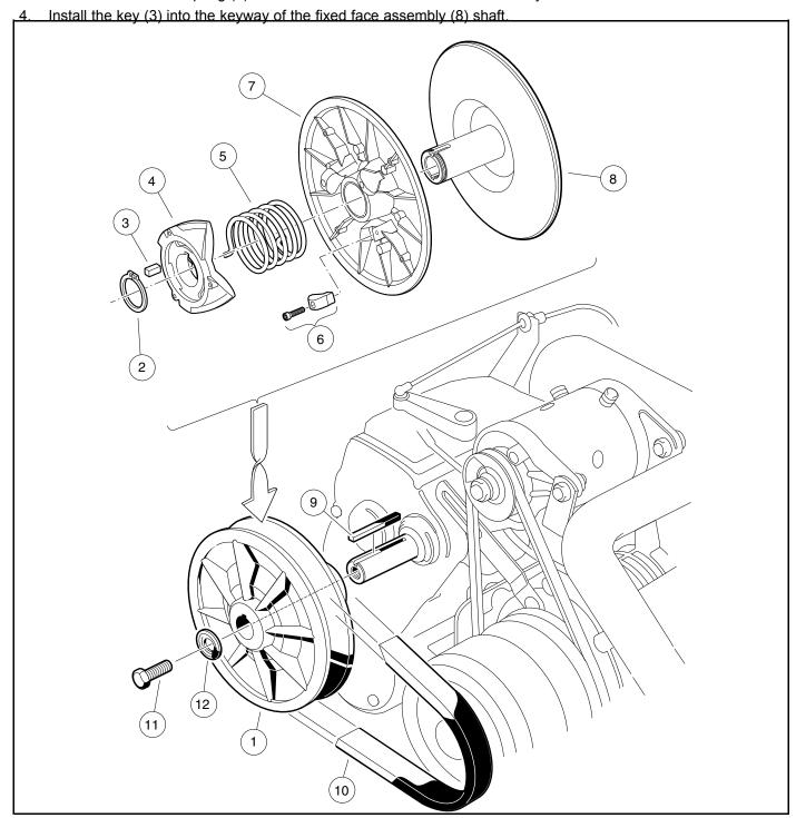
Figure 19-21 Driven Clutch Assembly
