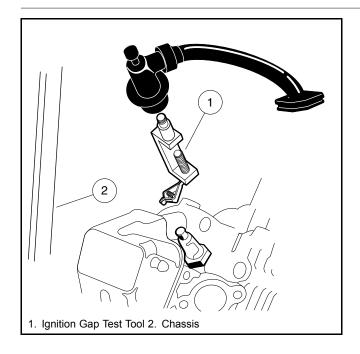
Figure 12-22 Ignition Spark Test
