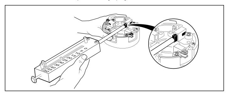
Figure 13-5 Brush Spring Tension Test
