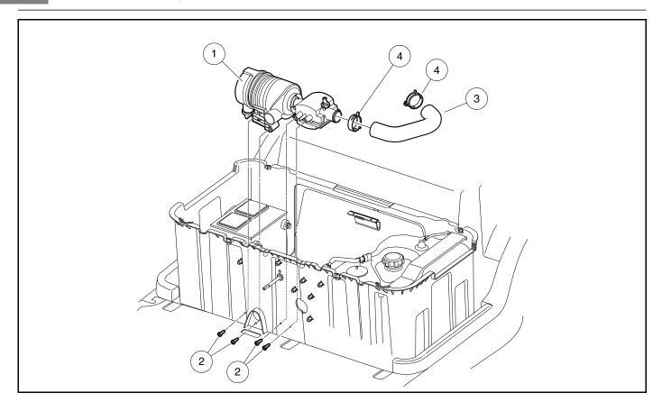
Figure 16-9 Air Intake and Choke Assembly
