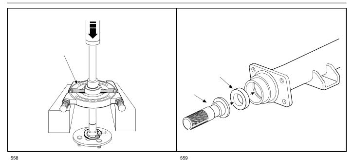
Figure 18-9 Press Bearing and Collar From Shaft Using Bearing Puller Wedge Attachment
