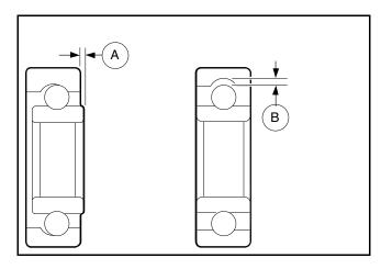
Figure 13-8 Bearing Play Inspection
