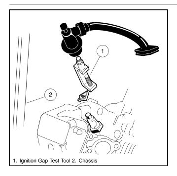
Figure 11-23 Ignition Spark Test
