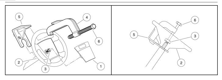
Figure 7-1 Steering Wheel Removal
