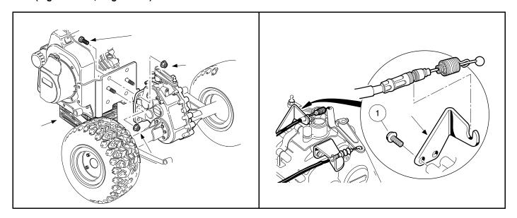
Figure 18-37 Transaxle Mounting
