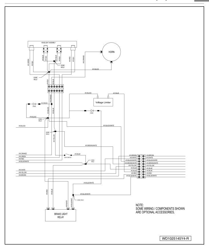
Figure 11-4 Precedent Gasoline Vehicle Accessory Wiring Diagram (Optional)
