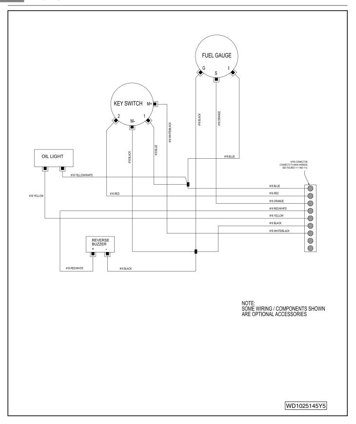
Figure 11-5 Precedent Gasoline Vehicle Instrument Panel Wiring Diagram
