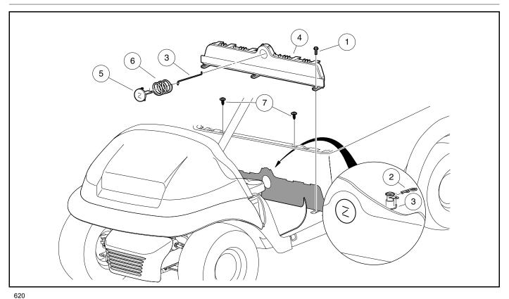
Figure 4-5 Kick Plate and Choke Button
