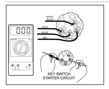
Figure 12-13 Test Key Switch – Engine Starter Circuit
