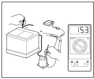
Figure 12-20 Voltage Regulator Test
