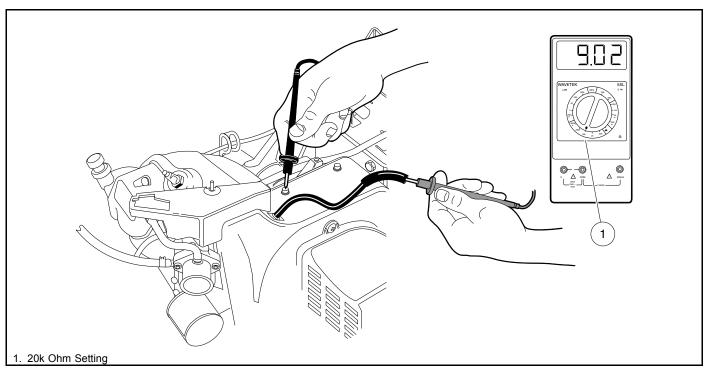
Figure 11-31 Secondary Coil Test Without Cap
