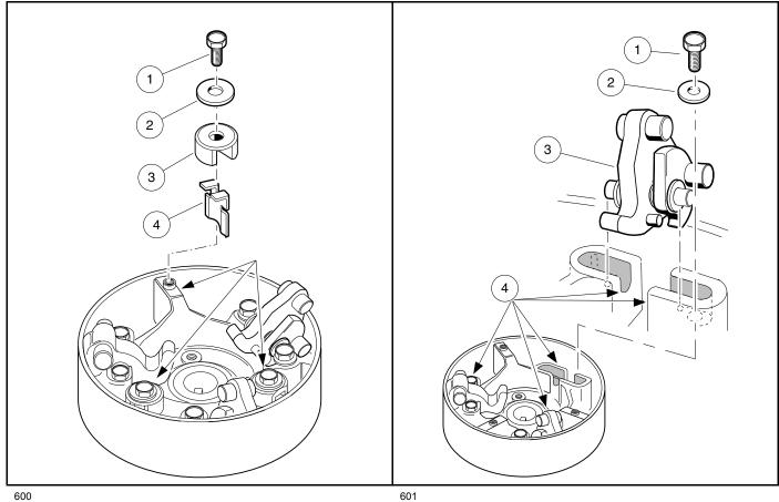
Figure 19-10 Drive Button Mounting
