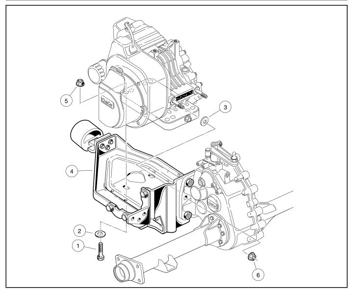
Figure 15-6 Engine Mounting Plate
