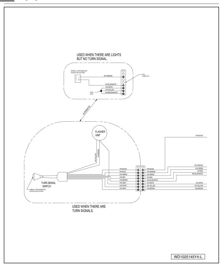
Figure 11-3 Precedent Gasoline Vehicle Accessory Wiring Diagram (Optional)
