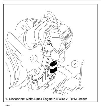
Figure 12-21 Disconnect White/Black Engine Kill Wire
