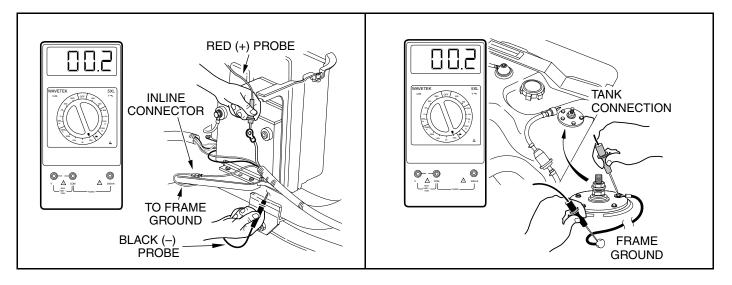
Figure 11-11 Battery Ground Cable Test
