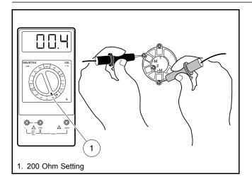
Figure 11-35 Test Key Switch - Engine Kill Circuit
