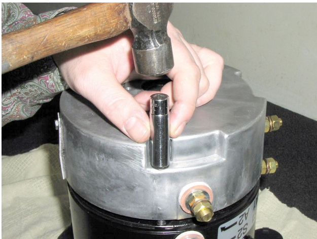
Figure 19-6 End Cap Disengagement
