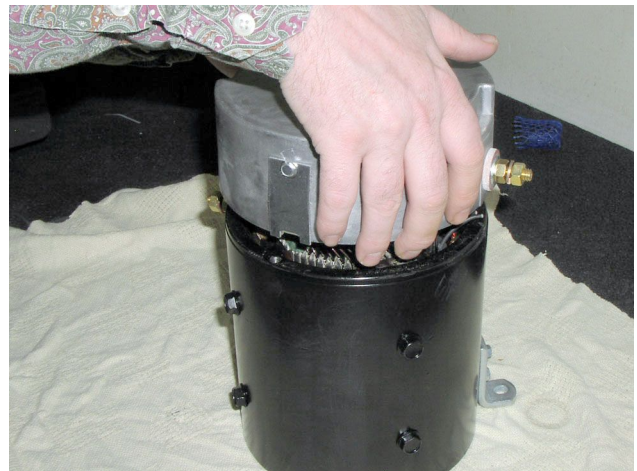
Figure 19-7 End Cap Removal
