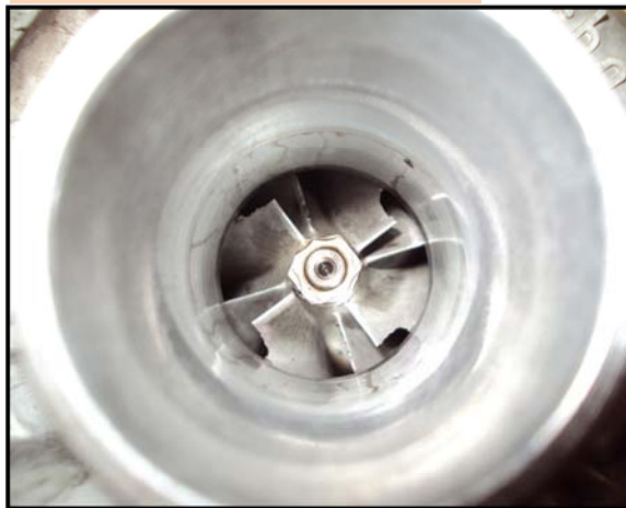
Lack of Lubrication - Worn Bearing
