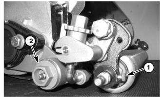
Figure 8 Roller retaining cap screw
