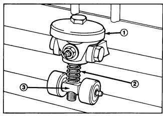
Figure 6a (Tool-adjustable knob)
