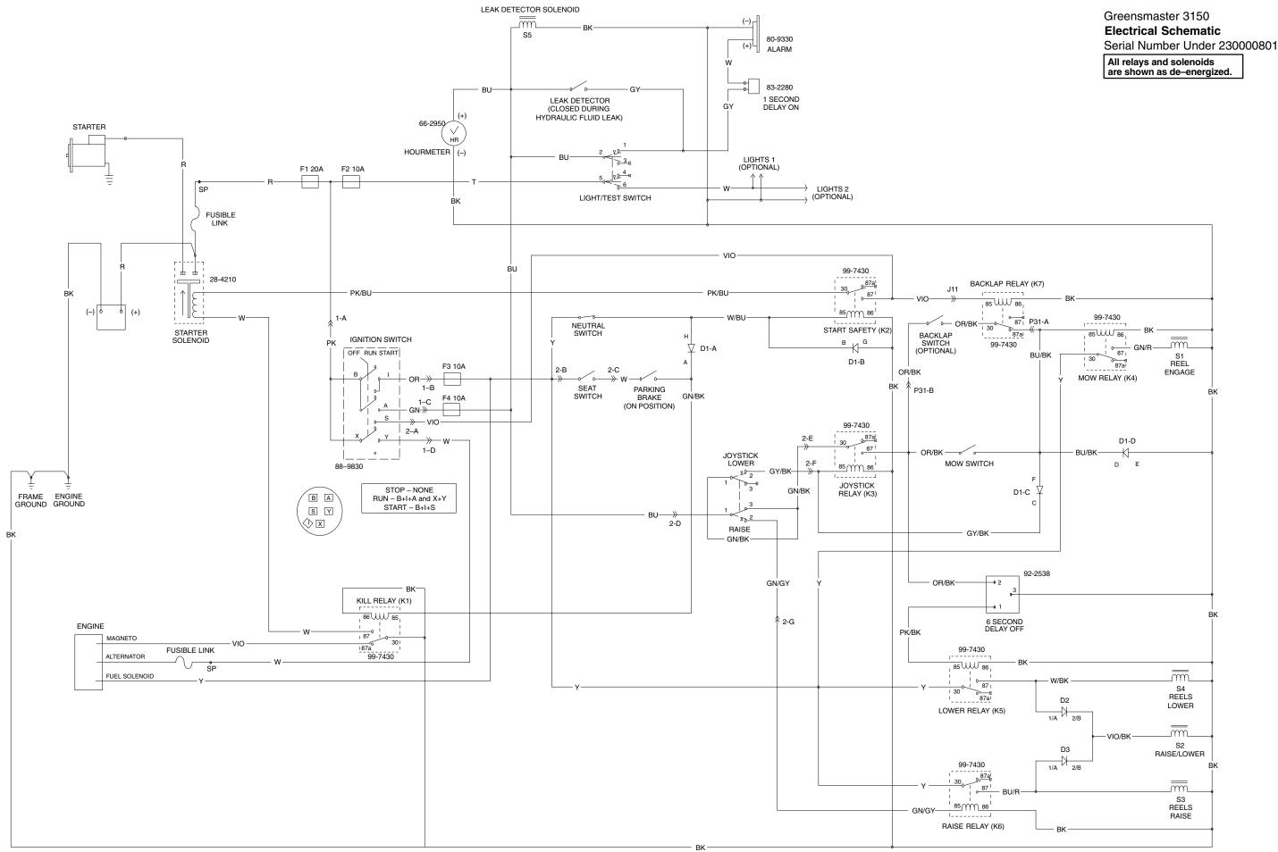
LEAK DETECTOR SOLENOID Greensmaster 3150 **Electrical Schematic** 80-9330 (+) ALARM Serial Number 230000801 & Up All relays and solenoids are shown as de-energized. 83-2280 1 SECOND DELAY ON LEAK DETECTOR (CLOSED DURING HYDRAULIC FLUID LEAK) 66-2950 STARTER HOURMETER (-) LIGHTS 1 (OPTIONAL) 3. F1 20A F2 10A V040 LIGHTS 2
