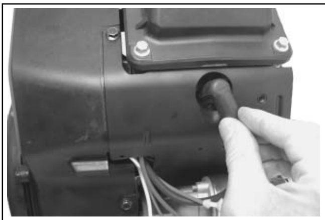
Figure 11-98. Connect Spark Plug Leads.
