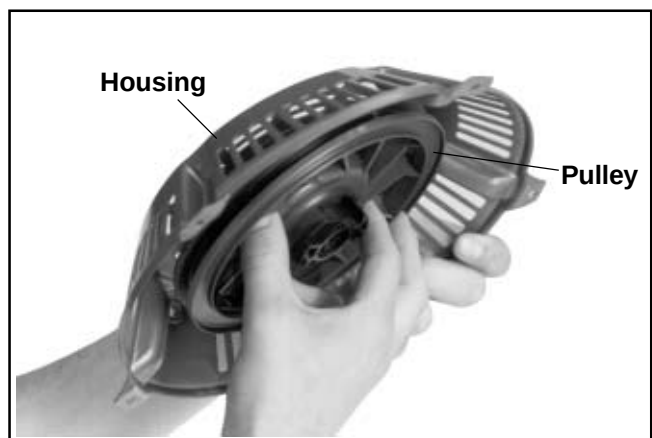
Figure 7-6. Removing Pulley from Housing.
