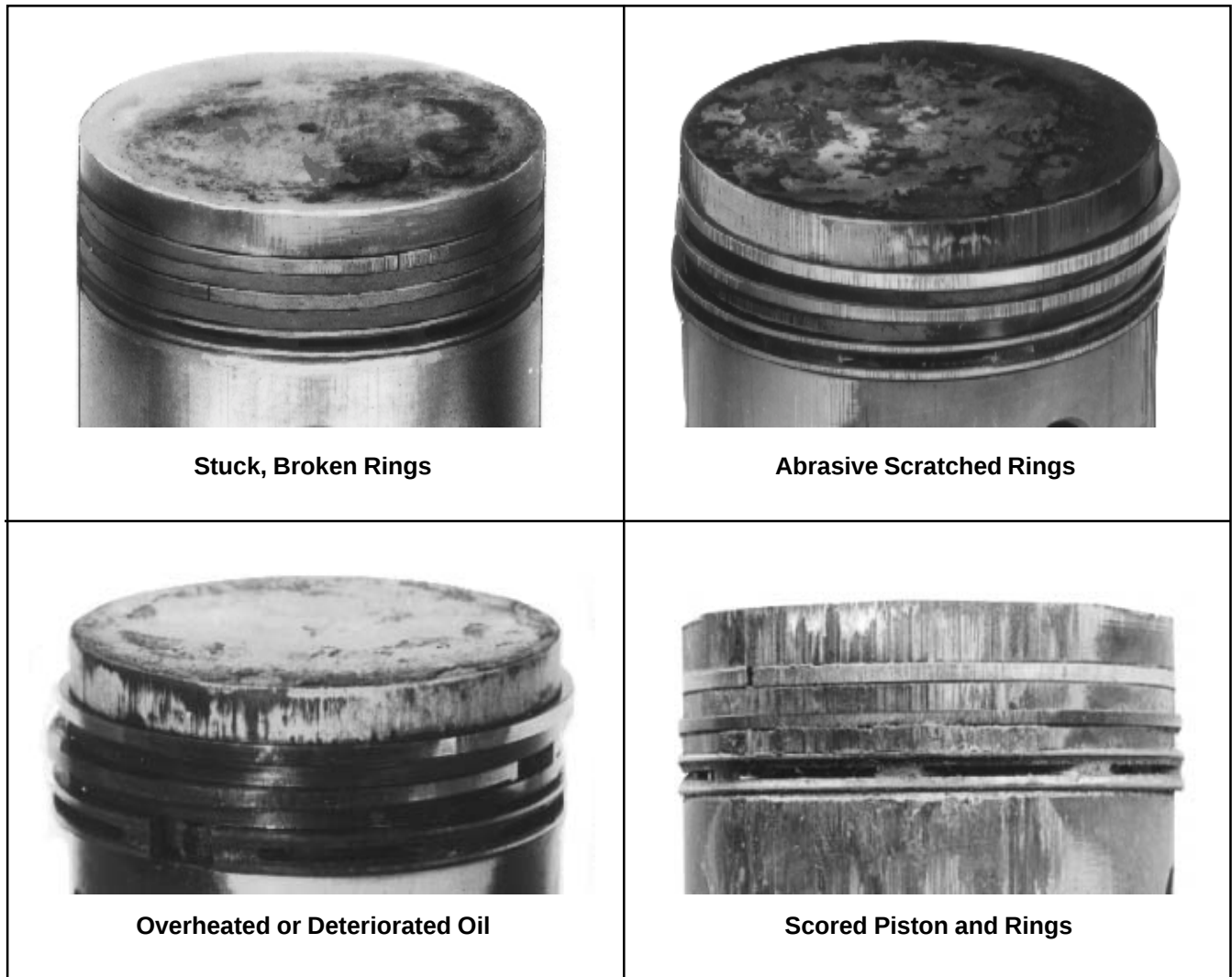
Figure 10-8. Common Types of Piston Damage.
