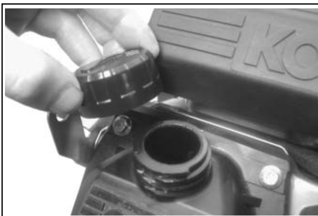
Figure 9-3. Removing Oil Fill Cap from Cover.
