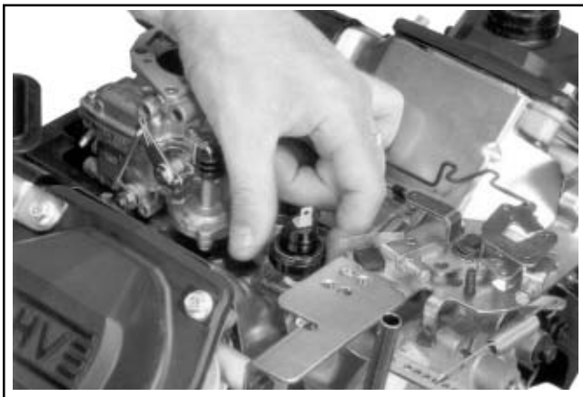
Figure 9-25. Removing Oil Sentry™ Switch from Breather Cover.
