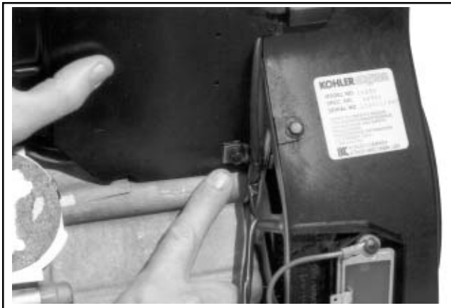
Figure 9-30. Note Location of Two Short Screws.
