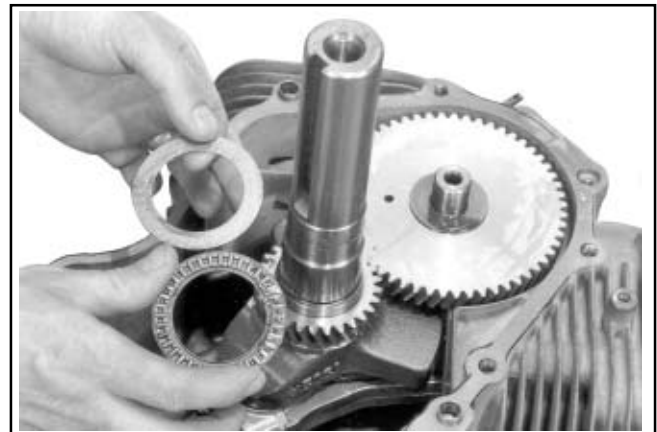
Figure 11-16. Thrust Bearing, Washer and Shim Used on Some Models.
