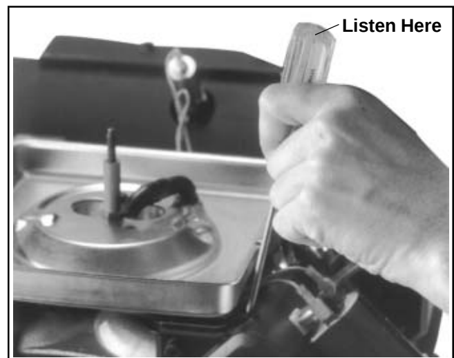
Figure 5B-19. Checking Injectors.
