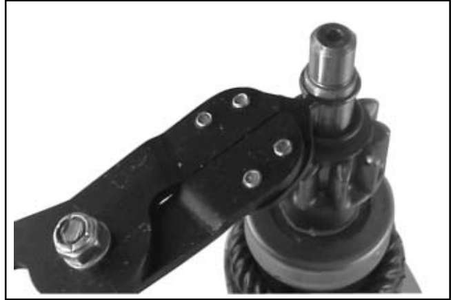
Figure 8-50. Removing Retaining Ring.
