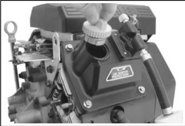
Figure 6-5. Removing Oil Fill Cap.
