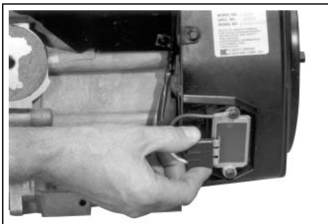
Figure 9-27. Disconnecting Plug from Rectifier-Regulator.
