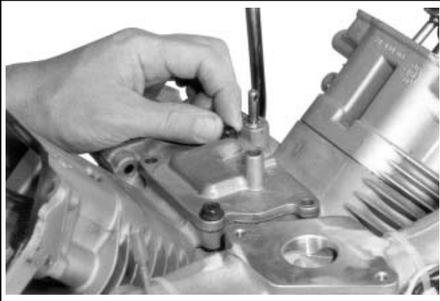
Figure 11-58. Installing Screws (Locations 3 and 4).
