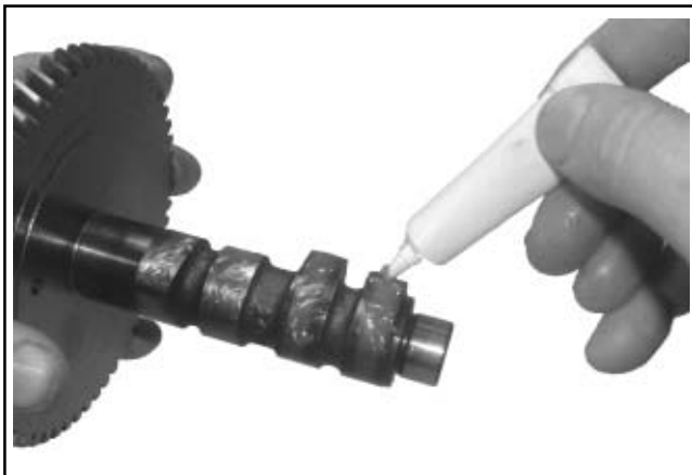
Figure 11-12. Apply Camshaft Lubricant to Cam Lobes.
