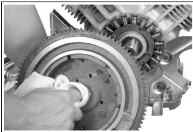
Figure 11-27. Clean and Dry Flywheel Hub.
