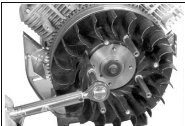
Figure 11-33. Torquing Supports for Metal Screen (Some Models).
