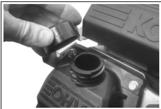
Figure 11-97. Reinstalling Oil Fill Cap (Some Models).
