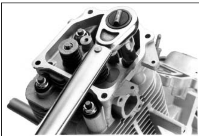
Figure 11-44. Torquing the Cylinder Head Mounting Nuts (Stud Design).
