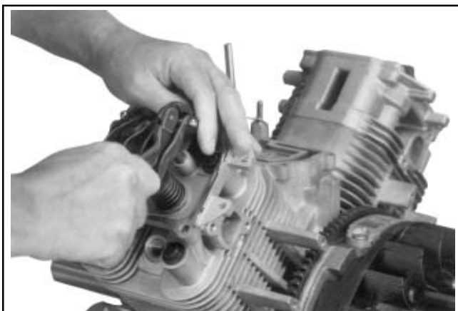
Figure 11-47. Using Spanner Wrench to Lift Rocker Arm Over Push Rod.
