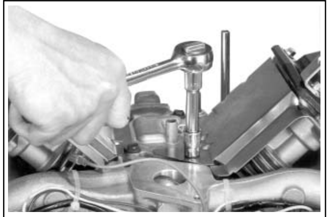
Figure 9-34. Removing Fasteners Holding Baffle and Breather Cover.
