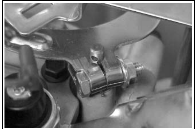
Figure 5B-41. Checking "Split" of Clamp.
