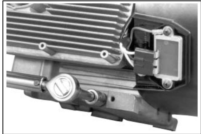
Figure 11-95. Reinstall and Torque Both Oil Drain Plugs.
