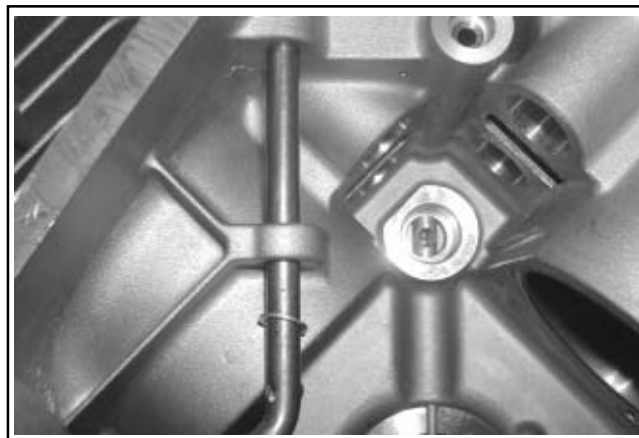
Figure 11-5. Installing 8 mm Governor Cross Shaft.
