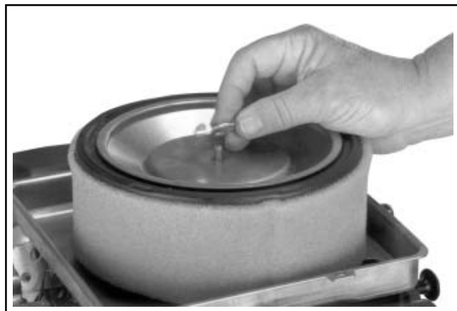
Figure 4-5. Removing Element Cover Wing Nut.
