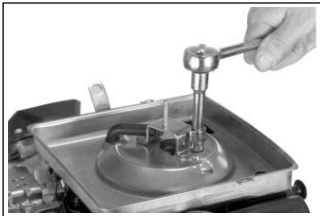
Figure 4-9. Bracket Retaining Screw.
