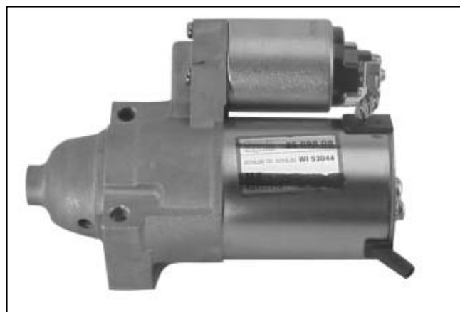
Figure 8-40. Completed Delco-Remy Starter.
