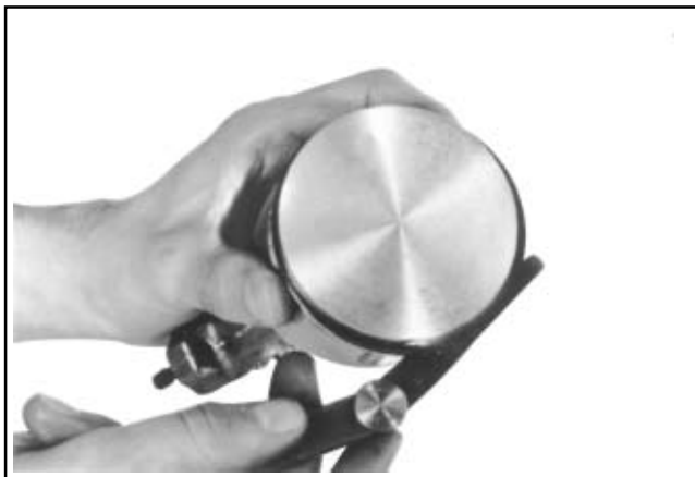
Figure 10-10. Measuring Piston Ring Side Clearance.
