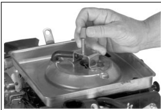
Figure 4-7. Removing Rubber Seal from Bracket.
