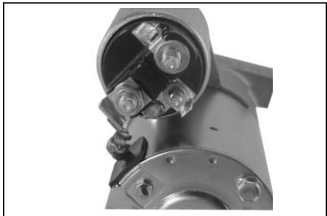
Figure 8-69. Positive (+) Brush Lead Connection.
