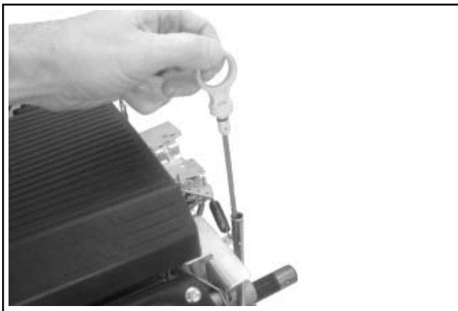
Figure 9-2. Removing Dipstick from Tube.
