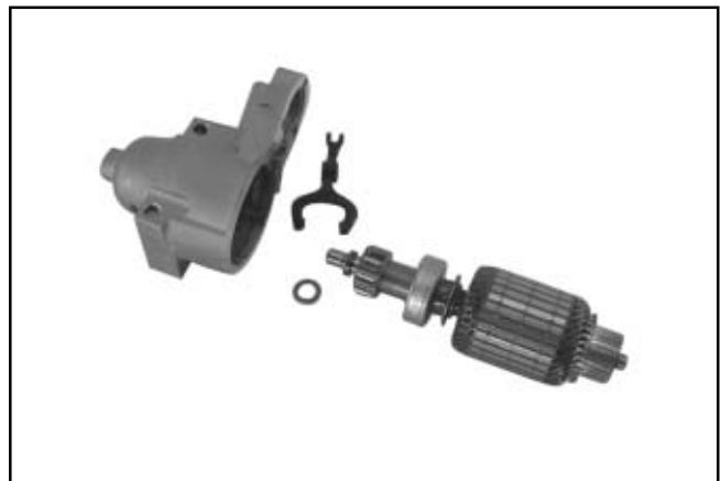
Figure 8-48. Armature and Lever Removed.
