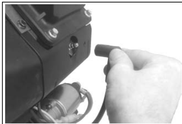
Figure 9-1. Disconnect Both Spark Plug Leads.
