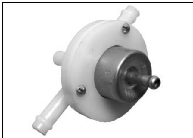
Figure 5B-28. Internal Fuel Pressure Regulator.
