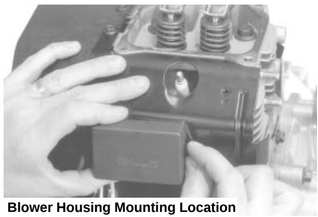
Figure 11-71. Reinstalling SAM Module.
