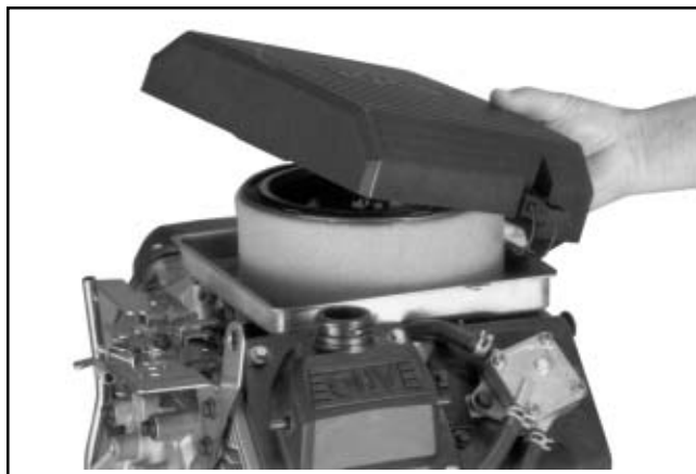
Figure 4-2. Removing Latch Style Cover.
