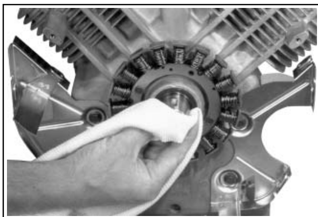
Figure 11-26. Clean and Dry Taper of Crankshaft.
