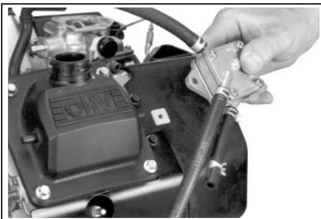
Figure 9-16. Remove Fuel Pump and Lines.
