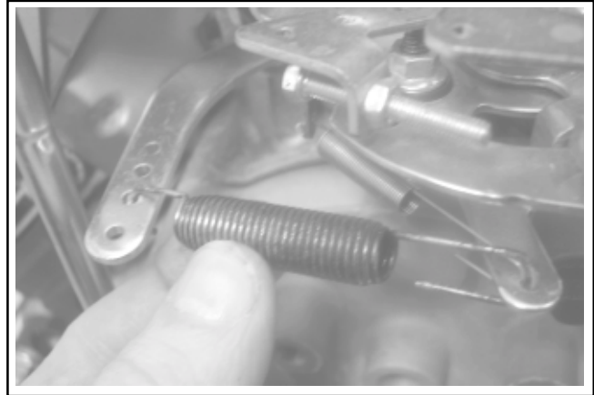
Figure 11-82. Connecting Spring to Governor Lever.
