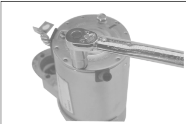
Figure 8-67. Torquing Thru Bolts.
