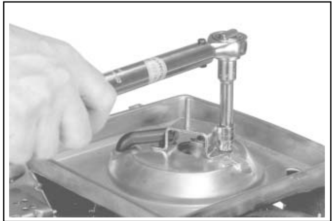
Figure 11-90. Torquing Base Screws.
