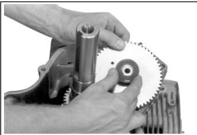
Figure 11-15. Change Shim to Obtain Correct End Play.
