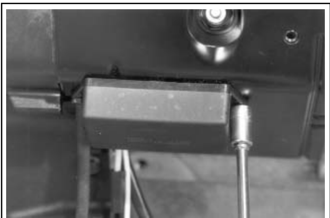
Figure 9-31. Removing Outer Baffles.
