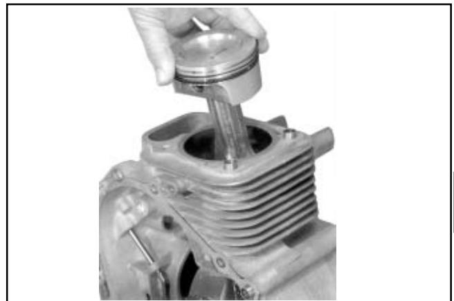
Figure 9-67. Removing Piston/Connecting Rod Assemblies.
