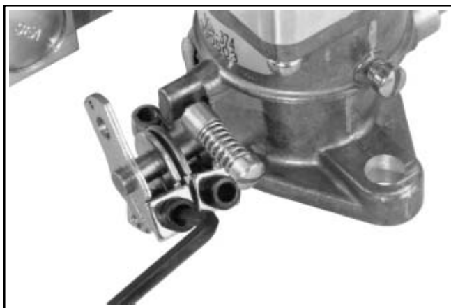
Figure 5A-14. Tightening Throttle Linkage Clamp Bracket.
