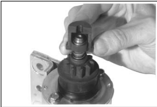
Figure 8-34. Assembling Larger Inner Half Around Spring Retainer.
