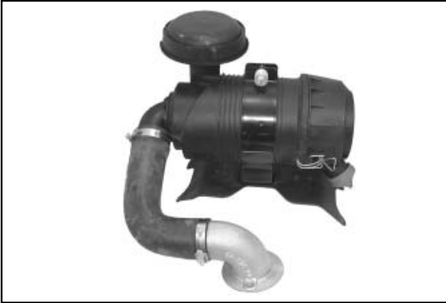
Figure 4-12. Heavy-Duty Air Cleaner.
