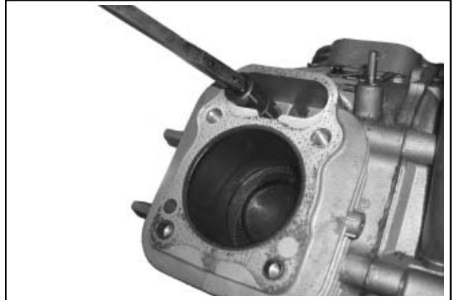
Figure 9-48. Removing Hydraulic Lifter.
