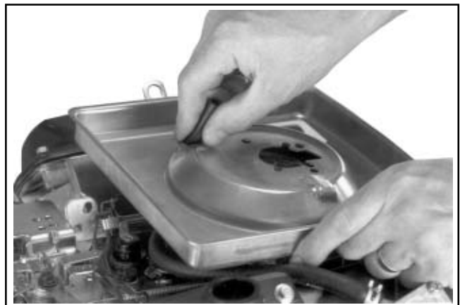
Figure 9-10. Removing Breather Tube from Base.
