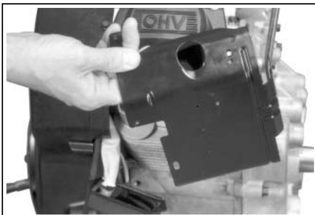
Figure 9-31. Removing Outer Baffles.
