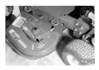
The Mower Deck Product Identification Number is located on the left hand side of the mower deck.
