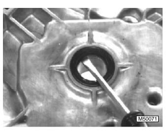
2. Remove worn or damaged seals with a screwdriver. (PTO end shown)
