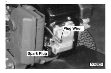
IMPORTANT: Spark plug wire must be grounded or electronic ignition could be damaged.
