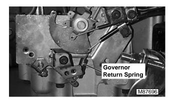
Governor return spring should be installed in hole closest to governor shaft. If not correct and adjust governor. See "GOVERNOR ADJUSTMENT" on page 24.
