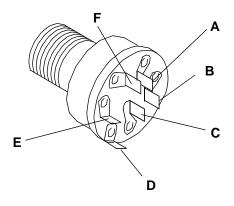
8. Check for continuity using JTO5791 Digital Multimeter and following table:
