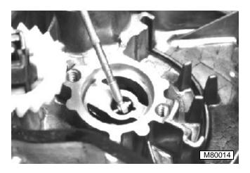
Measure crankcase cover oil pump bearing.
