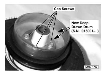
4. Install mounting cap screws and torque to 44 N•m (33 lb-ft).
