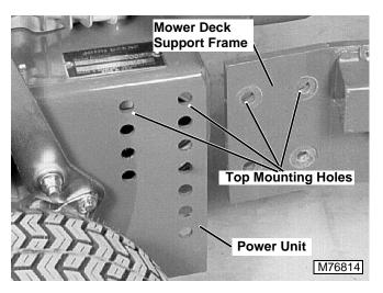
Align top holes of mower deck support frame with top holes of power unit. Install two cap screws in top holes on each side and loosely install nuts on cap screws.
