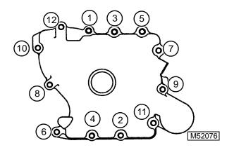
5. In sequence shown, tighten oil pan cap screws to specification.
