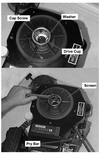
4. Remove cap screw and washer from bottom of drive cup by blocking flywheel with pry bar inserted into opening for carburetor intake. Remove drive cup, screw, washer, cup and screen.
