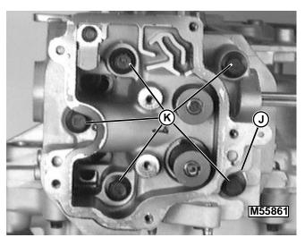
NOTE: Location of spacer (J) under lower right hand cap screw.
