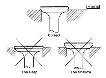
IMPORTANT: Center valve seat on the valve face.
