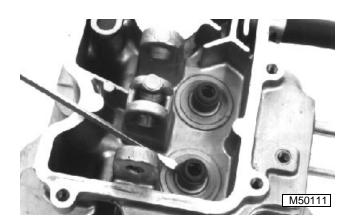
If necessary to replace stem seal, remove with screwdriver.
