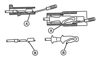
Use a small screwdriver to depress locking tang (A) terminal. Slide connector body off.
