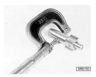
2. Measure pump rotor shaft. Replace if less than specifications:
