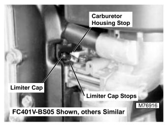
7. Rotate idle mixture screw back and forth between limiter cap stops until smoothest idle is obtained.
