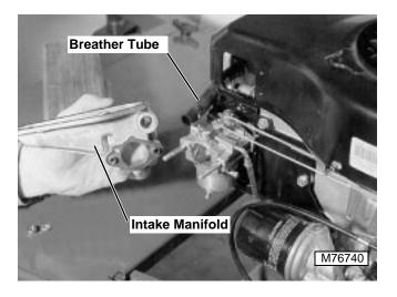
5. Separate intake manifold from carburetor and breather tube.
