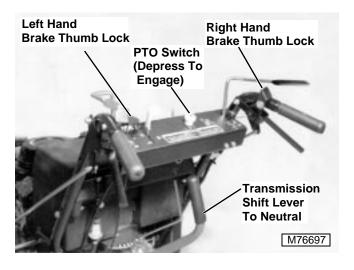
Move transmission shift lever to neutral position. Disengage PTO. Engage **both** brakes and thumb locks.
