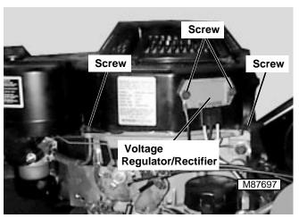
Remove two screws securing voltage regulator/rectifier to blower housing. Move voltage regulator/rectifier out of the way.
