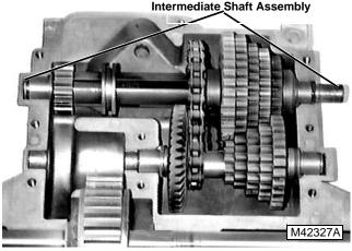
4. Install the remaining intermediate shaft components to the shaft in their proper order.
