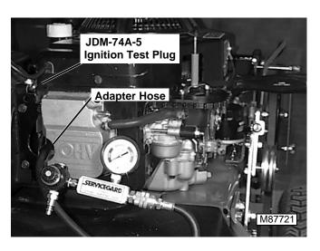
6. Ground ignition high tension lead using JDM-74A-5 Ignition Test Plug to protect ignition system and install test kit adapter hose into spark plug hole
