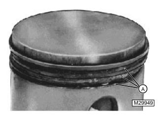
A cylinder bored at an angle to the crankshaft may result in improper ring contact with the cylinder which may cause the following:
