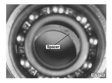
Pry inner spacer so that it is slightly to one side.
