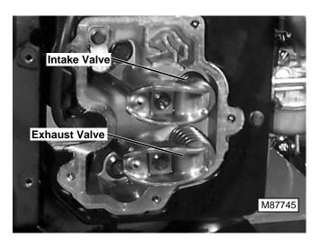
4. Use pull starter to turn flywheel clockwise until intake valve opens fully.
