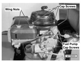
Remove wing nuts securing air cleaner. Remove air cleaner
