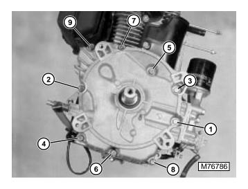
6. Install cover and gasket and tighten cap screws using the sequence shown. Evenly torque cap screws to 26 N•m (19 lb-ft).
