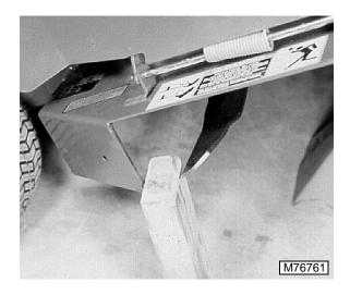
2. Block blade using a suitable piece of wood.
