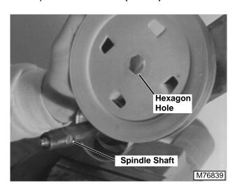
IMPORTANT: Make sure that the hexagon hole in the spindle sheave is in alignment with hexagon portion of spindle shaft.
