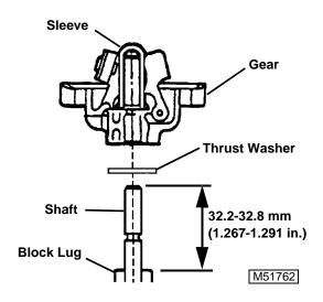
If removed, press shaft back into block lug until it protrudes 32.2—32.8 mm (1.267—1.291 in.).
