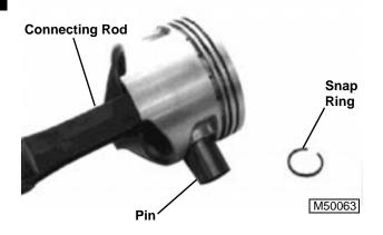
7. Remove snap ring, piston pin and connecting rod.
