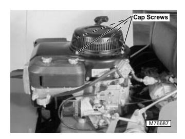
Remove four cap screws securing recoil starter assembly to engine. Remove recoil starter assembly.
