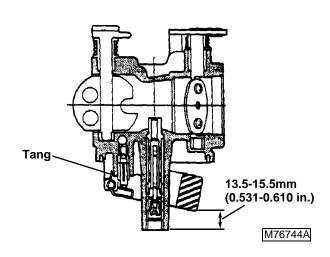
Invert carburetor, float down, and check dimension between bottom of float and end of jet holder. If not 13.5—15.5 mm (0.531—0.610 in.) adjust by bending stop tang.
