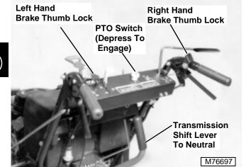
Move transmission shift lever to neutral position. Disengage PTO. Engage **both** brakes and thumb locks.
