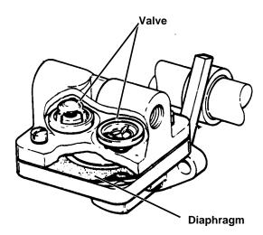
Inspect pump for wear or damage. Pay special attention to diaphragm and valves. If any damage is noted replace pump.
