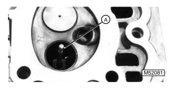
2. Measure inside diameter of guide with gauge (A).
