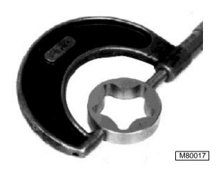
Measure outside diameter of outer rotor. Replace BOTH outer rotor and shaft if less than specification
