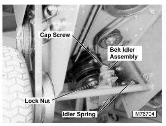
1. Disconnect spark plug wire and ground.
