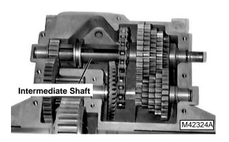
Visually check overall condition of assemblies, including gears for wear, pitting, broken teeth, etc. Replace as required.
