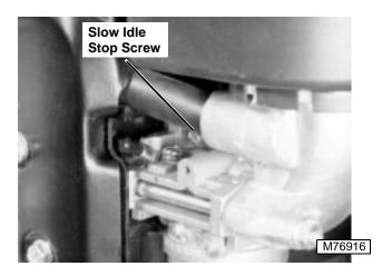
6. Turn slow idle stop screw on carburetor until slow idle speed is 1450 ±75 rpm.
