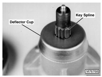
Install the deflector cup over the spindle and housing.
