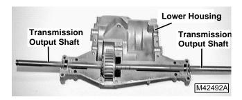
Remove the transmission output shafts from the lower housing half.
