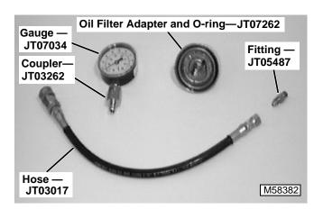
NOTE: SERVICEGARD™ Oil Pressure Test Kit (JT07262) only includes the oil filter adapter and O-ring. The hose (JT03017), gauge (JT07034), coupler (JT03262), and fitting (JT05487) are found in other SERVICEGARD test kits. The non-tapered threaded end of fitting (JT05487) matches the oil pressure port on Kohler engines.
