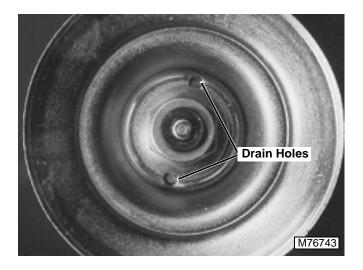
IMPORTANT: Drain holes in the drive sheaves indicate the orientation of the mower blades.
