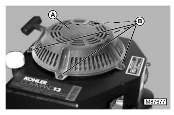
11. Place recoil starter (A) on engine. Secure with five (5) screws (B).
