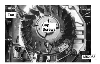
2. If fan requires removal from flywheel, remove four fan cap screws and washers and fan.
