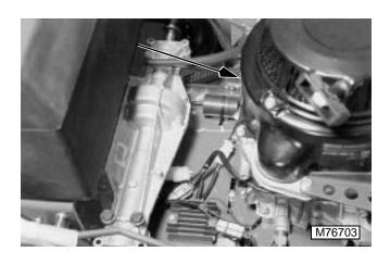
The engine serial number is located on the Fan Housing opposite the engine head.
