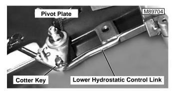
Remove cotter key from lower hydrostatic control link, and remove end of rod from hole in pivot plate.
