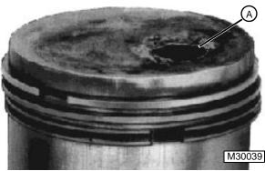
Pre-ignition is the igniting of the fuel-air mixture prior to proper ignition spark. Pre-ignition causes internal shock, resulting in pings, vibration, and power loss. Severe damage is caused to the piston crown (A), rings, and valves results from pre-ignition.
