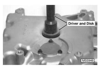
3. Using a suitable driver and disc, install new oil seal to specification.
