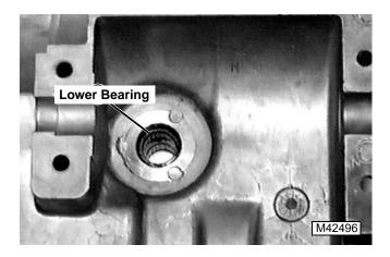
3. Install lower bearing with flat side of bearing (with lettering) toward inside of housing. Press into bore until flush—0.76 mm (flush—0.030 in.) from inside bore opening.
