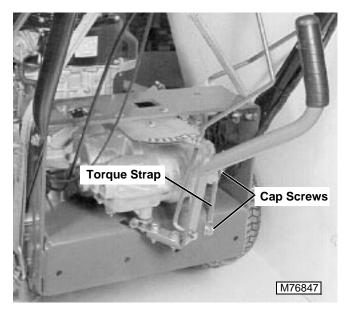
11. Remove the two (2) cap screws securing torque strap to the frame and the transmission.
