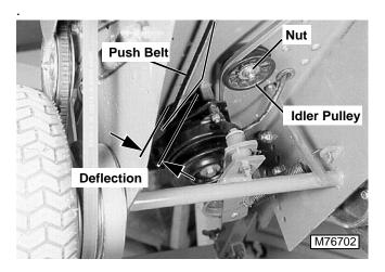
5. Push idler pulley against belt with approximately 16 kg (35 lbs) force and tighten nut to 27.1—40 N•m (20—30 lb-ft).
