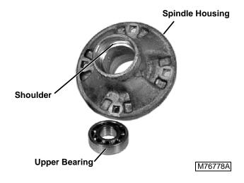
Lightly coat upper bearing with grease and install upper bearing tight against shoulder of spindle housing. 2. Coat seal with grease and install seal until flush with top of housing. Note correct seal orientation with lip facing bearing.
