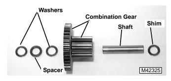
1. Install components on idler shaft in order shown:
