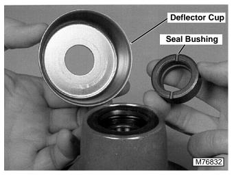
5. Remove deflector cup and seal bushing.
