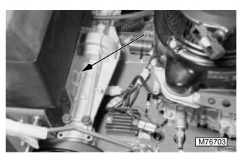
The gear transmission serial number is located on the transmission housing web.
