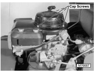
11. Place starter assembly on engine and secure with four (4) cap screws.
