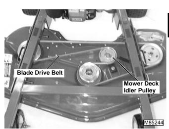
Pull spring loaded mower deck idler pulley to remove tension on blade drive belt. Remove blade drive belt from mower deck idler pulley.
