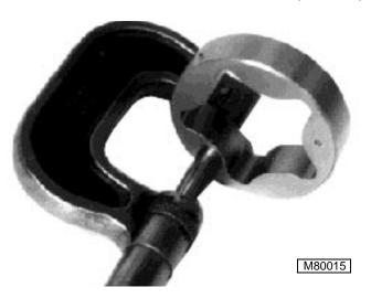
7. Measure thickness of outer rotor. Replace BOTH outer rotor and shaft if less than specification.
