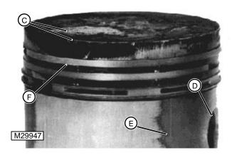
This detonation shockwave ("hammering") of the piston inside the cylinder causes damage to piston crown (C), top ring and groove (F), piston side skirts (E), and pin locks (D).
