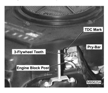
With a wide blade pry-bar move flywheel 3 teeth in the clockwise direction to insure the compression release mechanism is not activated.
