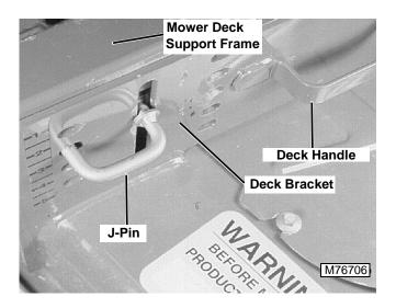
5. Pull all four J-pins from the frame and the deck brackets.
