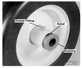
Align the relief on the outer bushing (indicated by a dot on the flange) with the grease fitting in the wheel.
