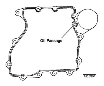
IMPORTANT: DO NOT get sealant in oil passage. Apply just enough to seal both sides of oil passage when case halves are fastened together.
