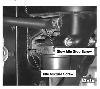
3. Carefully remove black limiter from idle mixture screw.
