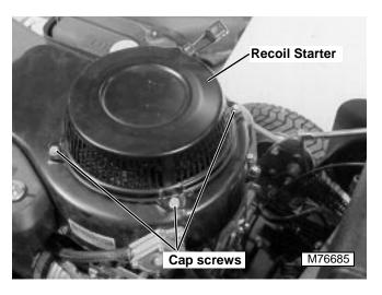
2. Remove four cap screws securing recoil starter to engine. Remove recoil starter.
