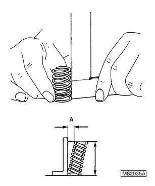
2. Inspect valve spring for squareness on a surface plate. Turn spring and measure space between top spring coil and square (A). Replace spring if not in within specifications.
