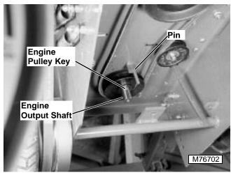
Apply NEVER-SEEZ lubricant to engine output shaft.
