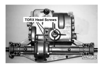
4. Remove all 16 transmission TORX™ head screws.
