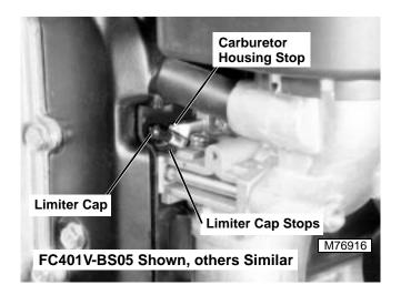
13. Center LIMITER CAP stop(s) between CARBURETOR HOUSING stop and install limiter cap onto slow idle mixture screw.
