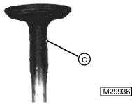
Use of old or stale gasoline can cause valves to stick.
