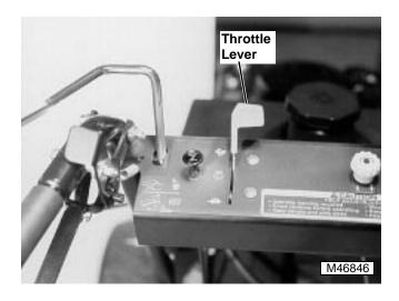
4. Move throttle lever to fast idle position.
