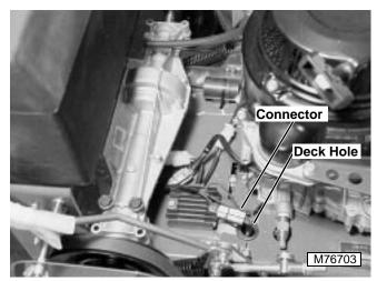
3. Disconnect PTO electrical connector. Push end of connector through hole in deck.
