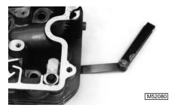
Put head on a flat surface plate. Check for distortion at several points with a feeler gauge. Replace head if distorted beyond specification.
