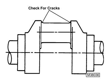
NOTE: Connecting rod journal can be resized to accept undersized rod. Have grinding done by a reliable repair shop. Before sending crankshaft for grinding, inspect journal radii for cracks.
