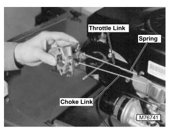
6. While removing carburetor disconnect throttle spring and remove throttle linkage and choke linkage.
