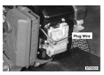
1. Disconnect spark plug wire.
