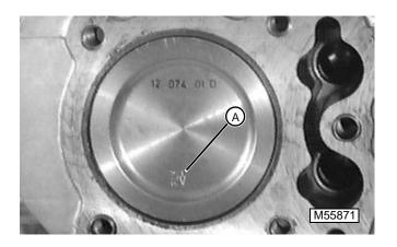
Install piston with FLY mark (A) toward flywheel side of crankcase. Use wooden dowel to push piston into bore.
