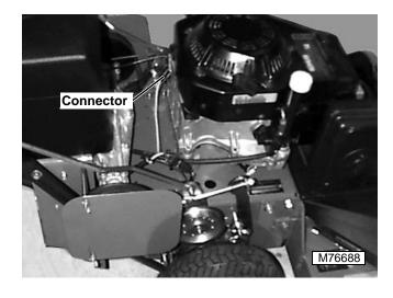
6. Connect engine electrical connector.
