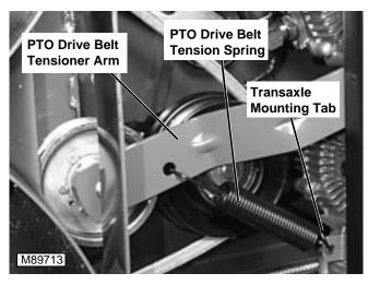
5. Remove PTO drive belt tension spring from tensioner arm and tab on transaxle.
