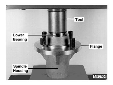
Place lower bearing, with shield facing out, in spindle housing and press until the bearing is seated on shoulder of the spindle housing.
