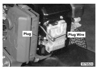
1. Disconnect spark plug wire and ground.
