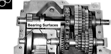
4. Inspect lower and upper housing combination shaft bearing surfaces for excessive scoring or wear. Replace housing halves as necessary.
