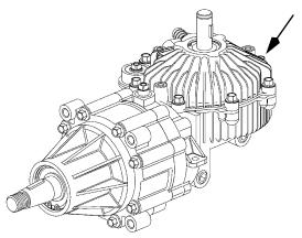
The hydrostatic transaxle serial number tag is bolted to the inside edge of the transaxle case, and can be seen from the rear of the mower deck.
