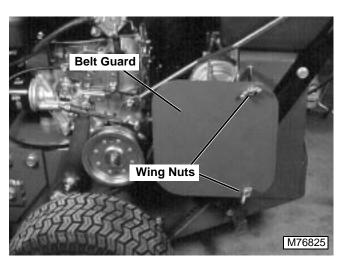
4. Remove belt guard and traction drive belt. See "TRACTION DRIVE BELT- REMOVAL AND INSTALLATION" on page 21.
