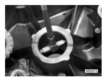
Measure crankshaft bearing in crankcase cover. Replace cover if diameter is greater than specifications. **Crankcase Cover Bearing I.D. for Crankshaft Specifications (Max):**
