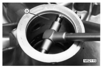
4. Measure inside diameter of crankshaft main bearing bore (D) in oil pan.
