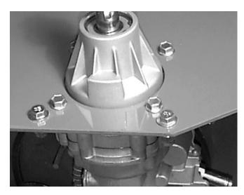
9. While supporting transaxle, remove four selftapping cap screws holding transaxle to mower deck. Carefully remove transaxle and reservoir as an assembly from power deck frame.
