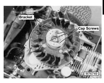
Remove three cap screws securing bracket to flywheel.
