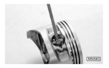
Measure piston pin bore. Replace piston if measurement is greater than specification.
