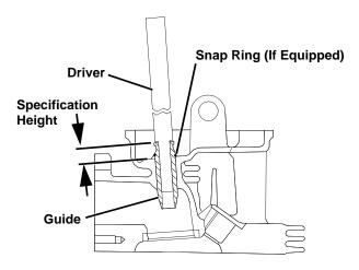
5. Coat outside surface of valve guide with a light coat of engine oil.
