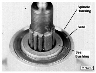
NOTE: Apply a light coating of grease to the inside and outside seal surfaces to protect seal lips and facilitate installation.
