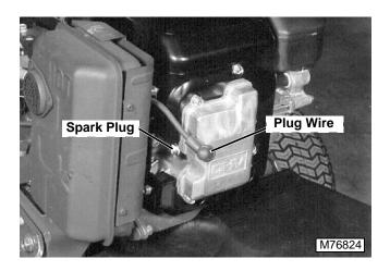
1. Disconnect spark plug wire and ground.
