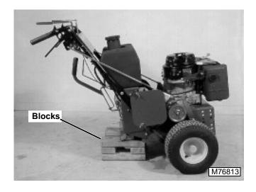
Support power unit with jack stand, blocks or other safe suitable means.
