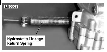
5. Remove hydrostatic linkage return spring from lower hydrostatic control link and frame.
