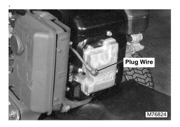
3. Disconnect spark plug wire and ground.
