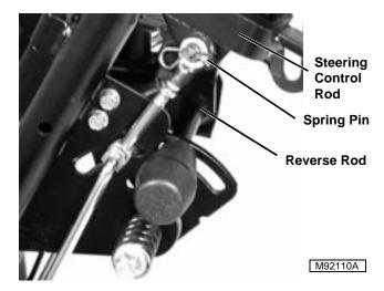
13. Remove spring pin and washer holding reverse rod to steering control lever from left and right side.
