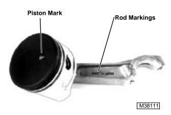
2. Align arrow match mark on piston head with MADE IN JAPAN on connecting rod web, or if piston is marked with "R" and "L", alight the "R" on the piston with the Japanese characters on the rod web.
