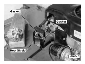
1. Place a gasket on either side of heat shield and install heat shield on studs.
