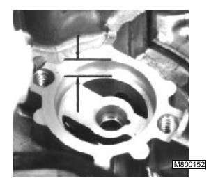
Measure outer rotor bearing depth. Replace crankcase cover if greater than specification. Oil Pump Rotor Bearing Depth Specifications: FC401V-BS05, FC420V-AS19... 12.14 mm (0.478 in.) FC540V-AS17 & AS18 ....... 10.17 mm (0.401 in.)
