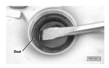
IMPORTANT: DO NOT damage seal bore when removing seal.
