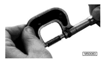
9. Measure relief valve spring. Replace if length is less than 19.00 mm (0.750 in.)
