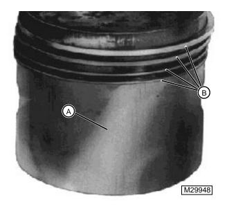
Check rod and piston alignment when piston shows a diagonal wear pattern (A) extending across the skirt of the piston. Contact with the cylinder wall shows on bottom of skirt at left and ring lands on the right (B).
