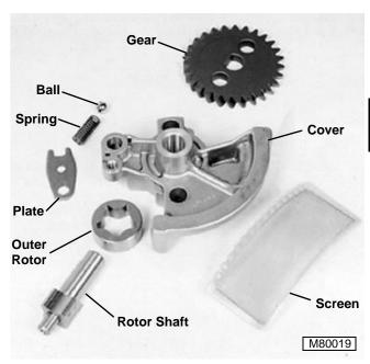
1. Inspect all parts. Replace if worn or damaged.
