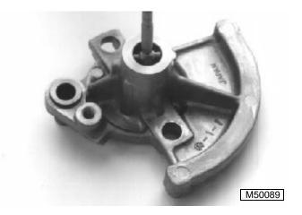
3. Measure pump cover bearing. Replace cover if greater than 12.76 mm (0.502 in.)
