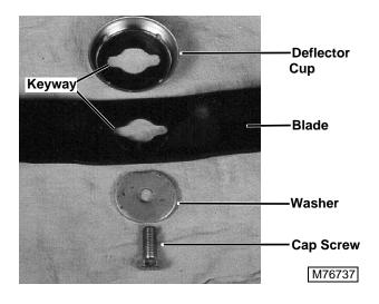
NOTE: The deflector cup and blade are keyed to the spindle shaft.
