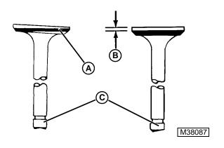
3. Replace warped valves (A) or valves with less than serviceable margin (B). Valve stem ends (C) should be square, not worn uneven as shown.
