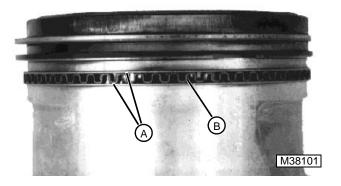
Abrasive particles in engine oil cause scratches on side rails (A) of oil control ring. If inner spacer (B) of oil control ring is worn or distorted it may cause:
