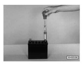
9. Use an hydrometer to check for a **minimum** specific gravity of 1.225 with less than 50 point variation in each cell.
