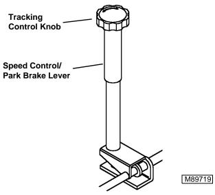
14. Turn tracking control knob in clockwise until it stops, then back out two turns. Cycle speed control lever a few times to allow spring to take up play in linkage.
