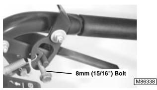
1. Install something that is approximately 8 mm (5/16 in) in diameter – such as a 8 mm bolt - in between the brake lever stud and the brake thumb lock.
