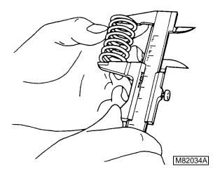
Measure free length of valve spring. Replace valve spring if not within specifications.
