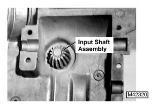
Install input shaft assembly into bearings from inner side of upper housing. Keyway should be on outside of housing.
