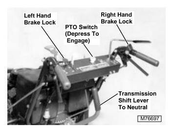
Move transmission shift lever to neutral position. Disengage PTO. Engage both brakes and locks.
