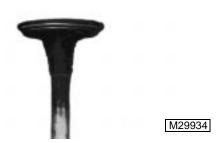
3. Replace warped valves (A) or valves with less than serviceable margin (B). Valve stem ends (C) should be square, not worn uneven as shown.
