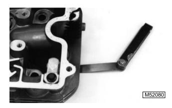
3. Put head on a flat surface plate. Check for distortion at several points with a feeler gauge. Replace head if distorted beyond specification.
