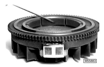
4. Place screwdriver about 25 MM (1 in.) from magnets.
