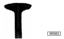
Inspect valve stems for bends using V-blocks and dial indicator. Turn valve slowly and read variation. Replace if variation is greater than 0.03 mm (0.001 in.).
