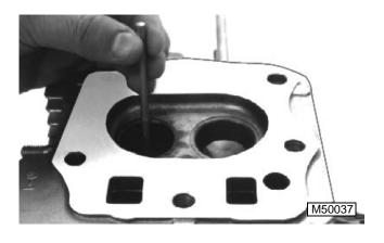
Measure inside diameter of valve guides. Replace Guide if inside diameter is greater than **7.07 mm (0.278 in.)**
