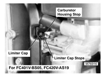
2. On **FC401V-BS05**, **FC420V-AS19**, use screwdriver to pry off limiter cap from slow idle mixture screw.
