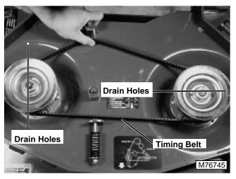
IMPORTANT: Proper blade orientation exists when one set of drain holes is positioned 90° in relation to the other set.
