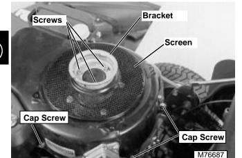
Remove three screws securing bracket to flywheel standoff bracket. Remove bracket and flywheel screen. Take care not to loose shims under bracket.
