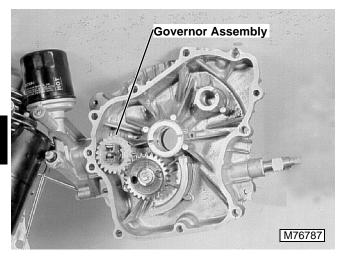
Inspect governor. If necessary to replace, remove with screwdriver.
