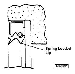
3. Install seal with spring loaded lip to inside of engine. Press seal in until flush with hub.
