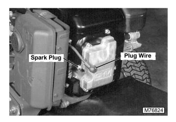
1. Disconnect spark plug wire and ground.
