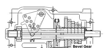
1. Visually check overall condition of assemblies, including gears for wear, pitting, broken teeth, etc.
