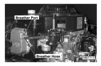
3. Disconnect crankcase breather hose from valve cover breather port and remove air cleaner element from engine so you can listen for air leaks.
