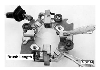
Measure brush lengths. Minimum brush length is 10.5 mm (0.413 in.). Brushes are not individually serviceable. If brushes are worn replace entire brush holder assembly.
