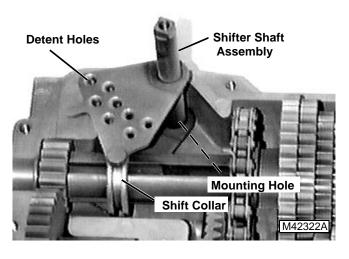
1. Lift shifter shaft assembly from mounting hole and disengage from groove in shift collar.
