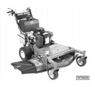
The Commercial Walk-Behind Power Unit Product Identification Number is located on the right hand side of the drive train housing.
