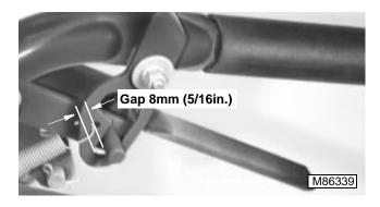
Remove bolt used as a spacer between brake lever stud and the brake lever lock. NOTE: If gap is less than 6mm (1/4 in.) the vehicle's traction may be restricted.
