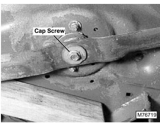
2. Block blade using a suitable piece of wood.
