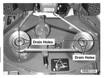
IMPORTANT: A properly timed mower deck must have one blade oriented 90° to the other blade. Due to belt stretching, tension on the timing belt should be adjusted after first 25 hrs. of use and at 100 hr. intervals afterward.
