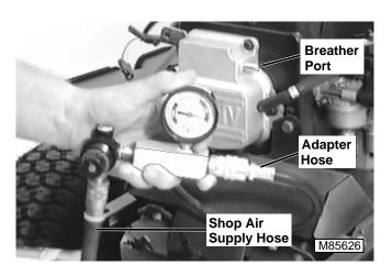
NOTE: A slight air leak from the breather port is normal as air escapes from the crankcase through the oil drainback hole in the head and breather valve.
