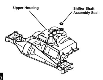
1. Inspect shifter shaft assembly seal and replace, if necessary.
