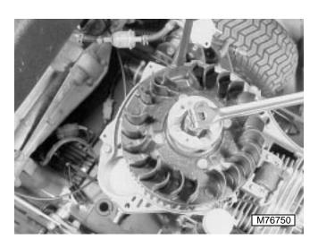
2. Remove flywheel nut. Use strap wrench around flywheel.
