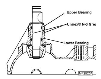
4. Pack needle bearings and gap between bearings with Unirex® N-3 grease before installing input shaft.
