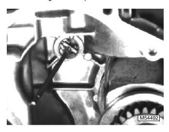
1. Measure camshaft bearings in cylinder block.
