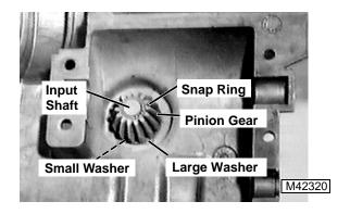
1. Remove snap ring, pinion gear, small washer, and large washer from input shaft.
