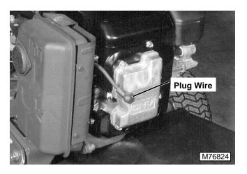
1. Disconnect spark plug wire and ground.
