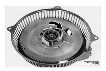
7. Turn the reel clockwise until NO spring tension can be felt.
