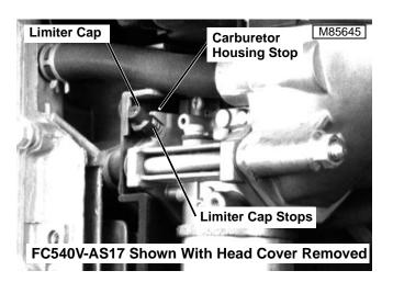
4. Use screwdriver to pry off limiter cap from slow idle mixture screw.
