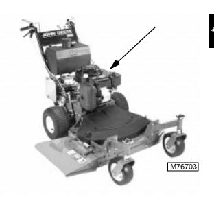
The engine serial number is located on the Fan Housing next to the carburetor intake air filter cover.
