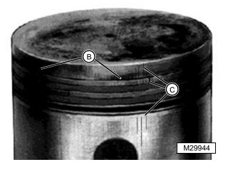
The engine operating at abnormally high temperatures may cause varnish, lacquer, or carbon deposits (B) to form in the piston grooves making the rings stick. When this happens, excessive oil consumption and blowby will occur.
