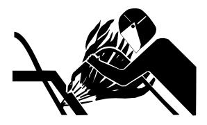
Flammable spray can be generated by heating near pressurized fluid lines, resulting in severe burns to yourself and bystanders. Do not heat by welding, soldering, or using a torch near pressurized fluid lines or other flammable materials. Pressurized lines can be accidentally cut when heat goes beyond the immediate flame area.
