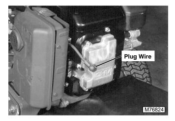
1. Disconnect spark plug wire.
