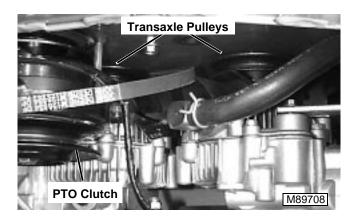
Install belt up over PTO electric harness, and electric clutch.
