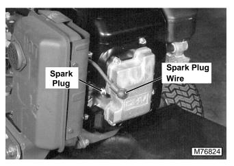
2. Disconnect and ground spark plug wire.
