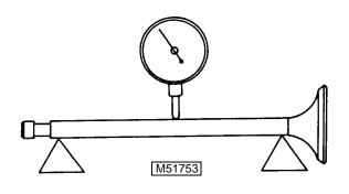
4. Inspect valve stems for bends using V-blocks and dial indicator. Turn valve slowly and read variation. Replace if variation is greater than specification.
