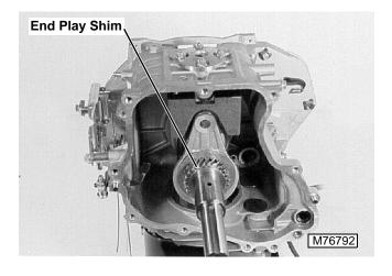
4. If play is not within specifications remove crankcase cover and replace shim.
