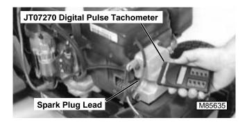
5. Check engine rpm with JT07270 Digital Pulse Tachometer.
