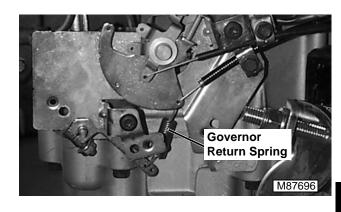
2. Governor return spring should be installed in hole closest to governor shaft. If not correct and adjust governor. See "GOVERNOR ADJUSTMENT" on page 24.
