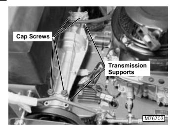
14. Remove caps screws securing transmission to frame. Remove transmission supports from under transmission.
