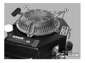
Remove five (5) screws (B) securing recoil starter (A) to blower housing. Remove recoil starter assembly.
