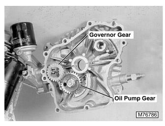
5. Make sure governor gear and oil pump gear are properly aligned to mesh with drive gear when installing cover.
