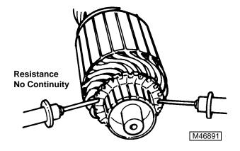
NOTE: Test armature windings using an ohmmeter or test light.
