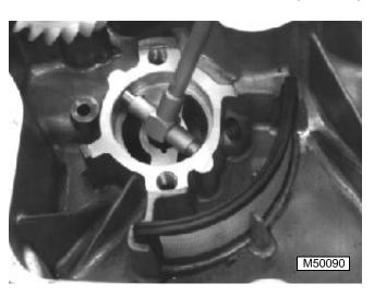
6. Measure inside diameter of rotor housing. Replace crankcase cover if greater than specification.
