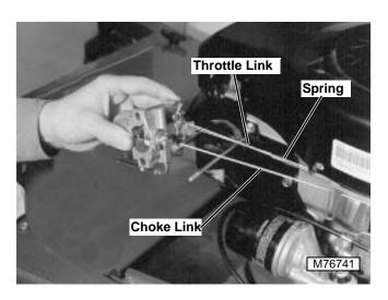
2. Connect throttle link, throttle spring, choke linkage and install carburetor.
