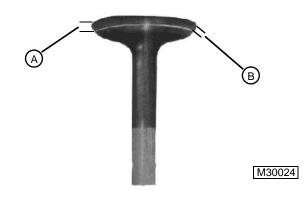
Operating at high temperatures for long periods of time can cause exhaust valve burning. Burned valve will show dark discoloration into the area protected by the valve guide. Another indication is distortion of the margin (A) and face angle (B). The valve seat may also show erosion.
