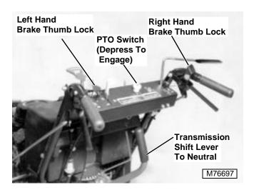
Move transmission shift lever to neutral position. Disengage PTO. Engage **both** brakes and thumb locks.
