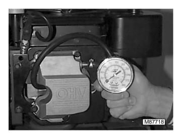
IMPORTANT: Spark plug wire must be grounded or electronic ignition could be damaged.
