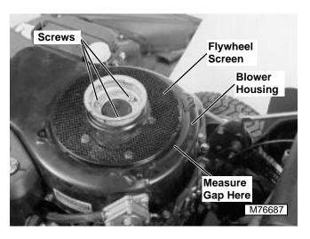
3. Check gap between flywheel screen and blower housing. If gap is less than 1.5 mm (0.059 in.) remove three screws securing starter pawl bracket to flywheel. Remove bracket and flywheel screen.
