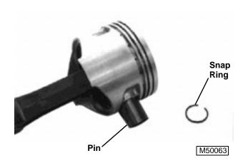
Install pin in piston and rod. Secure with snap ring at each end.
