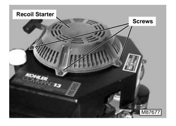
3. Remove five (5) screws securing recoil starter to blower housing. Remove recoil starter assembly.
