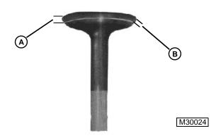
Measure valve stem diameter in several places. Replace valve if measurement exceeds specifications.
