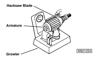
14. Test for short circuited windings using a growler. Put armature in a growler and hold a hacksaw blade above each slot while slowly rotating armature.
