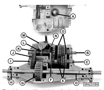
The pinion gear (A), which is splined to the input shaft and retained by a snap ring, drives the beveled gear (F). The beveled gear is splined to the drive shaft (C), as are the five forward drive gears (E).
