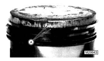
Light scuffing or scoring (A) of both rings and piston occurs when unusually high friction and combustion temperatures approach the melting point of the piston material.
