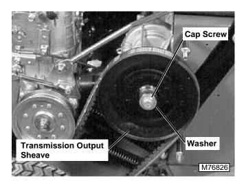
Remove the cap screw and washer retaining the transmission output sheave. NOTE: The transmission output sheaves are threaded to facilitate removal. Thread the appropriate size cap screw into the threaded end of the sheave to press off the sheave and belt.
