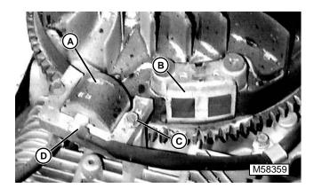
Turn flywheel magnet (B) away from ignition module (A).
