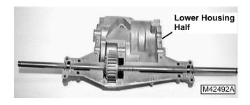
5. Install the transmission output shaft assembly into lower housing half.
