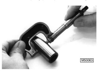
8. Measure piston pin outer diameter. Replace if less than specification.
