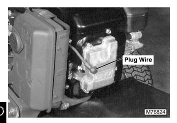
1. Disconnect spark plug wire and ground.
