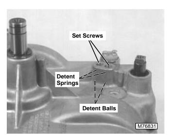
6 - 2411/5/97 1. Remove both set screws and detent springs.
