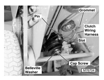
2. Install PTO clutch on shaft with pin through slot in coil housing.
