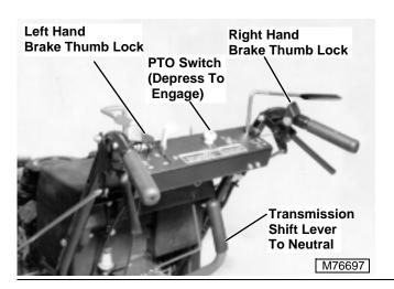
Park machine on level surface, turn key switch OFF, and allow engine to cool. Move transmission shift lever to neutral position. Disengage PTO. Engage both brakes and thumb locks.
