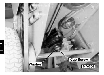
7. Remove cap screw, washer, and PTO clutch.
