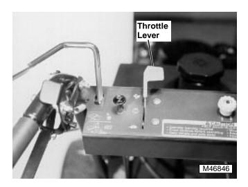
2. Move throttle lever to fast idle position.
