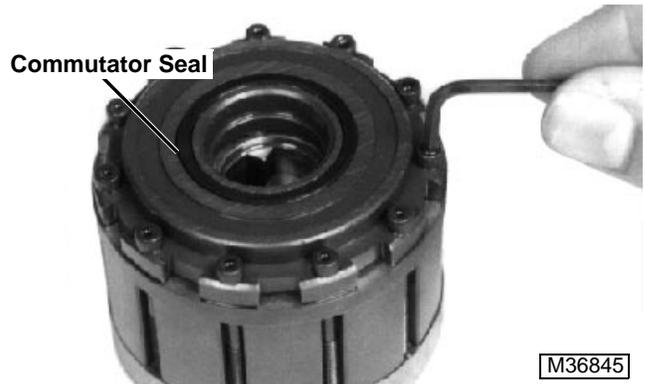
21. Remove commutator seal.
