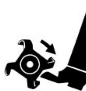
Keep hands and feet away while machine is running. Shut off power to service, lubricate or unlatch cutting units.
