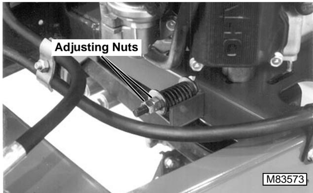
8. Loosen four engine cap screws and nuts and belt tension adjusting nuts. Engine should be free to move back and forth, but not tip. Move engine as far forward as possible.
