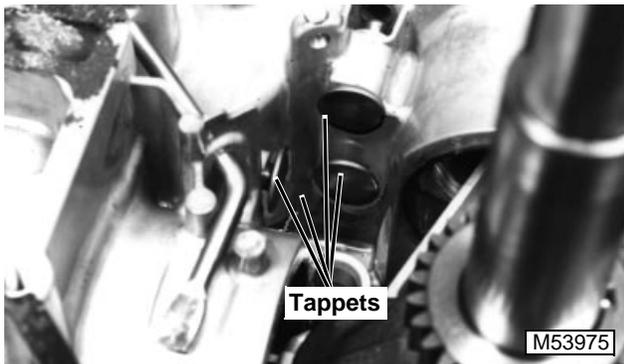
**NOTE:** Mark tappets so they can be installed in their original guides during assembly.
