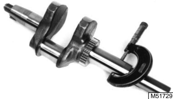
4. Measure main bearing journal diameters. If either journal O.D. is **less than 33.91 mm (1.335 in.)**, replace crankshaft.
