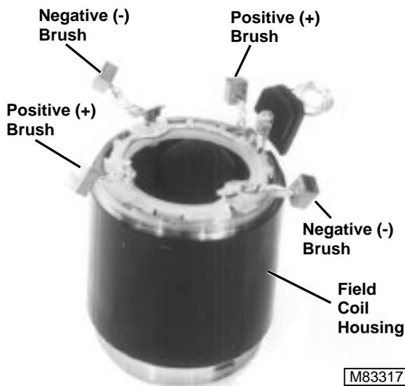
4. Test brush/field coil winding housing assembly:
