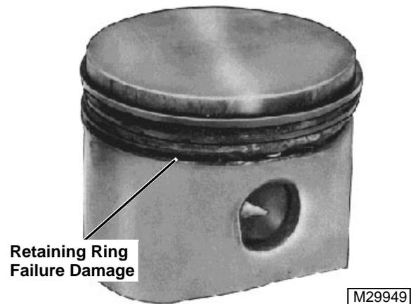
A broken retaining ring caused the damage shown. Retaining rings loosen or break due to:
