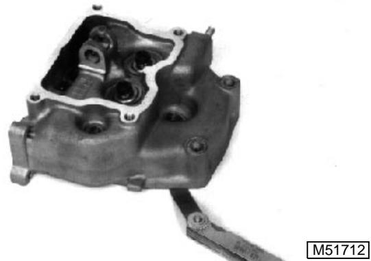
5. Put cylinder head on a surface plate. Check for distortion at several points around the head using a feeler gauge. Replace head if distortion is more than 0.06 mm (0.002 in.).
