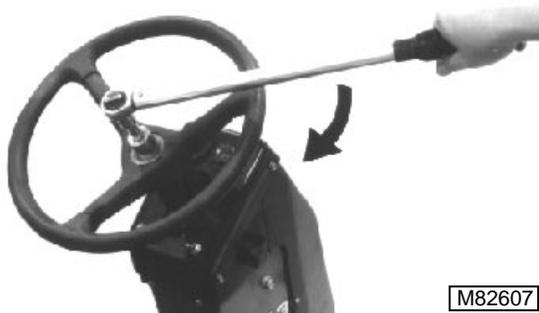
10. With steering wheel in a maximum right position, turn steering wheel to the right with a constant torque of **6.8 N•m (72 lb-in.)**.
