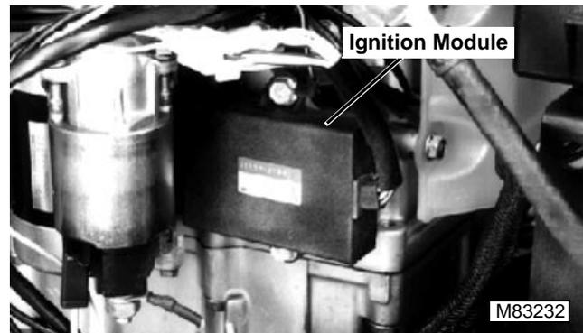
8. The ignition module is very sensitive to the type of ohmmeter used to check resistance. Due to variations in ohmmeters, the best way to determine if the ignition module is good is to replace the questionable module with a known good module.
