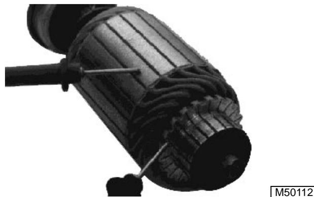
Test for grounded windings using an ohmmeter.
