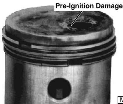
Pre-ignition is the igniting of the fuel-air mixture prior to regular ignition spark. Pre-ignition causes shock, resulting in pings, vibration, detonation and power loss. Severe damage to piston, rings and valves result from pre-ignition.
