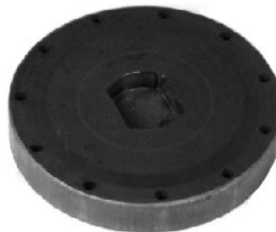
30. Lift the rotor and stator drive plate.
