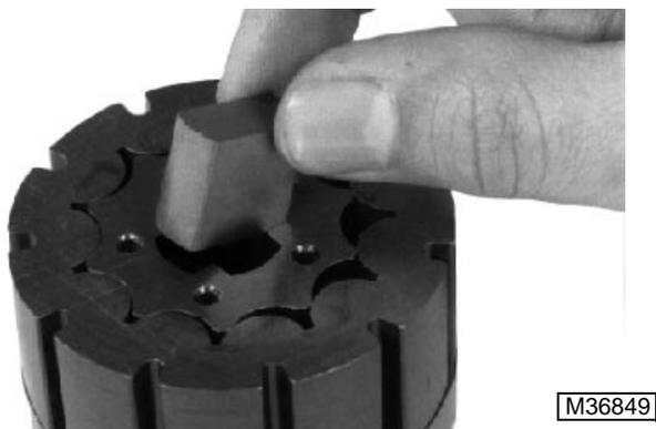
27. Remove drive link spacer. Check spacer for grooves, wear, or damage.
