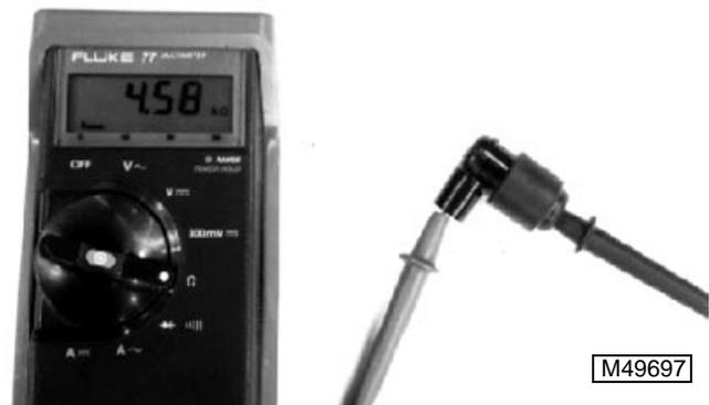
8. Connect one ohmmeter lead to spark plug side of spark plug cap.
