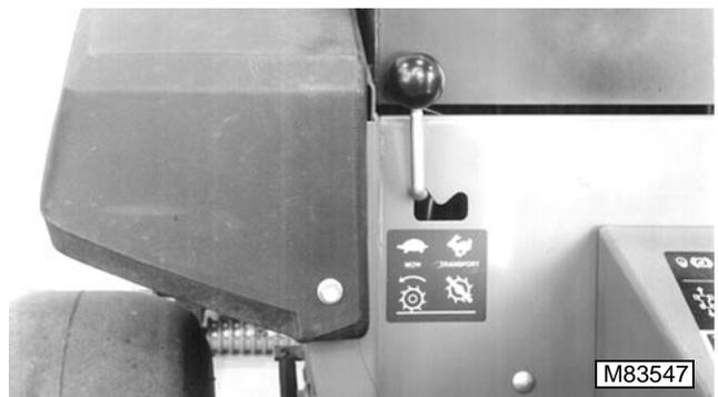
1. Move mow/transport lever to MOW position .
