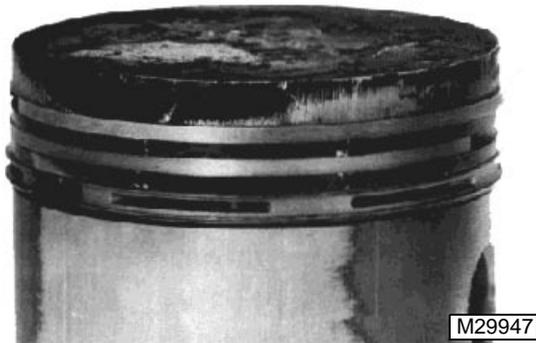
The following is a list of possible causes for detonation.
