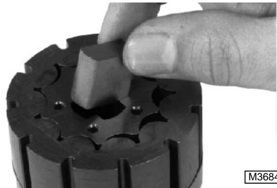
15. Apply multipurpose grease to spacer.
