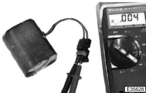
8. Using an ohmmeter or continuity tester, check if continuity exists between terminals. Replace coil if continuity is not present.
