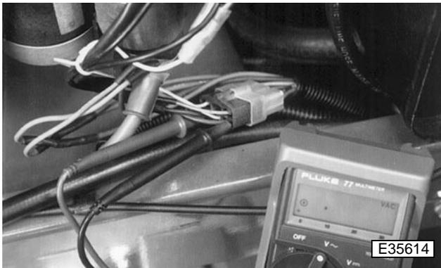
7. Disconnect two pin connector from stator.
