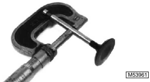
4. Measure outside diameter of valve stem. Replace valve if diameter is **less than specifications**.
