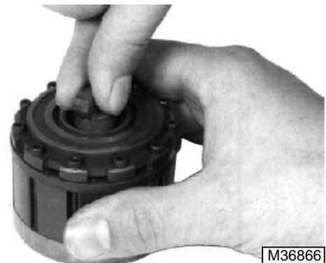
28. Install LARGE end of drive link into the slot in the rotor. Hold the drive link and rotate the metering assembly by hand. The rotor should turn freely inside the stator. If the rotor binds or does not move, disassemble and inspect to find the cause.
