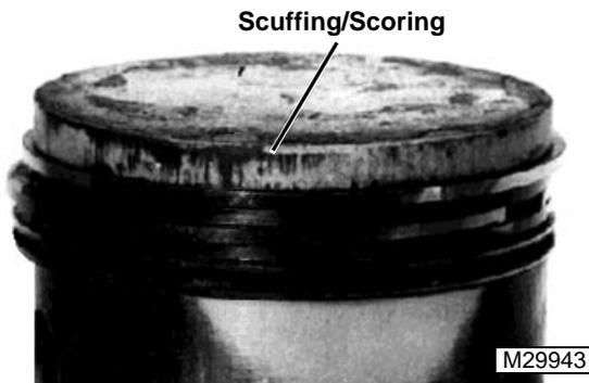
Light scuffing or scoring of both rings and piston occurs when unusually high friction and combustion temperatures approaching the melting point of the piston.
