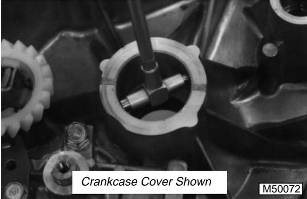
6. Measure crankshaft main bearing diameter in crankcase and crankcase cover. Replace cover or bushing in crankcase if diameter is **greater than 34.07 mm (1.341 in.)**.
