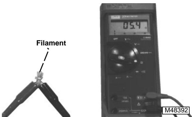
2. Check visually for broken filament.
