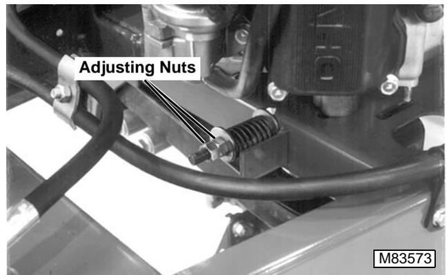
13. Loosen four engine cap screws and nut and belt tension adjusting nuts. Engine should be free to move back and forth, but not tip. Move engine as far forward as possible.
