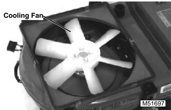
2. Remove four cap screws and cooling fan.
