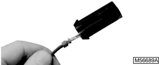
6. Push contact into new connector body until fully seated.
