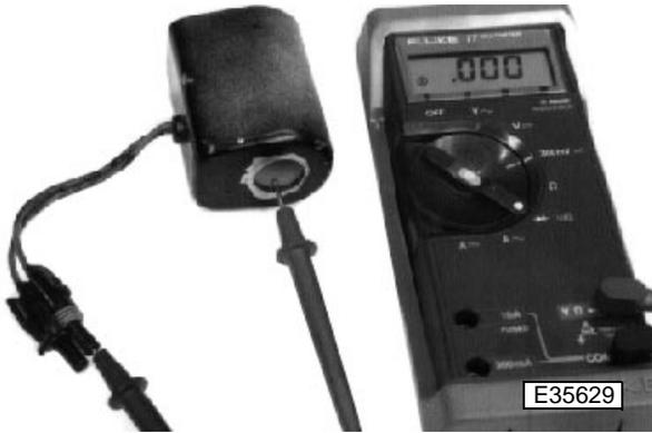
9. Check for grounds or shorts by connecting tester to one coil terminal and the other to bare metal of coil case.
