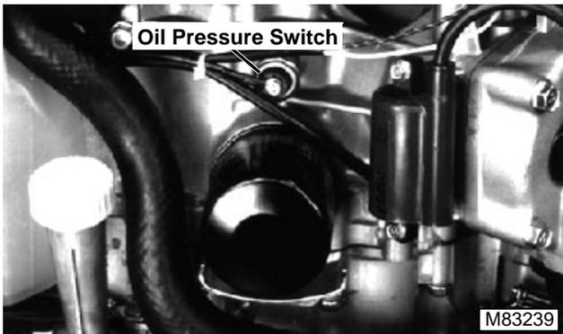
8. Disconnect wire from oil pressure switch.
