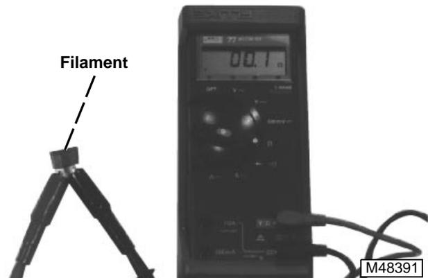
2. Check visually for broken filament.
