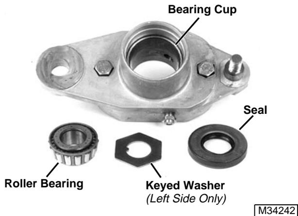
1. Remove seals, tapered roller bearings and keyed washer (left side only) from pivot arms.
