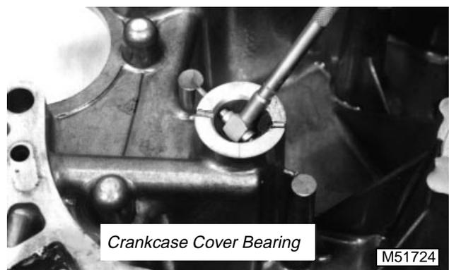
4. Measure camshaft bearings in cylinder block and crankcase cover. Replace block or cover if either diameter is **greater than 16.07 mm (0.633 in.)**.
