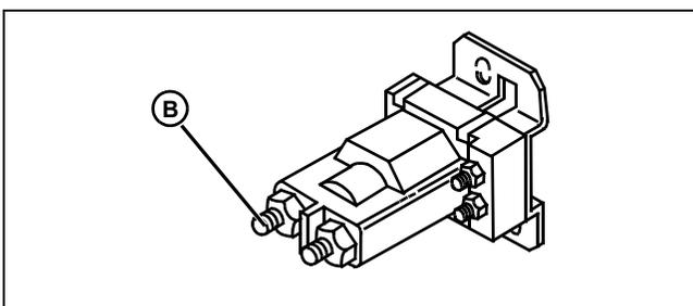
(1) Is there a minimum 14.4  $\pm$ 0.5 VDC at the starter solenoid 230 Red wire connector (B)?
