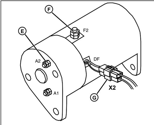
**(4) Is there greater than 0 volts and less than 0.2 volts at the starting motor/generator A2 160 Blk wire connector (E)?**
