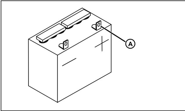
(1) Is there 11.8 to 13.2 volts at the battery positive terminal (A)?
