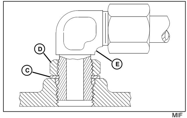
3. For angle fittings, loosen special nut (D) and push special washer (C) against threads so O-ring can be installed into the groove of fitting.
