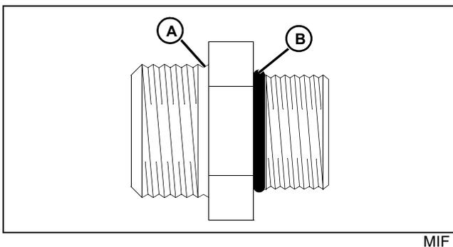
2. Put hydraulic oil or petroleum jelly on the O-ring (B). Place electrical tape over the threads to protect O-ring from
