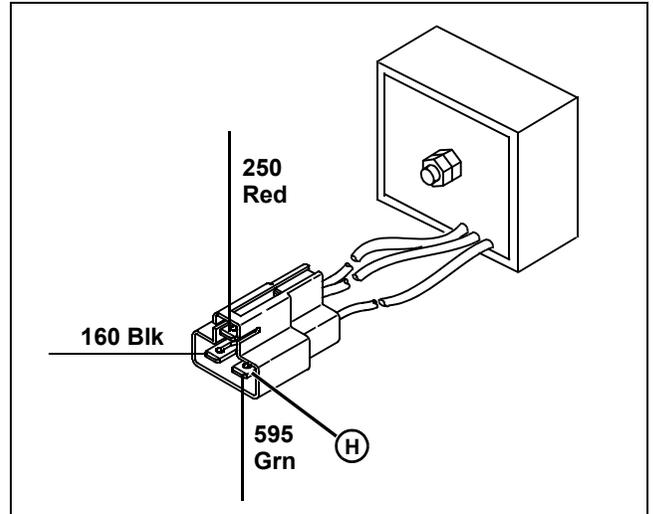
**(6) Is there greater than 0 volts and less than 12.0 volts at the voltage regulator 595 Grn wire connector (H)?**
