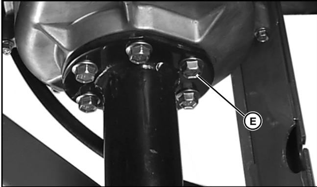
10. Remove six cap screws (E) holding axle tube(s) to transaxle.
