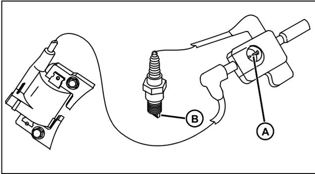
(1) Is there a hot blue spark in the spark tester (A)?
