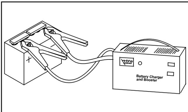
6. Connect variable rate charger to battery.
