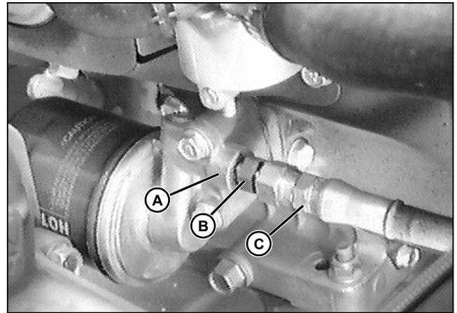
5. Remove plug from filter housing (A).
