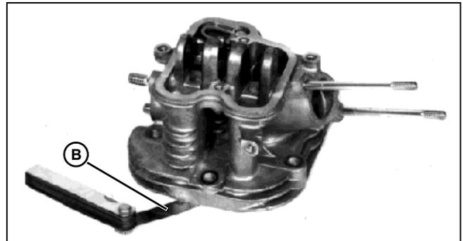
3. Put head on a surface plate. Check for distortion at several points around head with feeler gauge (B). If distortion greater than 0.05 mm (0.002 in.), replace.
