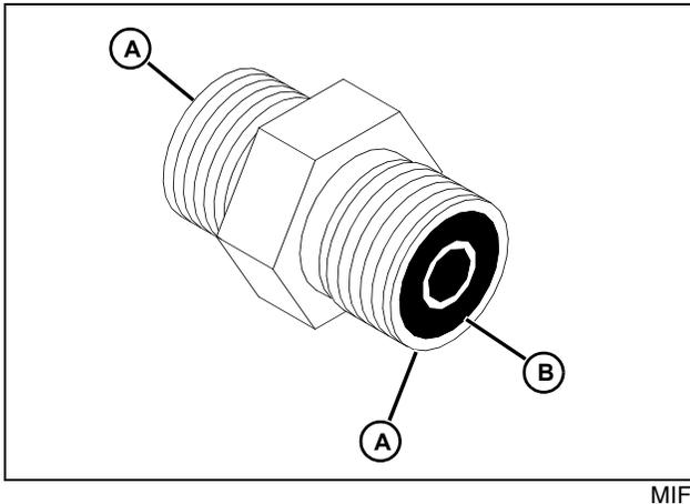
1. Inspect the fitting sealing surfaces (A). They must be free of dirt or defects.
