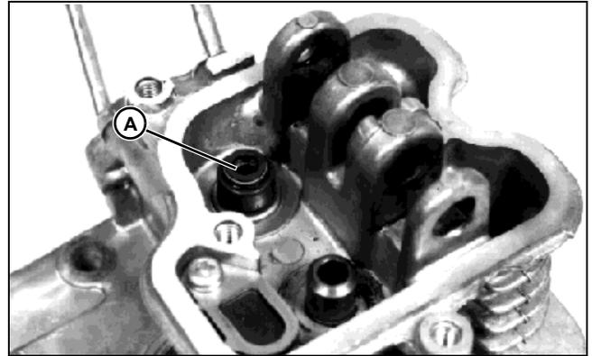
1. Inspect stem seal (A) for wear or damage. Remove stem seal using a screwdriver.
