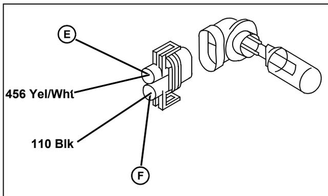
**(5) Is there battery voltage at RH headlight 456 Yel/Wht wire (C)?**
