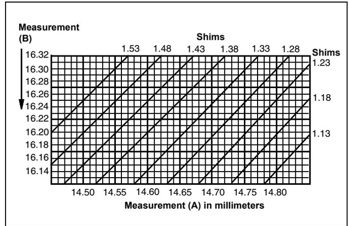
4. Locate measurements on appropriate table. Follow lines to where recorded measurements intersect. Choose the next smaller shim from the table.
