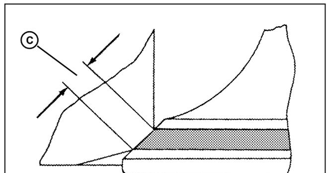
4. Measure valve seat width. Inspect valve seat for wear or damage. If valve seat width is not within 0.50 - 1.10 mm (0.020 - 0.043 in.) (C), recondition valve seats.
