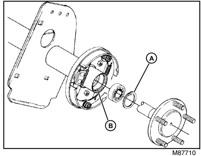
2. Using right angle compression ring pliers, remove C-clip (A) from groove (B) in axle housing.
