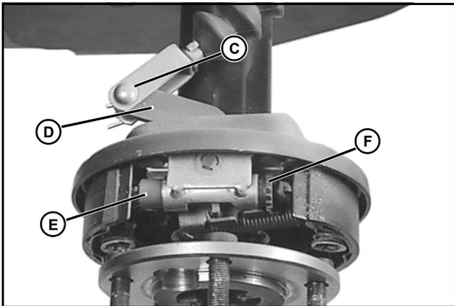
4. Remove clevis pin (C).
