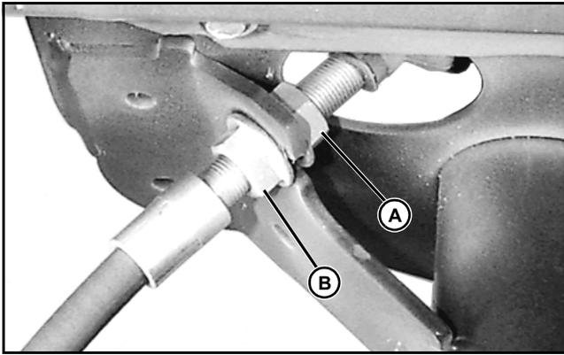
3. Loosen flange nuts (A) and (B) on rear brake cable housing.
