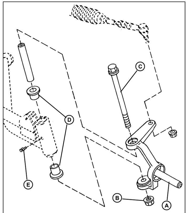
3. Disconnect tie rod end from spindle shaft (A).
