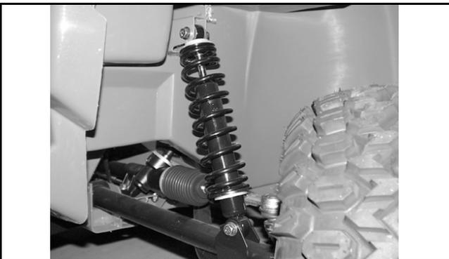
Standard Shock Absorber Mounting (New Style)
