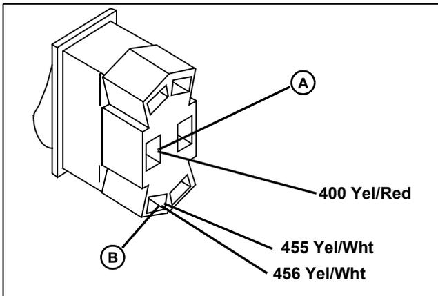
(1) Is there battery voltage at the headlight switch 400 Yel/Red wire (A)?
