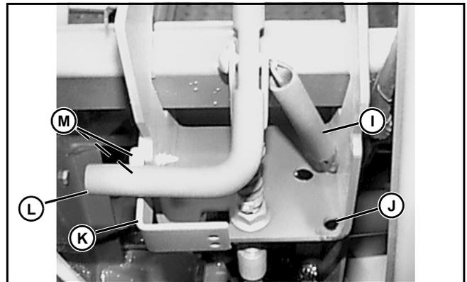
1. Loosen screws (M) of stop plate (K). Adjust stop plate up to reduce amount of freeplay in brake pedal. Apply only enough up force to stop plate to take up freeplay. Do not start actuating brake. There should be maximum freeplay travel of 4 mm (0.16 in.).
