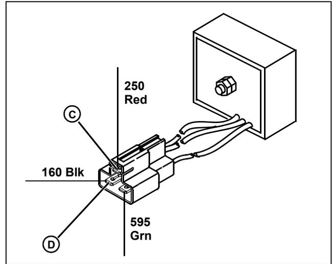
(2) Is there a minimum 14.4  $\pm$  0.5 VDC at the voltage regulator 230 Red wire connector (C)?
