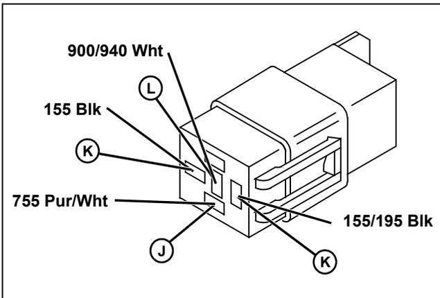
**(9) Is there battery voltage at magneto run relay (J)?**
