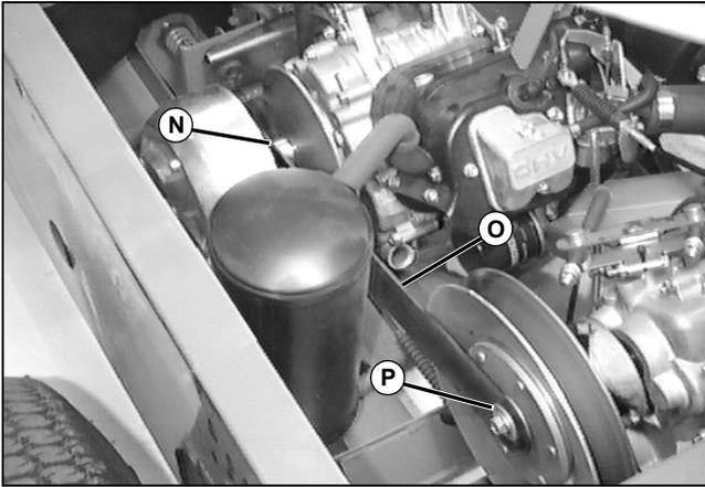
24. Position open end (N) of clutch center distance gauge (O) over the primary clutch shaft.
