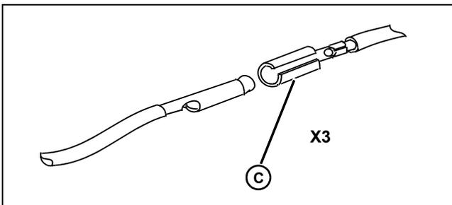
(3) Disconnect engine connector (C). Is there a spark present at tester?
