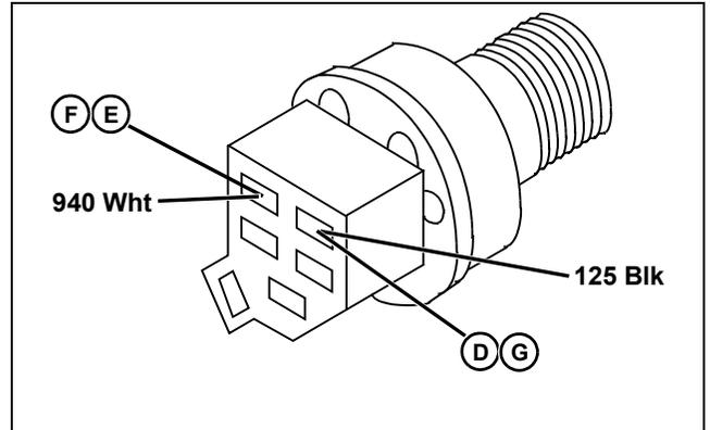
(4) Is there continuity between key switch connector (D) and engine connector, with no continuity to ground?
