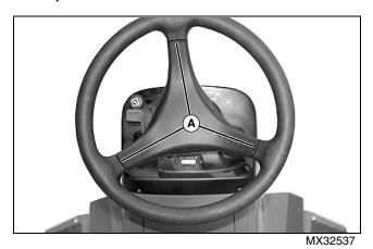
2. Remove cover from steering wheel by gently prying up on center cover at three points (A).
