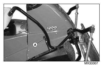
2. Raise blade and secure in transport (lock) position with hold down strap (A), as shown. Place block under blade.
