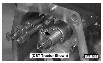
IMPORTANT: Be sure PTO collar is in place on shaft or in end of PTO clutch before assembling tractor sections. Smaller end of collar goes toward PTO clutch.
