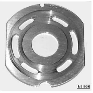
Inspect the bronze side of the valve plate for wear. Replace the valve plate if any wear, scoring, or scratches exist.
