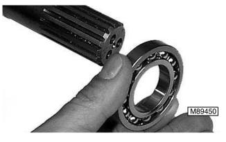
8. Using a knife edge bearing puller, remove bearing from shaft.
