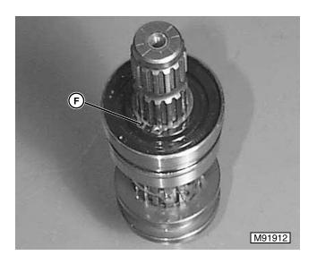
6. Install snap ring (F) onto shaft to retain seal.
