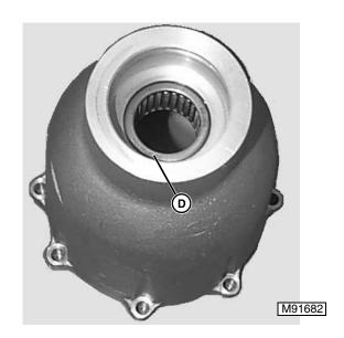
3. The housing bearing (D) should be pressed on the numbered side, from the outside of the housing inward, until the numbered end is recessed 1.78 mm (0.70 in.) into the housing bore.
