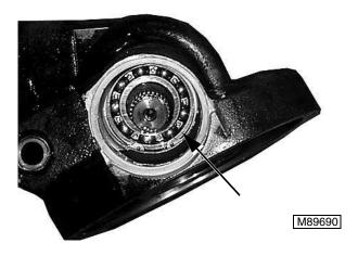
5. Remove the snap ring from the spindle housing.
