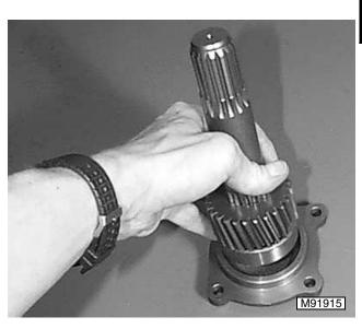
22. Install idler shaft assembly into cover.
