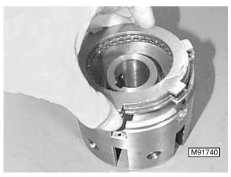
Assemble brake pack starting with a plate, followed by a disk, followed by a plate, disk, plate. Install into clutch cylinder.
