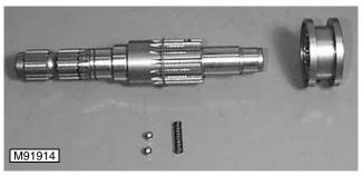
20. Remove shift collar, two steel balls, and spring.
