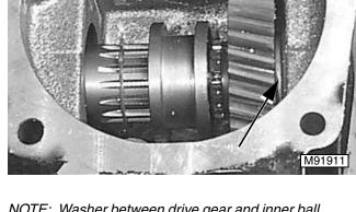
NOTE: Washer between drive gear and inner ball bearing may fall out when PTO stub shaft is removed.
