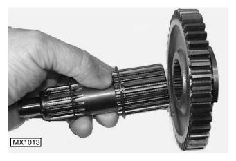
6. Slide 41T gear from stub shaft. Inspect all parts for wear or damage. replace as required.
