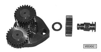
Remove washer, gear, bearing, and washer from planetary pinion shaft. Inspect components for damage. Replace as required.
