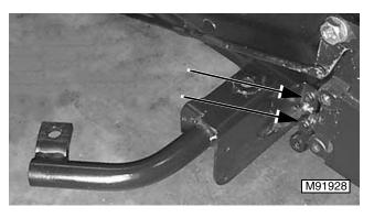
34. Remove two cap screws and RH operator's platform support.
