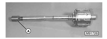
1. If necessary, remove splined coupling (A) from end of shaft.
