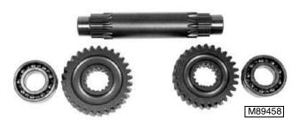
IMPORTANT: DO NOT spin bearings using compressed air. Damage to bearing balls, cage and races could result.
