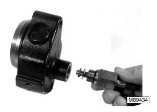
5. Remove rate of drop control valve from cover.
