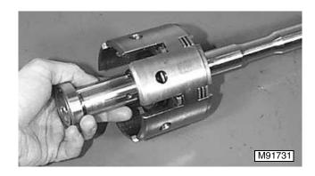
10. Install clutch cylinder onto PTO shaft.
