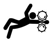
Tie long hair behind your head. Do not wear a necktie, scarf, loose clothing, or necklace when you work near machine tools or moving parts. If these items were to get caught, severe injury could result.
