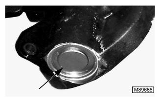
1. Carefully remove the spindle cap from the housing.
