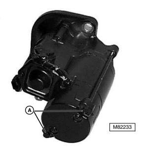
Remove field wire and (2) motor-to-clutch housing cap screws (A).
