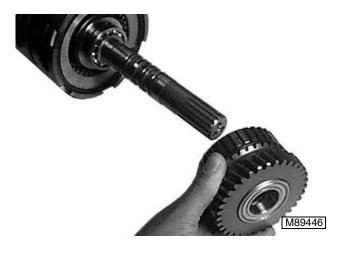
5. Remove clutch gear-33T and bearing from shaft.
