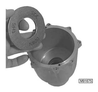
4. Apply some petroleum jelly to the "THIS SIDE DOWN" side of the cam washer before installing into motor housing so it will stay in place while installing rotating assembly.
