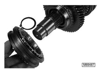
5. Remove synchromesh gears and shift collar as an assembly.
