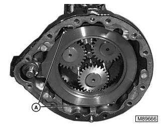
3. Remove the springs (A) that retain the brake plate in the rear axle housing.
