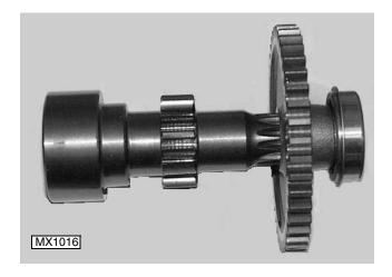
5. Assemble connecting shaft with 42T gear and bearing as shown.
