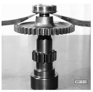
4. Pry or press bearing off of connecting shaft.
