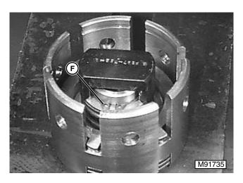
Use JDG1169 Clutch Spring Compressor, and a press to compress clutch spring. Install external snap ring (F).
