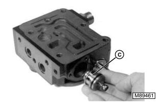
3. Thread one of the cover cap screws into threads on end of piston (C) and use as a puller to remove piston from valve body. Replace O-ring on piston.
