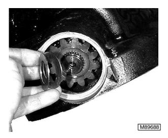
3. Remove the washer, shim, and bevel gear from the spindle shaft. Save any shim(s) from between the spacer and the bevel gear.
