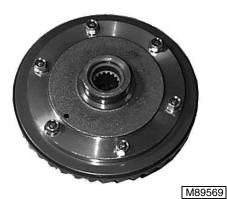
7. Remove six screws (46-4700), or twelve cap screws (4500), and lock washers securing ring gear to differential housing. Remove ring gear.
