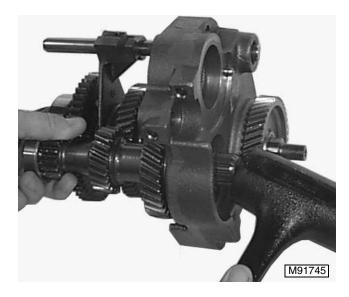
8. Tap gear reduction assembly out of bearing housing with plastic hammer.
