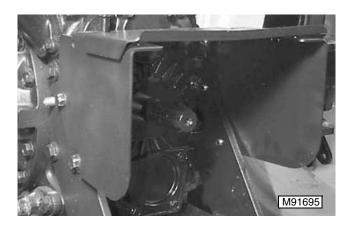
3. Remove four cap screws and rear PTO shield assembly.
