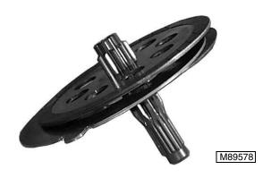
1. Assemble two brake disks and one brake plate on short left hand pinion.
