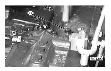
4. Remove three cap screws (B) securing SCV to PTO clutch valve. Remove SCV.
