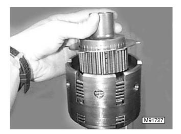
3. Remove clutch hub and retaining plate from clutch cylinder.
