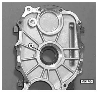
17. Using a seal puller or suitable driver, remove seal (H) from rear PTO cover.
