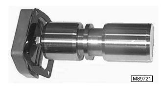
NOTE: The piston is larger than the opening in the gasket, so the gasket must be placed between the piston and the cover before installation of the piston and cover assembly.
