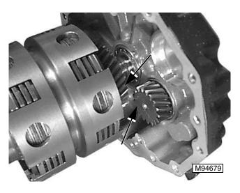
Slide PRT clutch and shaft assembly into front cover until the clutch gear 33T and idler gear 17T almost engage.
