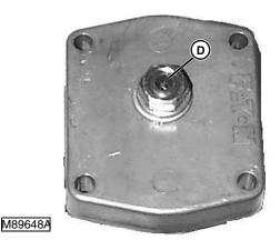
NOTE: The adjustment of the servo motor is performed by loosening jam nut and adjusting screw (D) inside the tunnel with special tools as shown below.
