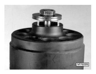
3. Place one of the flat washers over the 3/8 x 5 inch cap screw. Install cap screw through spline end of piston block so that the washer rests on the three pins.
