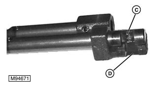
5. Inspect slot in fork shaft (C) and main shifter (D) for wear or damage. Replace worn parts as required.
