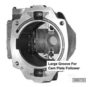
12. Place the cam plate into the housing. Make certain the cam plate follower is correctly positioned in the servo piston groove.
