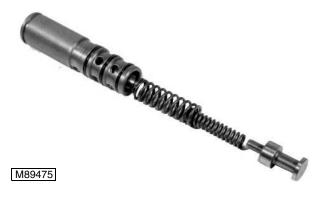
Remove piston and two springs from bore of delay relief valve.
