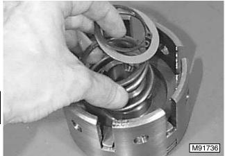
5. Place spring, washer, and snap ring onto center of piston.
