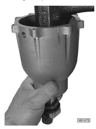
2. Gently tap the shaft with a plastic hammer as shown until the rubber seal releases from the housing.
