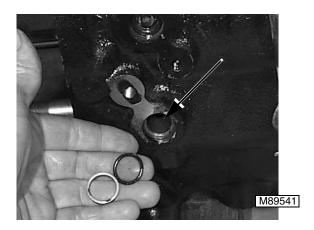
16. Remove O-ring and sleeve from shift shaft hole. Replace O-ring before reassembly.
