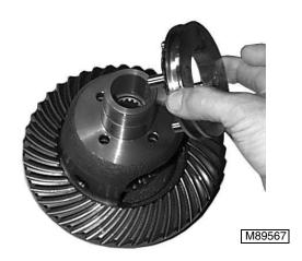
3. Remove differential lock collar from differential.
