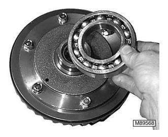
4. Remove bearing from carrier side of differential.
