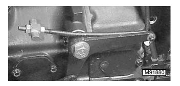
33. If not already removed, lay upper brake rods across bellcrank pivot to prevent them from becoming damaged when separating tractor sections.
