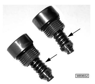
NOTE: The relief valves are dual purpose. The valves contain two springs. The strong spring is a 6000 psi relief valve. There is also a weak spring inside the head that operates a check valve function when the other circuit is being used. There are no serviceable parts in the valve and they cannot be adjusted. If any malfunction is suspected, replace the relief valve.
