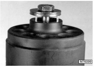
11. Place one of the flat washers over the 3/8 x 5 in. cap screw. Install cap screw through spline end of piston block so that the washer rests on the three pins.
