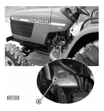
4. Locate rubber plug (B) on tunnel and remove plug.
