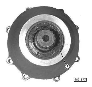
1. Remove the large retaining ring (F) from the housing at the output end of the shaft.
