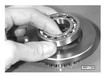
16. Install bearing into brake hub.
