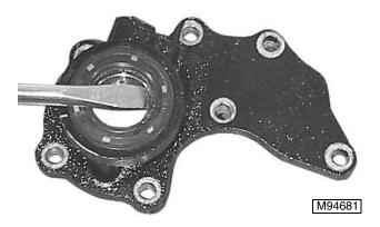
4. Remove seal, sleeve and snap ring from reverse case.
