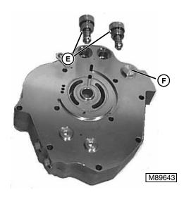
6. Mark the forward and reverse relief valves (E) as to which cavity they came from for reassembly purposes. Remove the relief valves from the backplate. Check for damaged springs or seats.
