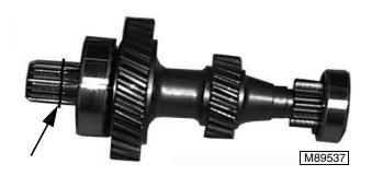
Remove external snap ring from end of gear reduction assembly.
