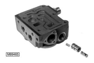
Remove piston, spool, and spring from PTO valve block.
