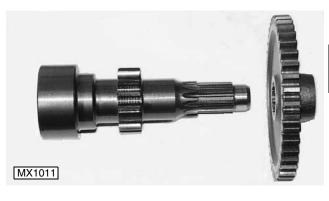
5. Slide 42T gear from shaft. Inspect all parts for wear or damage. Replace as required.
