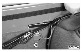
10. Disconnect Brn ground wire (G) from panel behind cab seat. Cut all tie straps as needed to free the ground wire for cab removal.
