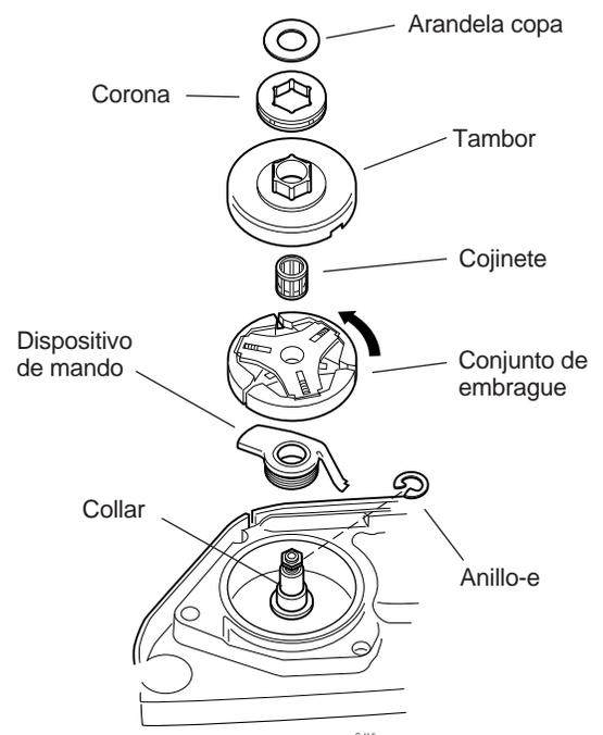
Figura 6.25 757 Clutch Assembly Installation
