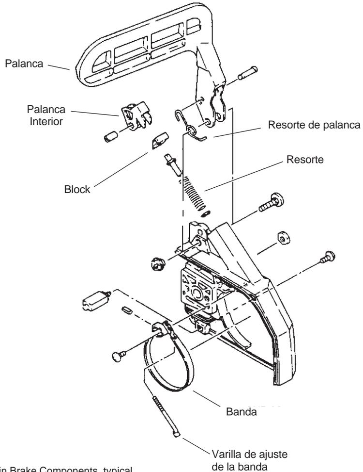
**Figura 10.5** Chain Brake Components, typical
