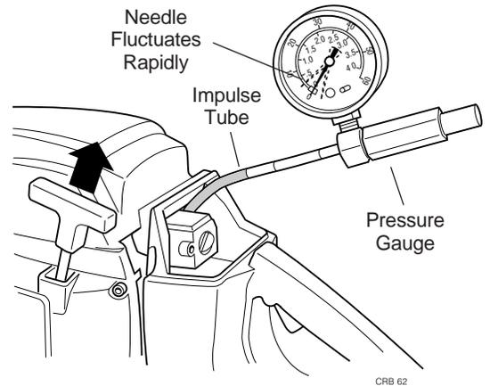
Figura 2.14 Testing Impulse Passage (488 and larger)
