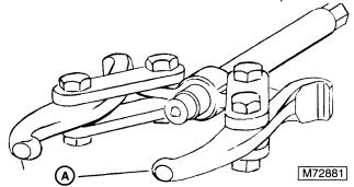
20. Use a modified two-jaw bearing puller, pulling against the two notches machined in the housing to remove the charge pump assembly.
