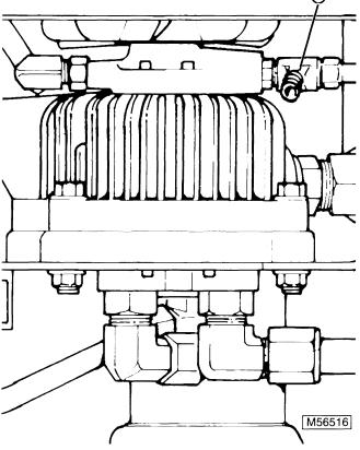
2. Disconnect the charge pump pressure hose and install a "T" fitting (A) and a direct reading pressure gauge.
