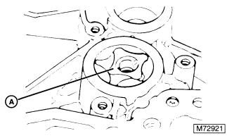
Check the clearance (A) between the inner and outer rotor with a feeler gauge. Measure the clearance between the high point of the inner rotor and the high point of the outer rotor. If the measurement exceeds the service limit, replace both rotors as a set.
