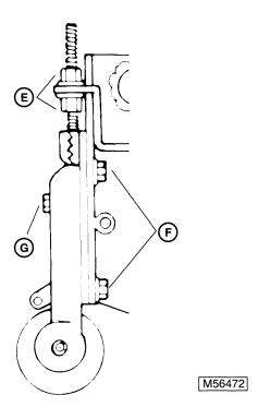
NOTE: To avoid binding the adjustment mechanisms, make small adjustments on each end of the roller.
