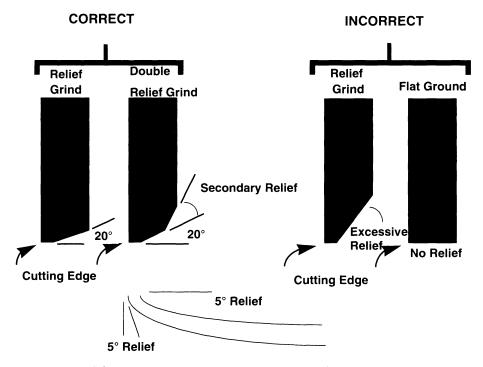
John Deere recommends Relief Grinding the reels before spingrinding for these reasons:
