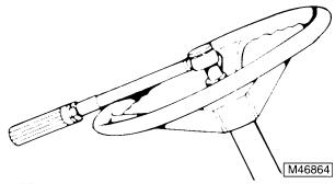
3. With steering wheel at a maximum right turn position, apply a constant torque of 6.8 N•m (72 lb-in.) and count the number of rotations occurring in one minute.
