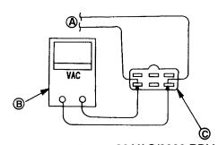
Unregulated Stator Output, 26 VAC/3000 RPM
