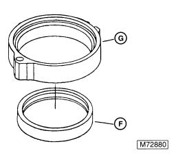
NOTE: The pump race (F) is press fit in the cam ring (G) and will require a press to remove it. The cam ring and pump race are available as an assembly.
