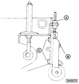
1. If HOC range needs to be changed, loosen nut (A). Remove nut and washer (B) and two bolts (C) (per side) and position the carriage bolt for the cutting height range.
