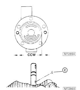
46. Lubricate carrier drive pin (C) and install in keyway of input shaft
