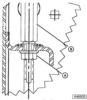
1. The lower adjusting nut (A) will lower the reel when turned counterclockwise and the upper adjusting nut (B) will raise the reel when turned clockwise. (as viewed from the top of the unit looking down).
