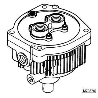
IMPORTANT: Clean the pump exterior thoroughly before disassembly to prevent foreign material from entering the inner passages while repairing the pump.
