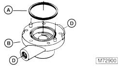
50. Lightly lubricate new square cut seal (A) and install in seal groove of pump housing (B).
