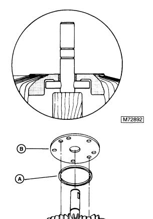
44. Lightly lubricate new square cut seal (A) and install in seal groove in cover
