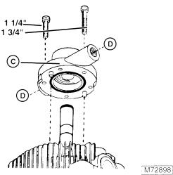
51. Align charge pump dowel pins with holes in cover. Protect oil seal lip from keyways, snap-ring grooves and shaft splines. Then guide pump over shaft, carrier and rolls until pins engage holes.
