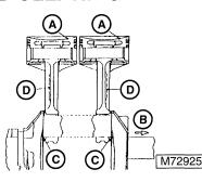
IMPORTANT: Note location of the arrow match mark on the piston head in relation to made in japan on the connecting rod. no. 1 piston is opposite no.2. Keep parts together as a set.
