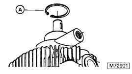
56. Install large snap-ring used to retain bearing in housing.
