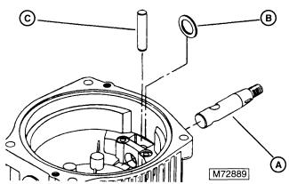
39. Install new control shalt (A) and washer (b) in cover.
