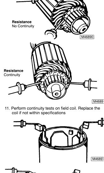
IMPORTANT: The coil frame is a tie point for 12 separate field coils. It may be difficult to detect one bad coil. If rpm was slow and armature tests are normal, replace the field coil assembly.
