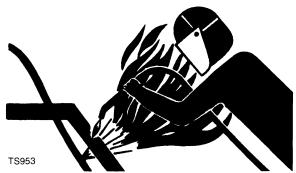
Flammable spray can be generated by heating near pressurized fluid lines, resulting in severe burns to yourself and bystanders. Do not heat by welding, soldering, or using a torch near pressurized fluid lines or other flammable materials. Pressurized lines can be accidentally cut when heat goes beyond the immediate flame area.
