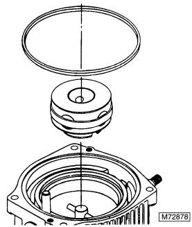
59. Align the slot in the pump rotor with input shaft cross pin. Install rotor assembly on shaft
