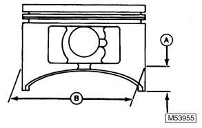
7. Measure the outside diameter (B) of the piston 11 mm (0.43 in.) (A) up from the bottom of the piston at a right angle to the direction of the piston pin hole. If the measurement is less than the service limit, replace the piston.
