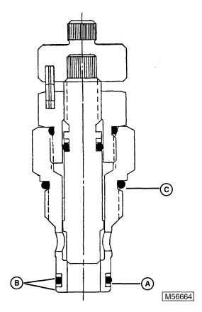
6. Ensure o-ring (A) is installed between back-up washers (B). Install o-ring (C). Lubricate o-rings and back-up washers before installing flow control valve.
