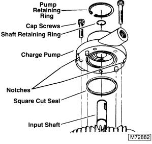
21. Remove the square cut seal from the pump assembly.
