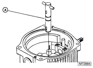
43. Turn cover over. Support input shaft from underneath. Use a piece of steel bar stock or hard wood 2" in diameter by at least 2 1/2" long to keep the shaft cross pin against the cover.
