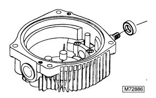
IMPORTANT: Be careful not to damage the inner portion of the oil seal. Excessive pressing or driving of the oil seal will damage the rubber portion of the oil seal.
