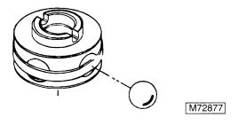
NOTE: Each ball must be replaced in the same bore from which it was removed. Use a suitable container for piston ball storage such as an egg carton or ice cube tray.
