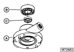
22. Remove the bearing (B) and oil seal (C) from the charge pump (A). Discard the oil seal.
