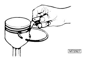
6. Measure the top and second ring groove clearance by inserting a new piston ring in the groove at several locations and measuring the gap between the ring and the ring land with a thickness gauge. Replace the piston if the gap exceeds the service limit.
