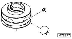
3. The pump ball piston assembly must remain intact as the ball pistons are matched to the pump rotor. Use a wide rubber band (A) to retain the ball pistons in place during handling.
