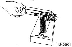
6. Locate shorts by rotating the armature on the growler while holding a thin metal strip (e.g., hacksaw blade) on top of the armature. If there is a short in the windings, the metal strip will vibrate at the point where the short exists.
