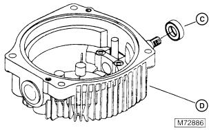
33. Use a sharp, narrow edged tool to pierce the top metal part of the oil seal (C) and remove seal from the cover (D)
