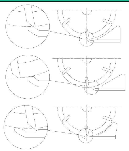
The bedknife position has a specific wear pattern as the reel blade sweeps over the bedknife, and the wear angle depends on the position and attitude of the knife. The pictures above illustrate the three primary positions of the bedknife cutting edge in relation to the centreline of the reel: even, behind or forward of the centreline.
