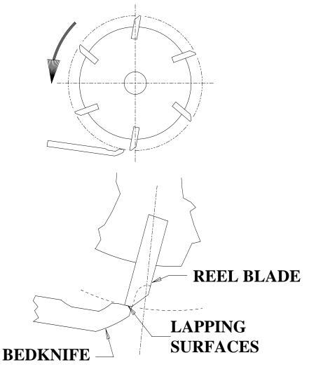
The correct procedure for backlapping will be to make light contact between the reel and the bedknife. The grit of the compound will pass between the top part of the bedknife that lies in the blade path and the surface width of the reel blade. This can be effective in bringing the cutting edges back to "square". When the cutting edges are rounded off too much, it will take much longer to remove enough metal to get to a "square" edge, and there can be greater wear on the bedknife.
