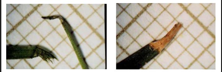
These two photos illustrate what you would like to minimize, as studies have shown the cutting process will always damage the turf to a certain degree. This type of damage can happen whether the reel is sharp or dull, but will always be most prevalent with dull and/or misadjusted reels.
