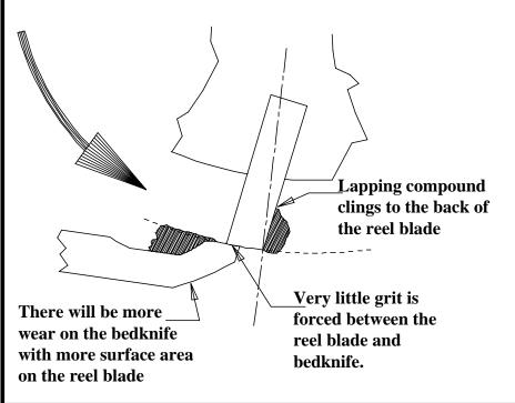
On a flat ground or worn reel, there is so much surface area and metal to remove on the reel blade that it makes the lapping process ineffective and time consuming. This will also cause excess wear to the bedknife and will induce more stress time on the drive systems.
