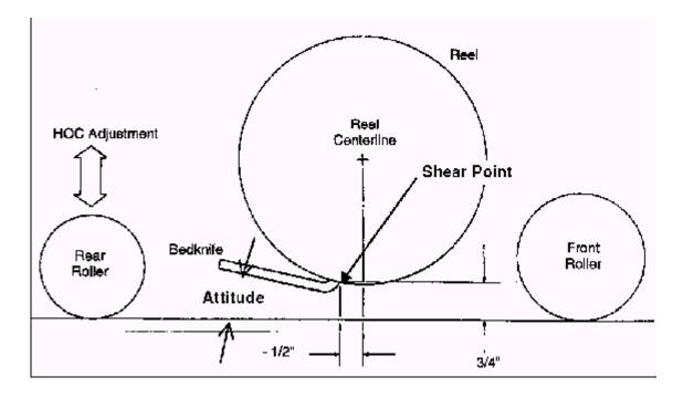
WHAT EXACTLY IS "ATTITUDE'? The cutting unit "attitude" is the angle between the bottom of the bedknife and the ground under the cutting unit. As the bedknife attitude is changed, it is important to note that the reel to bedknife shear point changes relative to the center line of the reel. This can change the after cut appearance of the grass. The result may be better or worse depending on several factors.
