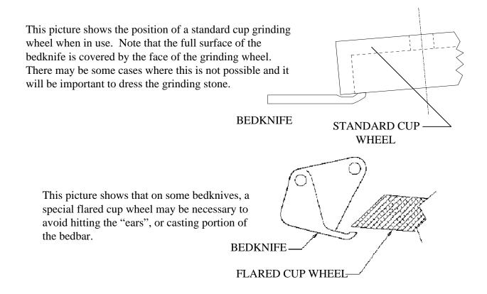
Dressing the grinding wheel is important to the quality of grind. A grinding wheel which is loaded will cause excessive heat build up and can cause an irregular grind. The best dressing method is a diamond dresser rigidly mounted in relation to the grinding wheel. Other methods which can be used are hand held diamond dressers and hand held dressing bricks. Hand held dressers are difficult to use and makes it more difficult to achieve an accurate wheel dressing.
