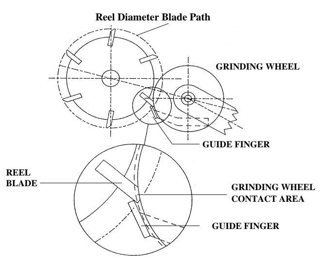
These pictures demonstrate how a reel is set up on a single blade grinder to achieve the desired angle on the edge of the blade. The grinding wheel turns and the reel does not as each reel blade is ground separately. The height of the grinding wheel will dictate the angle on the reel blade, as the reel blade rests on the guide finger.
