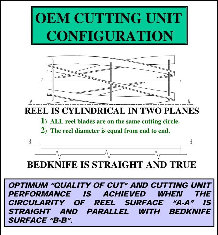
Total tolerance between reel and bedknife can only be +.002/-.001 to provide a quality reel to bedknife clearance that does not require backlapping.
