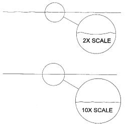
To mow roughs, the top surface can be wavy. Therefore, a 5-bladed reel at lower RPM is acceptable and a close up view might look like this picture at 2X.
