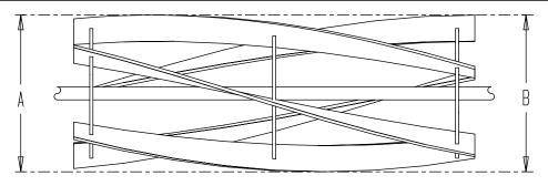
If diameters A and B are equal, the reel is CYLINDRICAL.
