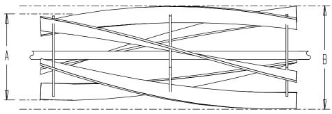
If diameters A and B are not equal, the reel is CONICAL.
