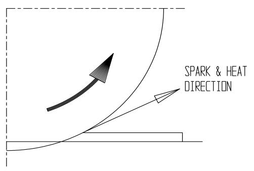
You would like to have the rotation of the grinding wheel to send the sparks away from the cutting edge of the rotary blade. This can help minimize the heat build up that occurs at the very tip, preventing it from losing the hardness, or temper, of the blade.
