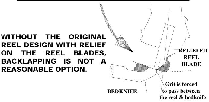
**REASON:** The relief area on the reel blade provides a landing area for the lapping compound to adhere to. This enables the grit to be suspended on the reliefed area and is pushed between the reel and the bedknife, thus "effectively" removing metal.
