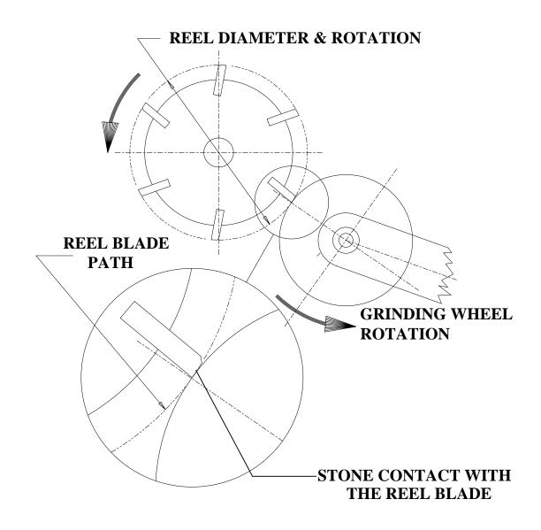
This picture shows how the edge of a reel blade is ground on spin grinders to achieve a sharp edge. Note that both the reel and the grinding wheel rotate in the same direction, causing opposite directional contact at the grind point. This will yield a better grind performance in producing a sharp edge.
