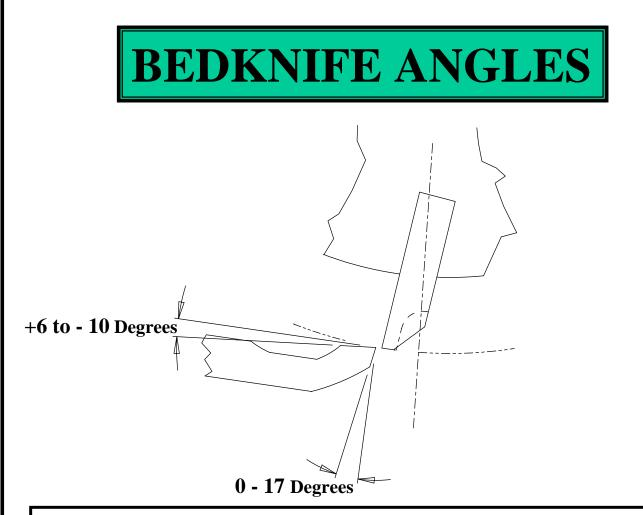
All bedknife angles are based on the bottom surface of the bedknife. These values are industry averages - for the correct angles of specific models, refer to the mower manufacturers specifications.
