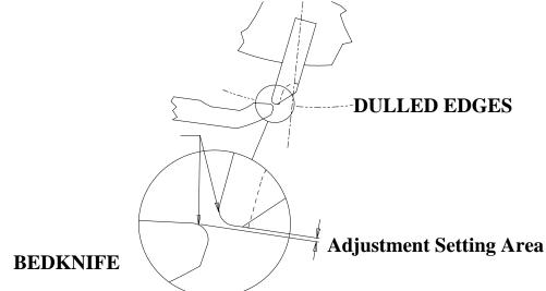
A microscopic review of the reel and bedknife reveals that it takes only SIX to TEN HOURS of operation for a crisp sharp edge to begin to round off. This can result in a widening of the gap between the cutting edges when the machine is through cutting for the day.
