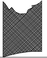
A concave grind as illustrated above does not occur with any grinding traverse system that was tested.
