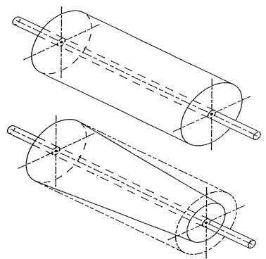
Even reels that are properly adjusted can start to lose their cylindrical shapes and become coned or tapered. As the "relief" wears away through the season and more surface of the reel blade passes the bedknife, the adjustments may accentuate inaccurate wear patterns.
