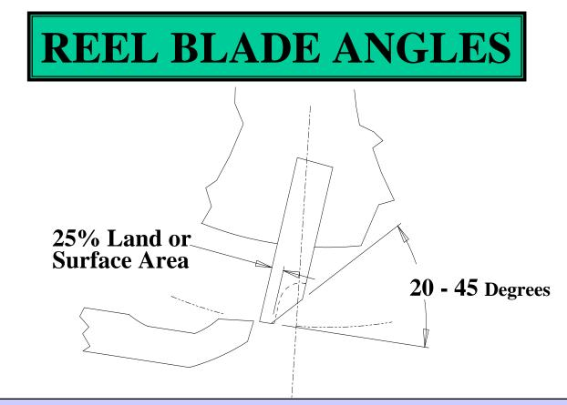
Reel blades have a back "RELIEF ANGLE" where approximately 75% of the blade is removed. The OEM reel blade configuration has two basic process designs :
