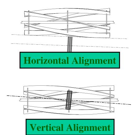
On some reels, the window of adjustment allowing for taper is relatively small. Taking time to properly grind a true cylinder will minimize the potential for problems, including adjustment issues, quality of cut issues, or "aftercut" appearance issues.
