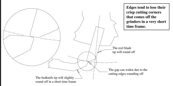
You will never attain the sharpness that comes off a grinder through adjustments, but advocates of the light contact process indicate that the rubbing of the two parts will allow for adjustments to be more effective for a longer time frame.
