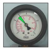
Pressure specification: Pressurize to 0.5 bar (7 psi). Leakage to 0.3 bar (4 psi) in 20 seconds is acceptable.
