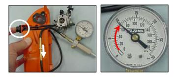
Step 3: Attach tester to primer return hose. Push primer bulb; gauge should indicate pressure and hold. If not, purge primer is faulty.
