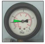
Vacuum specification: Apply vacuum of -0.5 bar (-7 psi). Leakage to -0.3 bar (-4 psi) in 20 seconds is acceptable.
