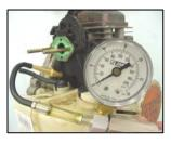
Connect carburetor tester to impulse hose while performing pressure and vacuum tests. Gauge should move while performing tests. 14. Perform carburetor check-shafted products:
