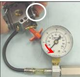
Step 1: Attach tester to fuel line fitting. Pressurize carburetor to 10 psi (0.7 bar). If pressure holds, the fuel pump components and inlet needle are sealing. Go to step 2.
