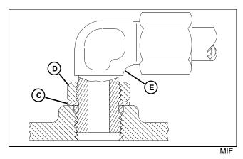
3. For angle fittings, loosen special nut (D) and push special washer (C) against threads so O-ring can be installed into the groove of fitting.
