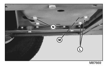
15.Remove two cap screws (L) and strap (M) with pal nuts from front of engine.
