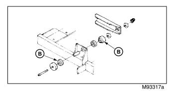
3. Remove snubber isolators (B) and hardware.
