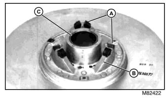
2. Inspect bushing (C) for wear or damage. Replace movable sheave if necessary.
