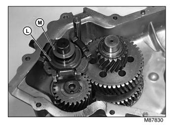
11.Install actuating sleeve assembly (L), with thrust washer end outward, and shim (M) on input shaft.
