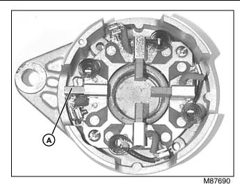
3. Hold each brush spring (A) back and slide each brush out so spring is tensioned against brush side instead of brush end.
