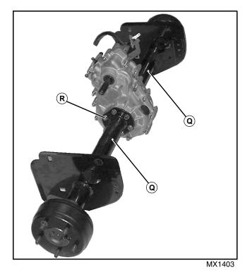
16.Install axle tubes (Q) and cap screws (R) onto transaxle
