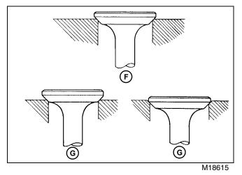
• The valve seating surface should show good contact all the way around (F). If seat does not make proper contact (G), lap valves to seats.
