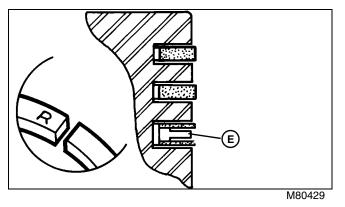
4. Oil ring is an assembly. Install spacer (E), then side rails in bottom ring groove of piston. Put side rail end gaps  $180^{\circ}$  apart.
