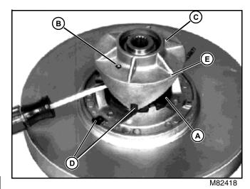
3. Place alignment marks (D) on cam (E) and movable sheave to aid in assembly.
