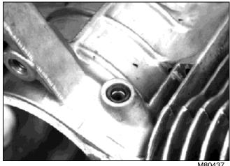
2. Remove worn or damaged seal using a screwdriver. Install seal with lip toward inside of engine using a driver set. Press in seal 1.42 mm (0.056 in.) below flange surface.
