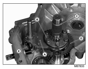
2. Install washer and forward drive gear (D), shift fork (A), gear selector (B) and drive gear shaft (C) with the splined end up. Be careful to keep ball in place when installing shift fork.
