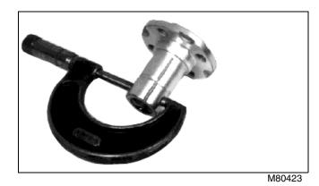
6. Measure support shaft diameter. If shaft OD is less than 25.93 mm (1.021 in.), replace shaft.
