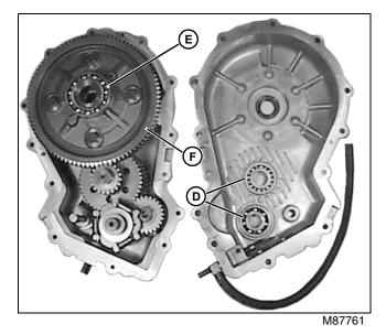
1. Inspect bearings (D). If either bearing is pitted, corroded, discolored or does not rotate freely, replace bearing.
