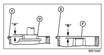
2. With gasket (C) installed on crankcase, measure from gasket surface to crankshaft gear surface (D). Record this measurement as "A".
