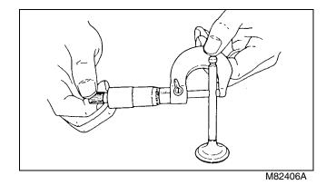
5. Measure valve stem diameter in two directions at right angles, at four different positions. Replace if measurement is less than specifications.
