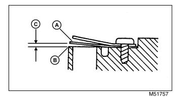
2. Measure air gap between reed valve (A) and valve seat (B) at valve tip. Replace reed valve if gap is greater than 0.20 mm (0.008 in.) (C).
