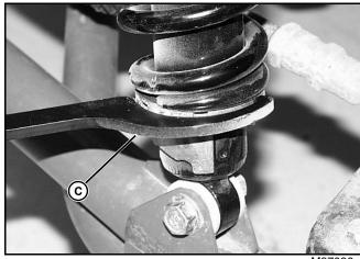
4. Use the adjusting wrench (C) to adjust the shock up to 5 levels of adjustment. Each level of the adjustment is approximately 3 mm (1/8 in.) more spring preload.
