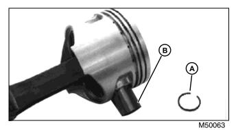
3. Remove circlip (A), piston pin (B) and connecting rod.
