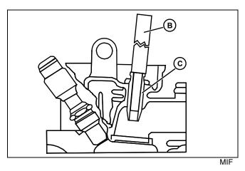
4. Install new bushing with JDG504 Valve Guide Driver. Drive in from top of cylinder head until bottom of groove on outside of guide is even with top of cylinder head.
