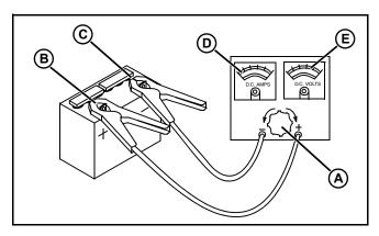
6. Turn load knob (A) counterclockwise to OFF position.
