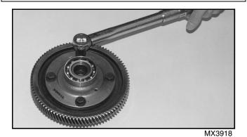
14.Install four cap screws and nuts and tighten with the wrench applied to the bolt head to  $80 \pm 5$  N•m (59 ± 4 lb-ft).
