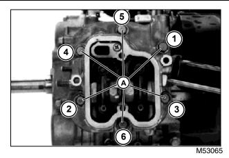
2. Install cap screws (M8 x 45) (A), and tighten finger tight.
