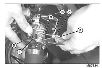
5. Loosen jam nuts (B and C).
