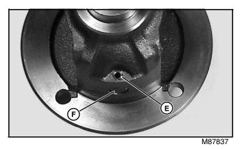
3. Using a drift punch, drive rolled pin (E) far enough through differential housing to allow cross shaft (F) to be removed.
