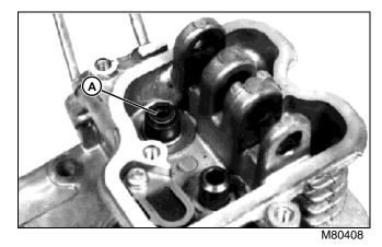
1. Inspect stem seal (A) for wear or damage. Remove stem seal using a screwdriver.
