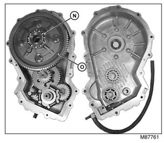
12.Install ring gear and differential assembly (O).13.Seat axle bearing (N) on ring gear and differential
