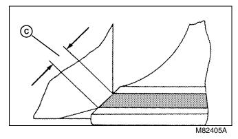
4. Measure valve seat width. Inspect valve seat for wear or damage. If valve seat width is not within 0.50 - 1.10 mm (0.020 - 0.043 in.) (C), recondition valve seats.
