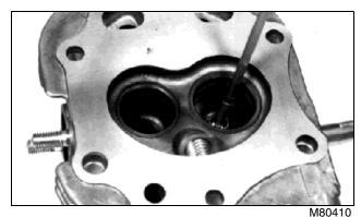
2. Measure inside diameter of valve guide bushings. If ID is greater than 7.065 mm (0.2781 in.), replace bushings.
