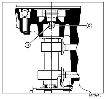
4. Apply clean engine oil to camshaft lobes, journals, and tappet guides before installation.
