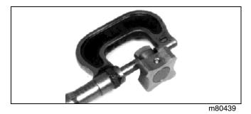
Measure rotor shaft diameter. If shaft OD is less than 12.63 mm (0.497 in.), replace both shaft and outer rotor.
