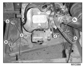
7. Remove two nuts (D & D1) attaching each engine mount. Retain hardware. Replace engine mounts as necessary.
