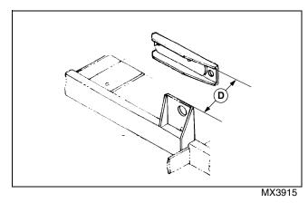
6. Determine the number of shim washers required when assembling the snubber isolators to maintain the center distance by accurately measuring gap (D) between frame and engine bracket and using the following chart. Gap can be best measured using an inside calipers.
