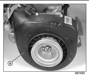
6. Remove six cap screws attaching blower housing section (G) and remove section.
