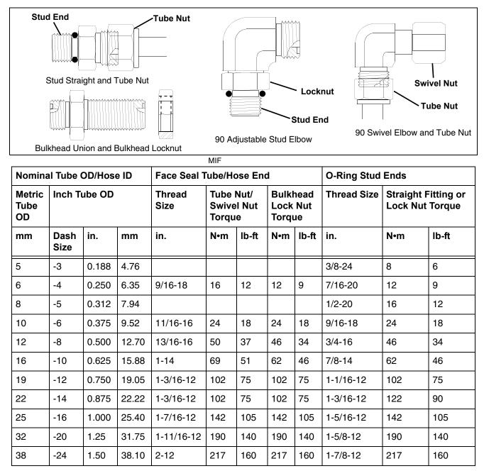
NOTE: Torque tolerance is +15%, -20%
