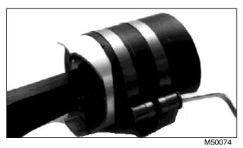
11.Install piston and connecting rod assembly in cylinder bore with engraved match mark/arrow on piston head facing flywheel side of engine.
