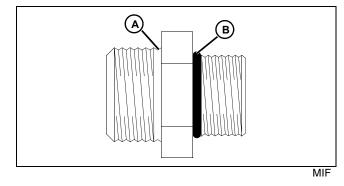
2. Put hydraulic oil or petroleum jelly on the O-ring (B). Place electrical tape over the threads to protect O-ring from nicks. Slide O-ring over the tape and into the groove (A) of fitting. Remove tape.
