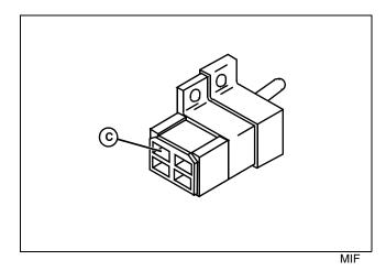
(3) Is battery voltage present at S4 park brake switch - 410 Yel wire (C)?
