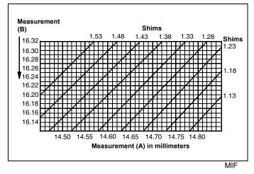
4. Locate measurements on appropriate table. Follow lines to where recorded measurements intersect. Choose the next smaller shim from the table.
