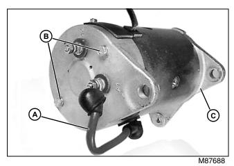
2. Disconnect jumper wire (A) from end of starting motor/ generator.
