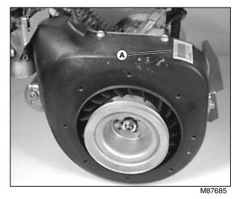
Engine serial number (A) can be located on the blower housing.
