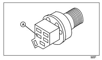
(2) Is battery voltage present at S2 key switch - 200 Red wire (A)?
