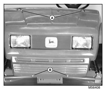
2. Loosen top cap screws (A) and (B).
