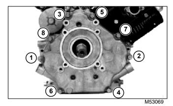
3. Install short end of mounting stud into block.
