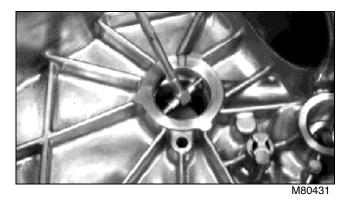
5. Measure crankshaft main bearing diameter in crankcase. Replace crankcase if diameter is greater than 30.08 mm (1.184 in.).
