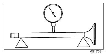
2. Inspect valve stem for bend using v-blocks and dial indicator. Turn valve slowly and read variation on indicator. If variation is greater than 0.03 mm (0.0012 in.) replace valve.
