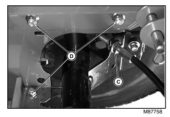
7. Loosen jam nut (C) and disconnect brake cable housing from axle bracket.
