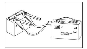
6. Connect variable rate charger to battery.
