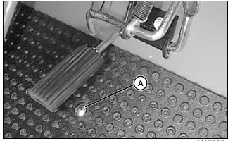
6. Adjust position of pedal stop (A) to achieve desired reading.
