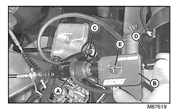
5. Remove high tension lead (A) from spark plug and connect to spark tester (B).
