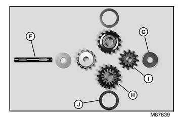
7. Inspect bevel pinion gears (H), cross shaft bevel pinion gears (I), shaft (C), and washers (G) for wear, corrosion, discoloration, and damaged teeth (12 and 15 teeth). Replace differential assembly as necessary.
