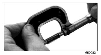
Measure relief valve spring free length. Replace spring if measurement is less than 19 mm (0.748 in.).
