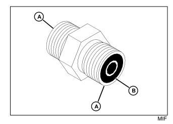
1. Inspect the fitting sealing surfaces (A). They must be free of dirt or defects.
