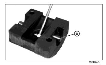
4. Measure support shaft bearing diameter in balancer weight. If bearing ID is more than 26.10 mm (1.027 in.), replace balancer weight.
