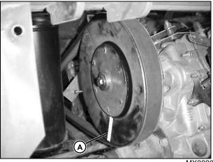
2. Install reflective tape (A) on the secondary clutch. It may be necessary to apply black paint to the outside of clutch for reflective tape to allow photo tachometer to read the reflective tape.
