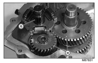
7. Partially install input shaft (G) and then install gears (H). Ensure input shaft is fully seated and gears mesh.
