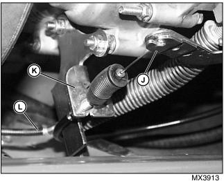
17.Slide governor cable into cable support bracket (K).
