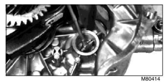
3. Measure camshaft bearing diameter in cylinder block. If bearing ID is greater than 23.06 mm (0.908 in.), replace block.
