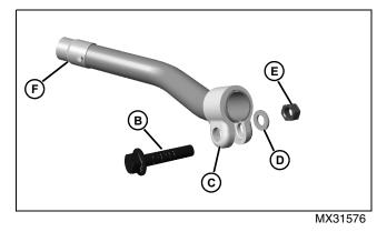
4. Install bolt (B) through the welded clamp (C), washer (D) and secure with lock nut (E).
