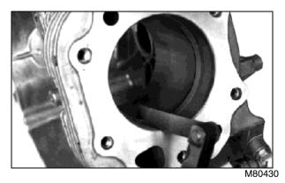
10.Measure piston ring end gap. Push ring into cylinder bore, using a piston, until ring is approximately 25.4 mm (1 in.) down from top of cylinder bore.
