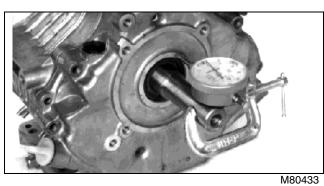
4. Push crankshaft in as far as possible. If end play is not within 0.09 - 0.22 mm (0.004 - 0.009 in.), adjust end play.
