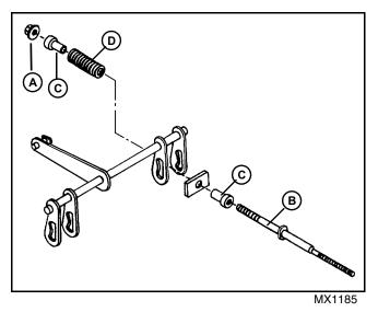
4. Tighten nut (A) onto linkage (B) completely until the ends of sleeves (C) make contact inside spring (D). This sets a predetermined preload on the spring. Repeat for second cable.
