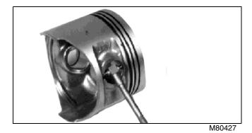
12.Measure piston pin bore diameter. Replace piston if diameter is greater than 19.03 mm (0. 749 in.).
