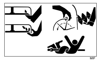
Keep hands and feet away while machine is running. Shut off power to service, lubricate or remove mower blades, augers or PTO shafts.
