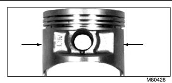
13.Measure piston diameter perpendicular to piston pin bore.
