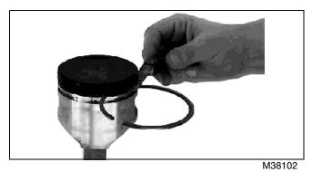
9. Measure piston ring groove clearance. Measure several places around piston.
