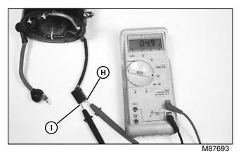
Check for continuity through generator coils at DF connector (H and I). There should be approximately 5.0 ohms of resistance.
