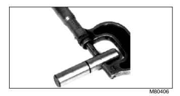
1. Measure outside diameter of rocker shaft. Replace shaft if OD is less than specification.
