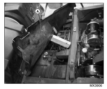
2. Remove two rear cap screws securing seat base cover (A) to frame. Prop seat base cover up with a block of wood to provide access to snubber isolators.
