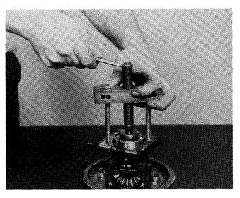
4. Using a bearing puller, remove differential bearings from each side of case.
