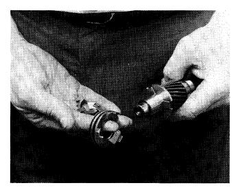
(Gas Axle Only) After inner bearing removal, governor weights, inner and outer thrust washers, and thrust bearing will be free for removal.
