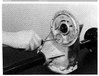
Punch or drill approximately 1/8" diameter near the center of each intermediate bore plug. Insert a suitably sized sheet metal screw until the metal bore plug is forced out of the bearing bore.
