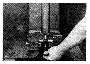
(Gas Axle Only) If necessary, remove governor backing plate from input shaft with arbor press.
