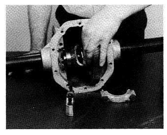
3. Remove differential case assembly from housing.
