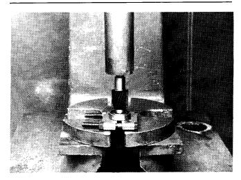
Press inner and outer bearings on input shaft to bearing shoulders.
