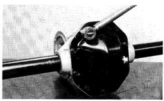
Place a small bead of RTV (non-acidic) silicone sealant to bottom flange of axle housing. Sealant should be applied inside of cover plate mounting holes. Install the ten (10) cover plate screws and torque to 18-28 Ft. Lbs.
