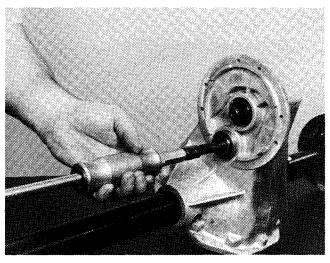
4. Using an I.D. bearing puller attached to a slide hammer, remove intermediate bearing from flange side of housing.
