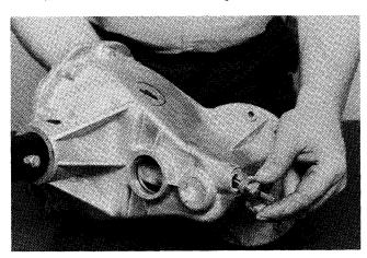
8. (Gas Axle Only) After steps 2, 3, 4, 5, and 6, install bushing assembly and governor actuator. Actuator must be inserted thru inside of housing and bushing from outside. Actuator tangs must be against rear of outer thrust washer. Torque bushing to 35-45 Ft. Lbs. Refer to Diagram #2 for proper location of actuator tangs.
