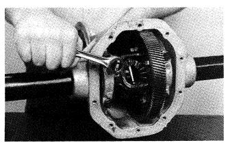
Remove four (4) bearing cap screws and remove bearing caps.
