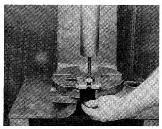
3. Using an arbor press and bearing support, remove bearings from both ends of input shaft.
