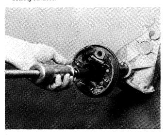
Using an oil seal puller, attached to a slide hammer, remove oil seal. Use caution as not to damage the seal seating surface.
