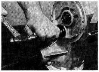
3. Using a brass drift pin, drive the intermediate shaft from the flange side of housing. Shaft should travel far enough to allow engagement of I.D. bearing puller.
