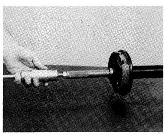
2. Using a slide hammer attached to the threaded end of the axle shaft, remove axle and bearing assembly.
