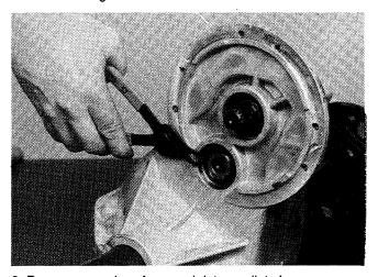
2. Remove snap rings from each intermediate bore.
