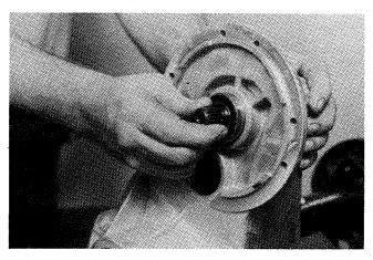
Pull input shaft assembly from housing. The input shaft assembly should slide out of the housing easily. If resistance is encountered, a slide hammer may be required. Use caution as not to damage gear.
