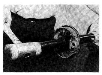
With properly sized seal driver, install shaft seals.
