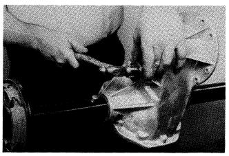
5. Install new intermediate bore plug to both sides of housing. Use Loctite Safety Solvent #75559 to clean bores, then apply Loctite RC 609 to housing bores. Bore plugs can then be installed by using a properly sized driver and a hammer.
