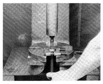
3. Remove the bearing from the axle shaft, by supporting the inner race of the bearing on an arbor press, and apply pressure to the threaded end of the axle shaft.
