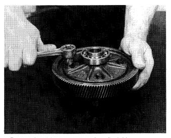
Remove four (4) bolts and nuts from final drive gear.
