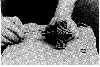
6. Remove "O" rings at each end of intermediate shaft on bearing shoulders.
