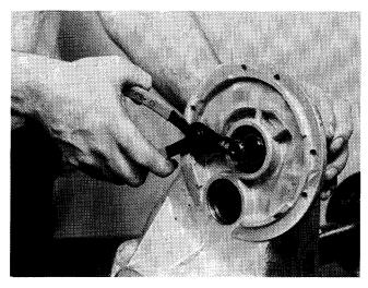
1. Remove snap ring from input shaft bore.
