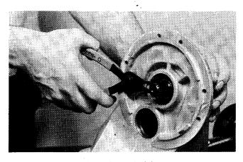
3. Install outer snap ring at input shaft bore.
