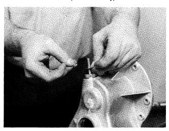
4. (Gas Axle Only) Remove "E" clip and washer from top of governor actuator bushing.
