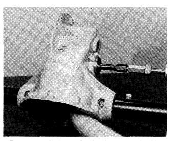
5. Repeat step 3 for intermediate bearing on opposite side. CAUTION: Shaft and gear assembly must be supported by hand as not to damage gear teeth. NOTE: Small end of intermediate shaft and gear assembly must be tilted toward opening in bottom of housing for removal. Use caution as not to damage gear teeth.
