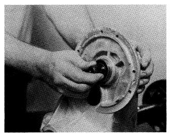
Reinstall input shaft. Bearings and shaft should slide easily into housing. If resistance is encountered, a plastic or leather mallet could be used to tap the shaft into its correct position, using caution not to damage gear teeth.
