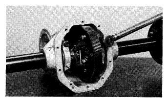
Position housing with opening up and insert differential case, final drive gear, and bearing assembly into housing. Install differential bearing caps.
