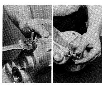
(Gas Axle Only) Remove governor bushing. Governor actuator can then be removed from inside of housing.
