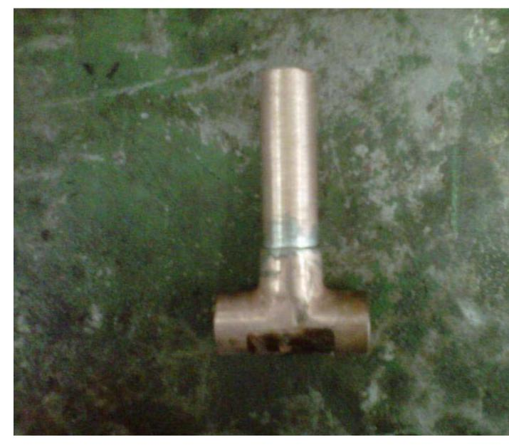
The tool is just a piece of 1/2 copper pipe with a T soldered on it .
